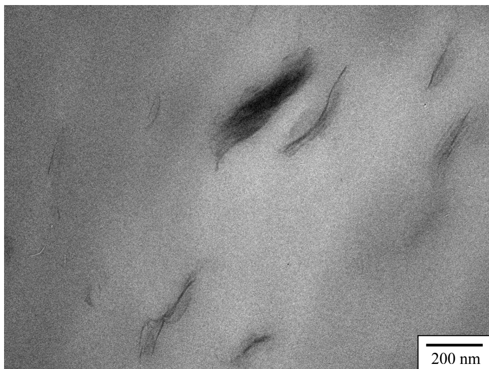
Figure 7.10: TEM micrographs of linear PP/diamino monomethoxy silated I.30P (PPNC-S3) nanocomposites showing the effect of extrusion on nanoclays dispersion (top: before extrusion, bottom: after extrusion).
