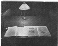
Fig. 1. Illustrating the effect of specular reflection from a polished surface. The book at the right has matt paper, the one at the left glossy. The camera is placed at the position of the eye. It is impossible to see the printing on the glossy paper.
