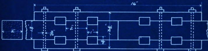
KEYED FISH PLATE SCALE \frac{3}{8}'' = 1'' DESIGNED FOR 2000 # TENSION
