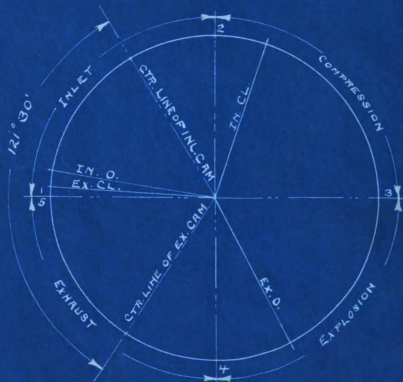
DIAGRAM OF CAM SETTING FOR FOUR-STROKE CYCLE.
