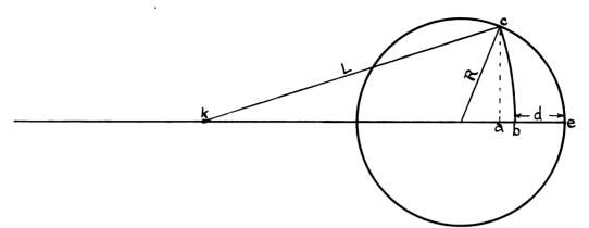
In the above figure, representing kinematically the working parts of an engine, as - ab = d, as = R vers  $\alpha$ , ab = L-ka, ka =  $\sqrt{L^2 - ca^2}$ ,  $ca^2 = R^2 sin^2 \alpha$ , whence d = R vers  $\alpha$  -L +  $\sqrt{L^2 - R^2 sin^2 \alpha}$ d = distance of piston from end of stroke when corresponding crank angle is  $\alpha^{\circ}$ .
