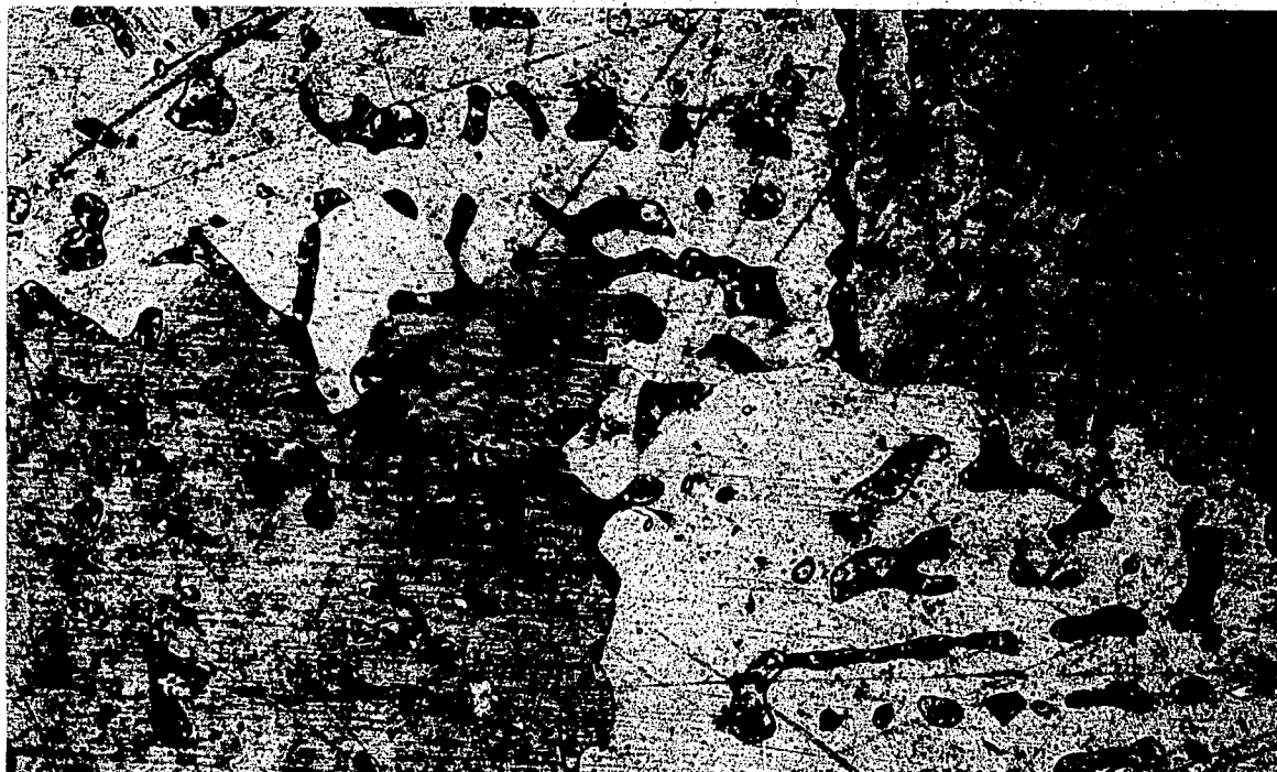
FIGURE 45. Microstructure of a cast and solution heat-treated alloy containing 2.25% Be- 0.04% Fe- 97.63% Cu. Etch: Ferric Chloride Magnification: 100X
