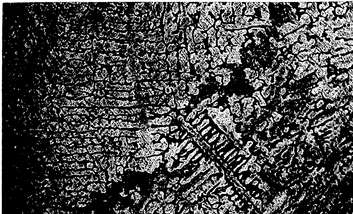
FIGURE 37. Microstructure of a cast alloy containing 2.25% Be-0.04% Fe- 97.63% Cu. Etch: Ferric Chloride Magnification: 100X
