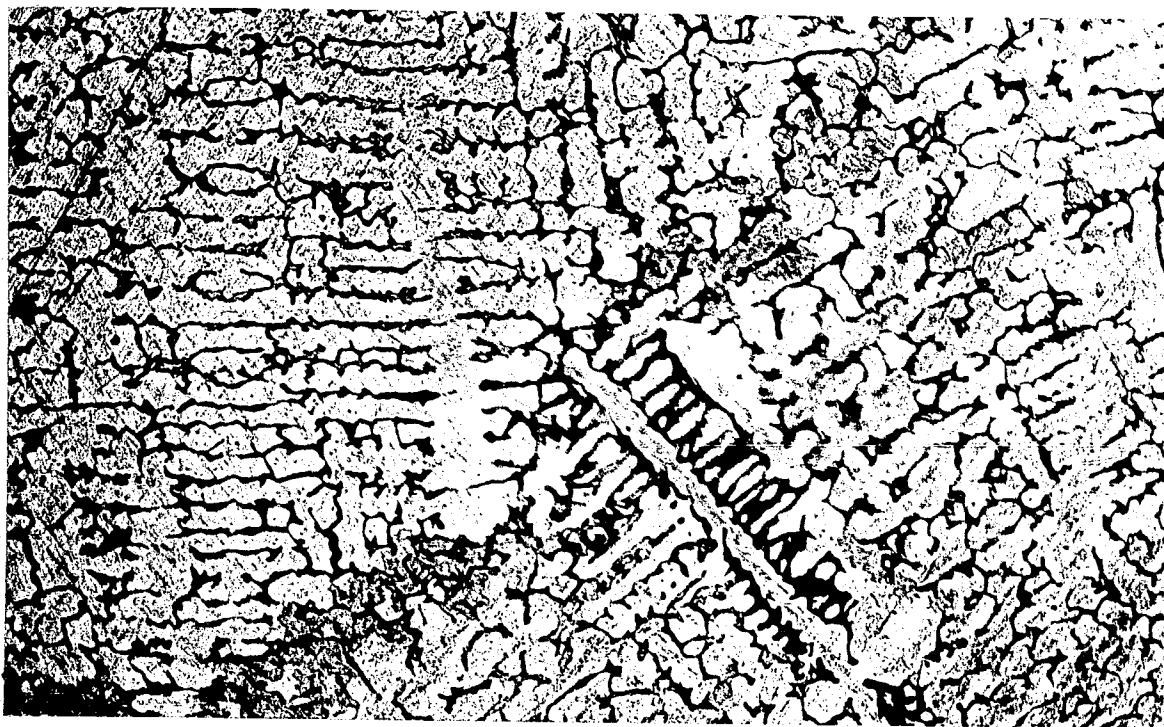
FIGURE 7. Microstructure of a cast alloy containing 2.25% Be-0.03% Al- 97.63% Cu. Etch: Ferric Chloride Magnification: 100X
