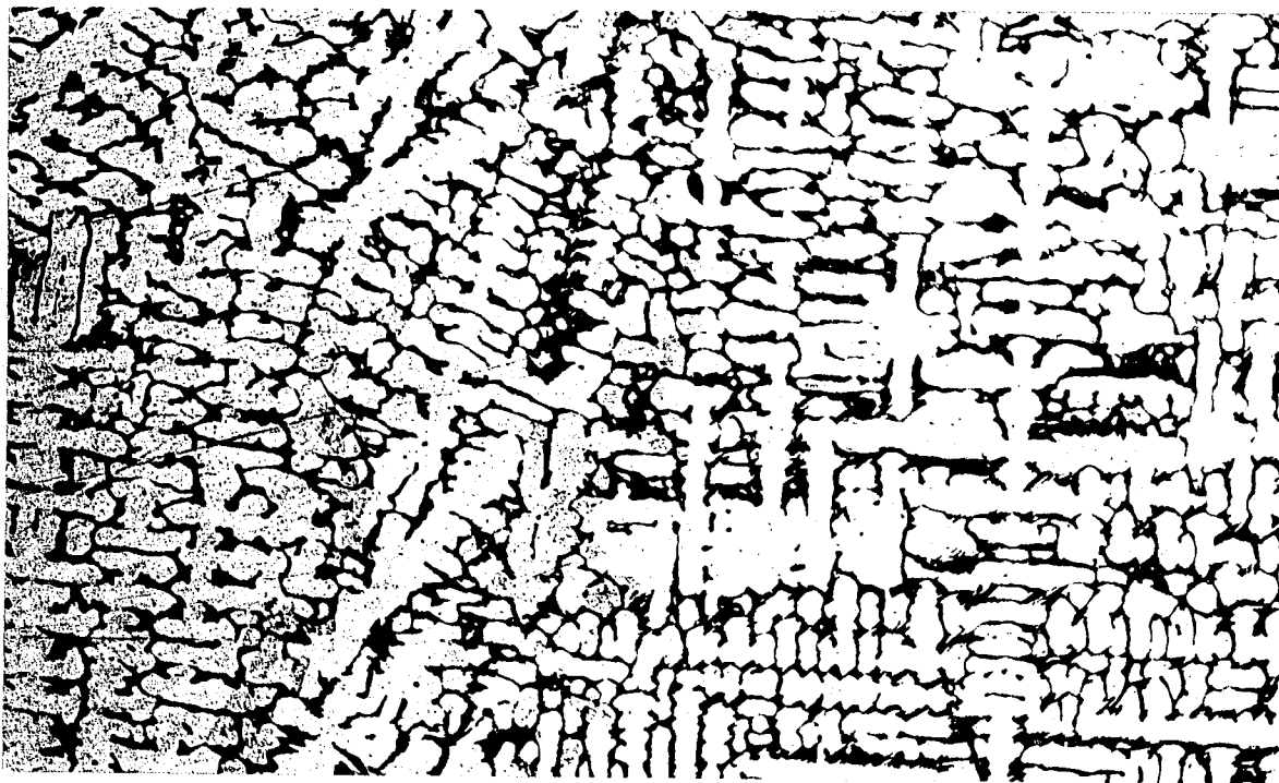
FIGURE 11. Microstructure of a cast alloy containing 2.18% Be-1.07% Al- 96.69% Cu. Etch: Ferric Chloride Magnification: 100X
