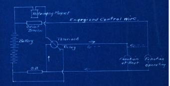
If we had a cross between the buss bars or wires on the interlocking machine (shown on the drawing by dotted lines) the current would flow in the direction as shown by the dotted arrows which is opposite to the normal flow and would magnetize the coil of the polarized relay in the opposite direction and immediately open the circuit broaker.
