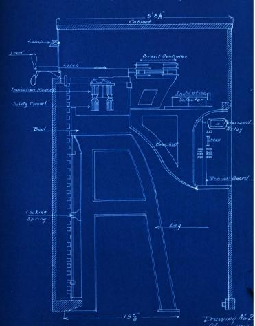
The indication selectors mounted on the rachine, as shown on the drawing, consists of two electro-magnets and a contacting armature which throws in one direction when the lever is reversed and in the other when the lever is put normal.
