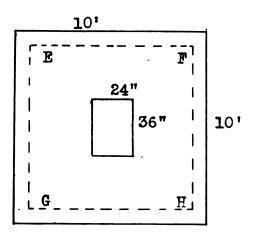
Since d = 36"the total shear on EFGH  $= \frac{100 - 8 \times 9}{100} \times 507,000 =$  142,000 #  $V = \frac{V}{b j d} = \frac{142,000}{388 \times .875 \times 32} =$  13.4 # so no are needed.
