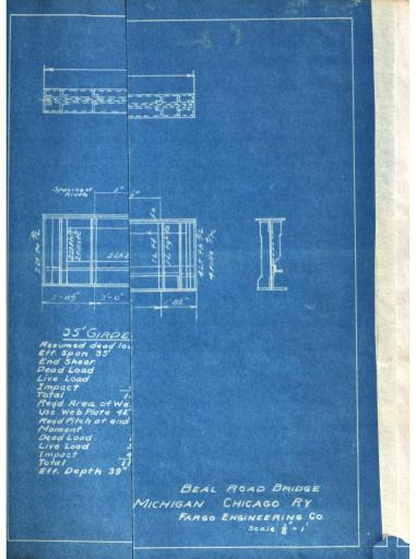
Complete Design of a 35' Through Plate
