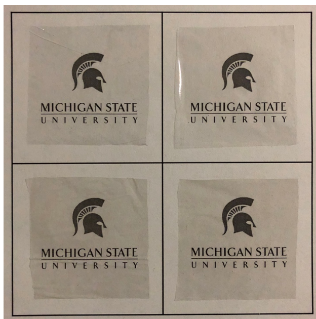
Figure 4.22 Visual clarity of PLA and PLA/CNC nanocomposite films.
