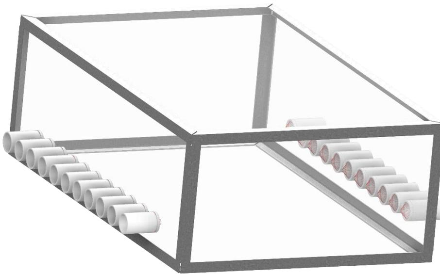
Figure 4.3: An AutoCAD rendering of the initial trap design. SoftValves are placed low enough on the frame for crayfish to have access. The galvanized steel mesh is shown as a clear surface to better view the SoftValves.
