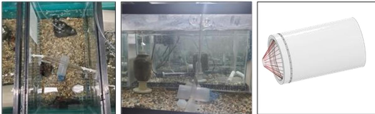
Figure 4.2: The top view shows two RSC that moved through the SoftValve to the bristle side of the aquarium (left). The profile view (middle) show the directionality of the Softvalve. A 3D rendering was created using Autodesk Inventor™ (right).
