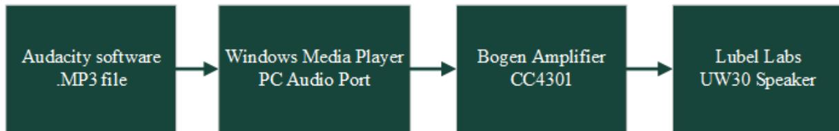
Figure 2.2: Flowchart of the process used to play sounds in habitats.
