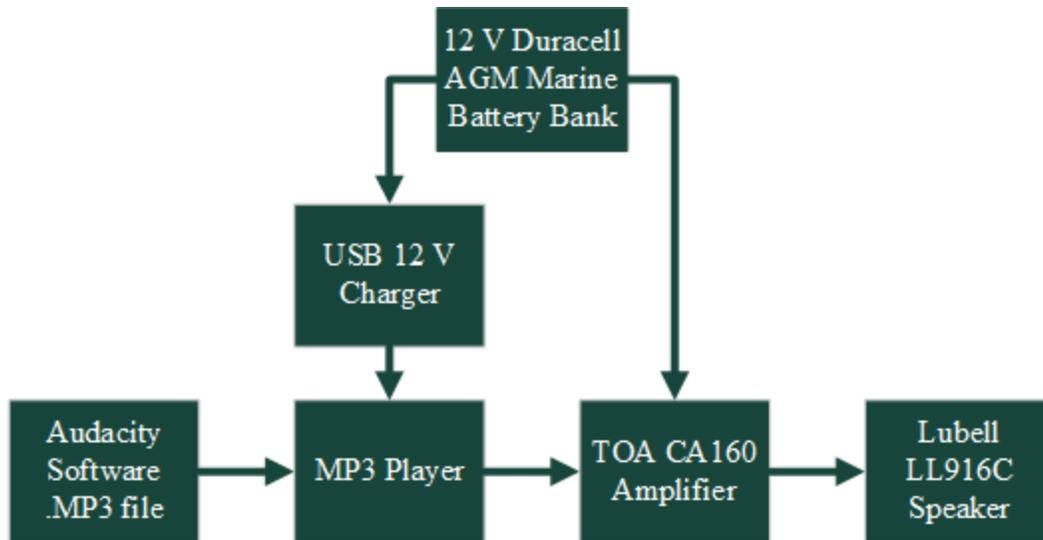
Figure 3.3: Process flow for sound generation using batteries as a remote power source.
