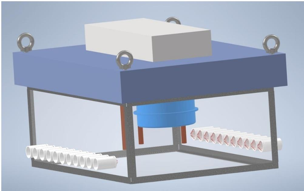
Figure 4.4: A floating mat is attached to top of the trap. Modular systems such as battery bank, heating elements, speakers and anchors for drone retrieval are attached.
