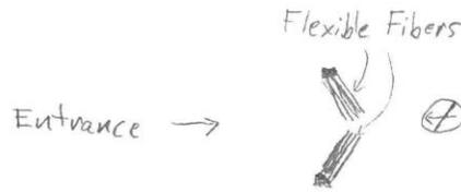
Concept: Fibers bend to allow crayfish in, but axial forces are resisted upon exiting
