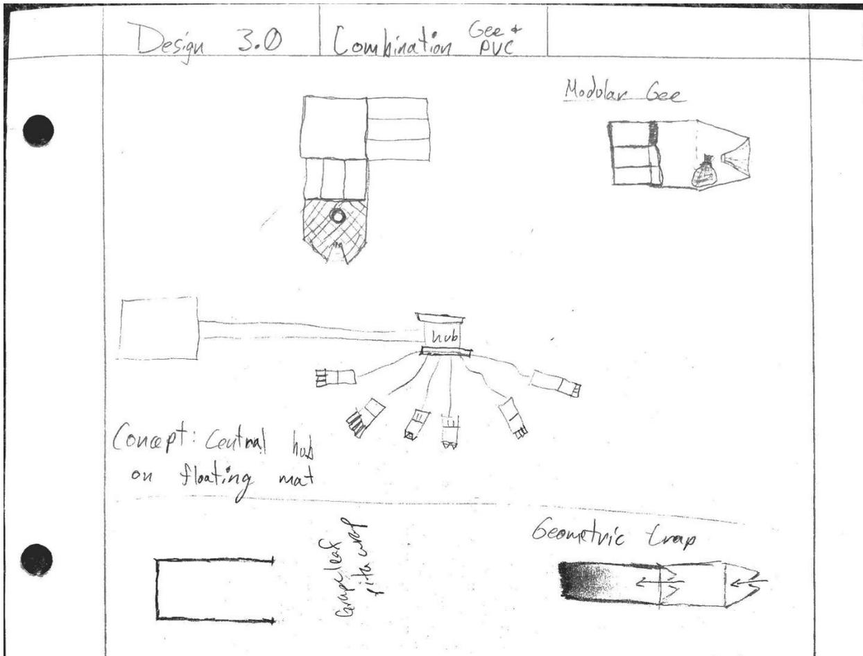
Figure C.3: The third design uses a combination of semi-cylindrical trap and refuge trap to direct crayfish toward a central floating cage.
