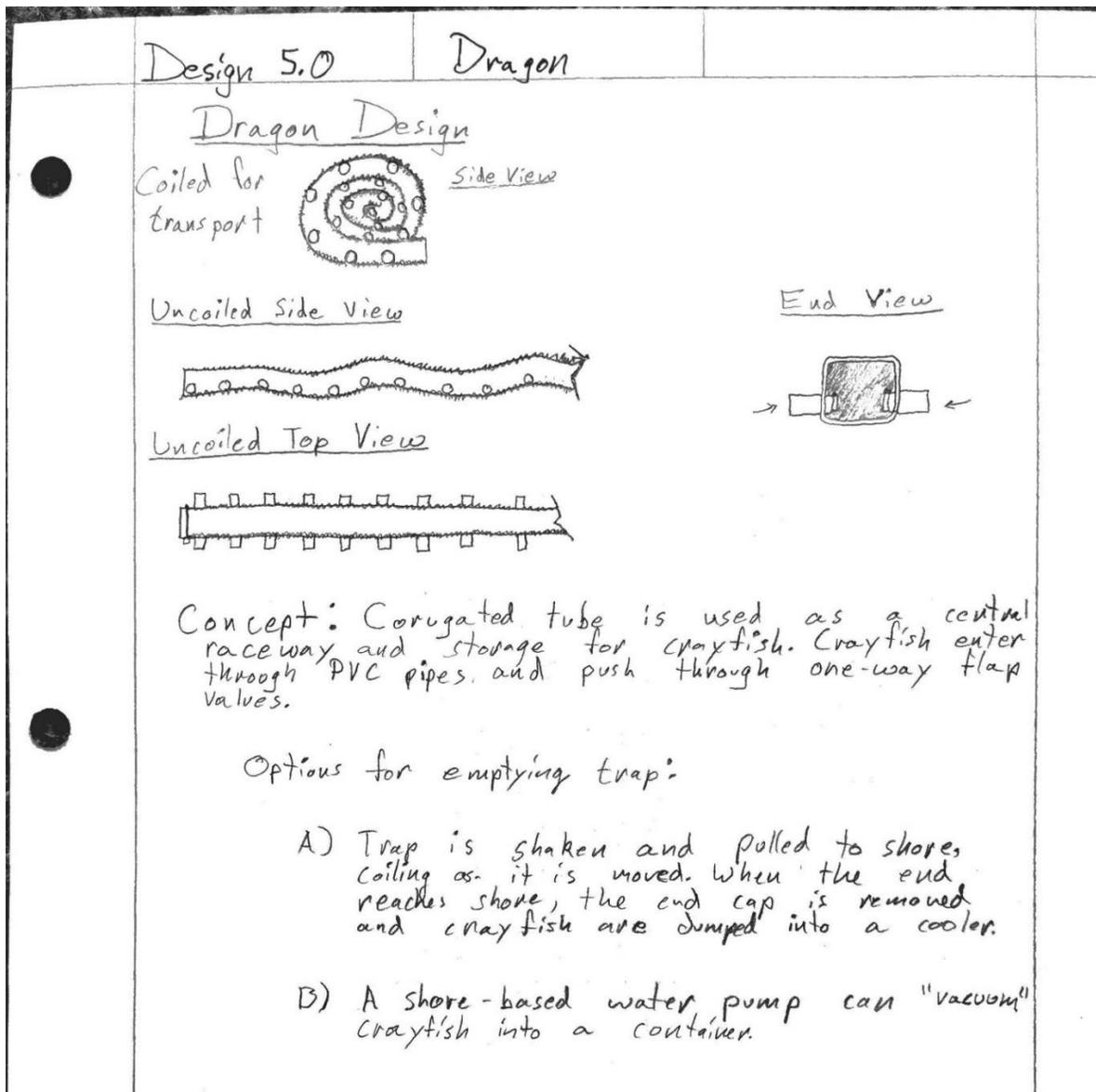
Figure C.5: The Dragon design is made of a corrugated plastic tube that coils up for storage and is uncoiled during deployment. Refuge tubes with flapper valves allow crayfish to enter into the corrugated tube.
