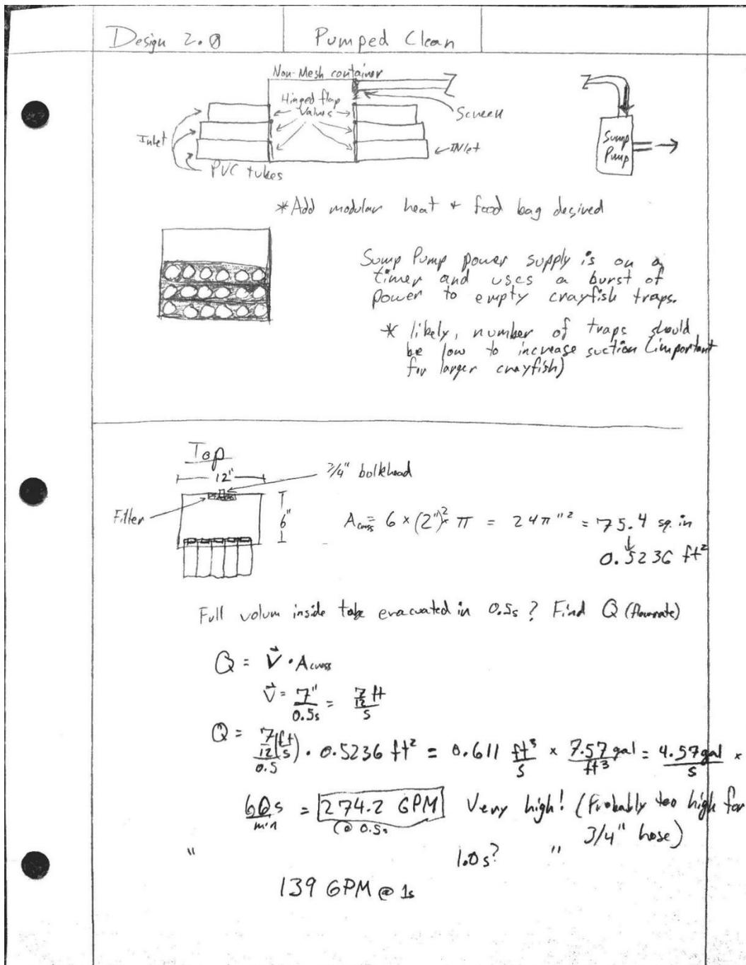
Figure C.2: Crayfish enter the refuge style traps before a pump intermittently empties traps into a cage through a flapper valve.
