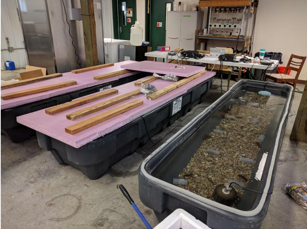
Figure 2.1: The cattle bunk feeders provided a long and narrow habitat shape for conducting the lab-scale research. This picture was taken during cleaning of the sponge filter in zone 2, which explains its absence. A layer of door sealing insulation was used to create a seal around the uneven top of the bunk feeders, to prevent escape.
