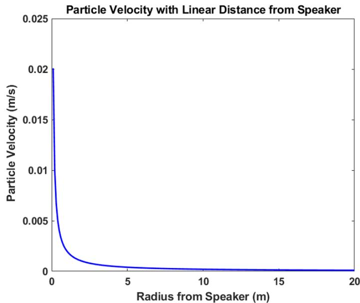
Figure 3.5: The particle velocity is asymptotic about zero as radius from the speaker increases.
