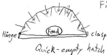
Fibers imbedded in silicone dome with holes to allow crayfish in, but not out.
