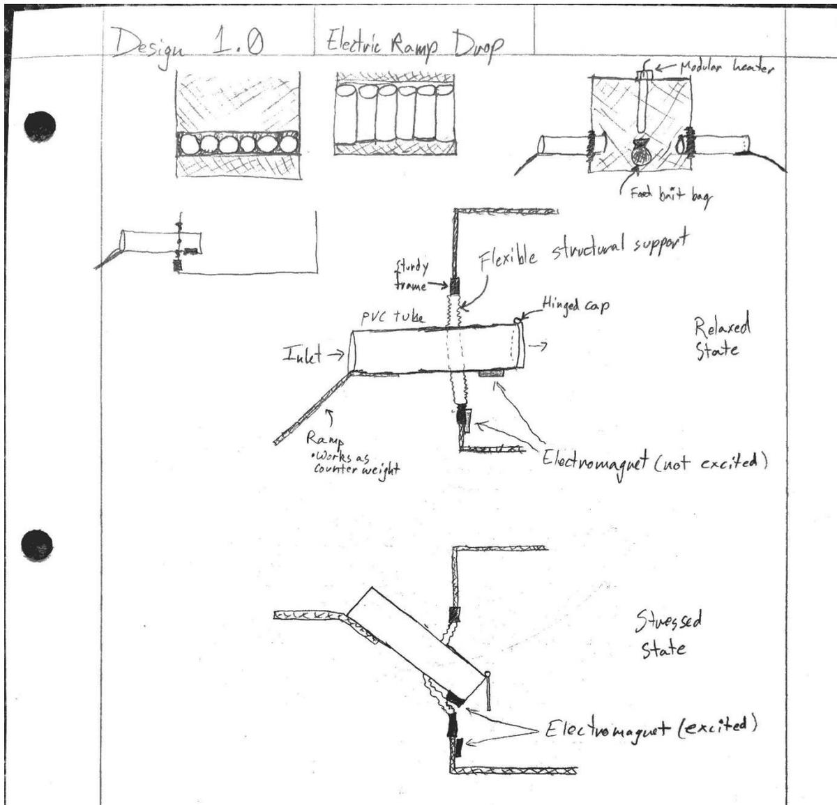
Figure C.1: PVC pipes are tipped upwards using electromagnets to empty crayfish into a cage.
