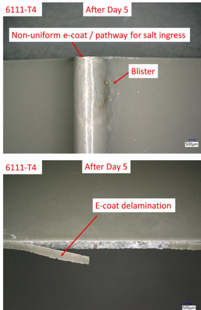
Figure 6.6 Digital micrographs (20x) of a 6111-T4 alloy conversion coated with Bonderite M-ZN 958 and e-coated after a 5-day exposure to a G85 test. Top micrograph: arrows indicate a region where electrolyte creep underneath the e-coat layer occurred resulting in the formation of a blister. Bottom micrograph: an example of e-coat layer delamination along the edge of a hem flange.
