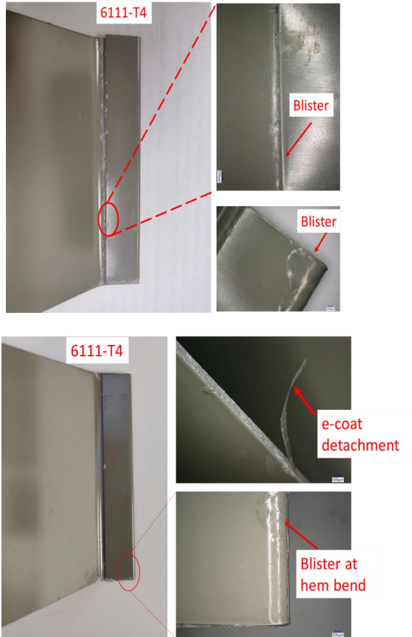
Figure 6.9 Photographs (left) and digital micrographs (right) (20x) of AA6111-T4 specimens with (Top) Bonderite M-NT 1820 and (Bottom) Bonderite M-ZN 958 conversion coatings and an e-coat after a 30- day G85 test. Small blisters are seen at the hem edge (top right) and hem bend (bottom right).
