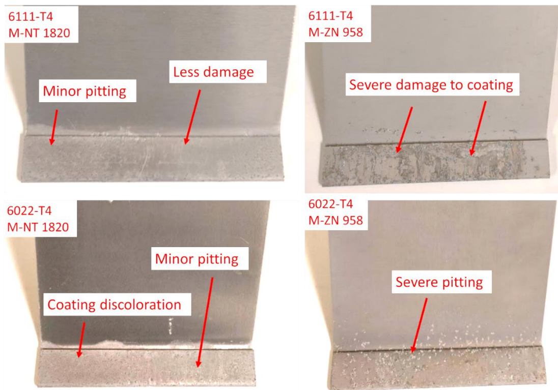
Figure 6.12 Photographs of conversion coated 6022-T4 and 6111-T4 hem flange specimens after 5-Day G85 test. Of the two alloys, 6111-T4 showed more corrosion damage. Bonderite M-NT 1820 conversion coated panels appear less damaged than panels conversion coated with Bonderite M-ZN 958.
