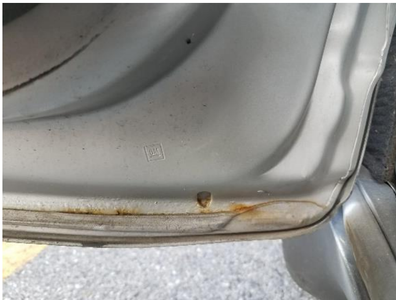
Figure 6.1. Photograph of an actual hem joint on the inside of an automobile door panel where corrosion has developed along the joint edge during service.
