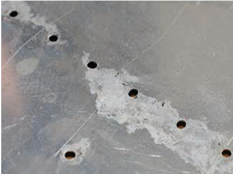
Figure 1.3 Filiform corrosion attack on an aircraft wing. Areas around fastener holes are most affected by corrosion. Imaged obtained from online source: Aviation safety experts ( http://www.dviaaviation.com/aircraft-corrosion.html ).
