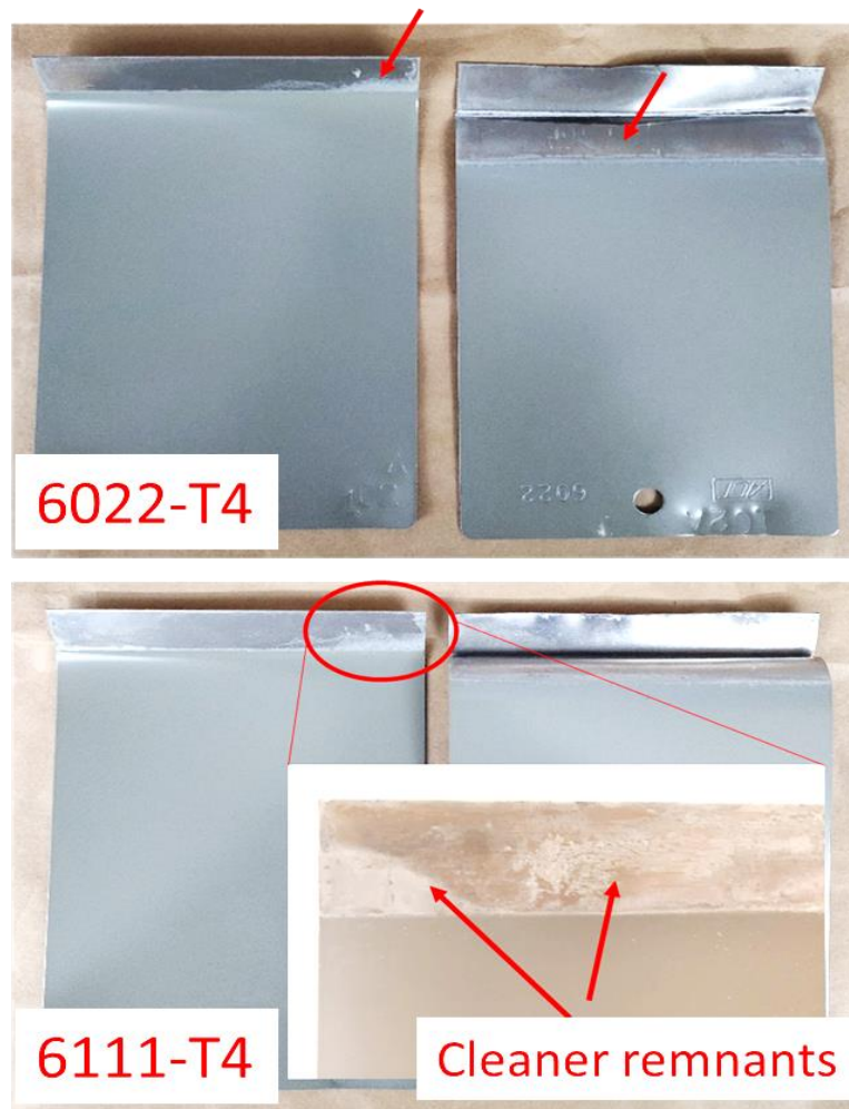
Figure 6.4 Photographs of Bonderite M-NT 1820 conversion coated, and e-coated hem flanges separated before G85 testing. Inspection of the photographs reveal no evidence of e-coat under the hem. Arrows and the inset figure indicate cleaner residue.
