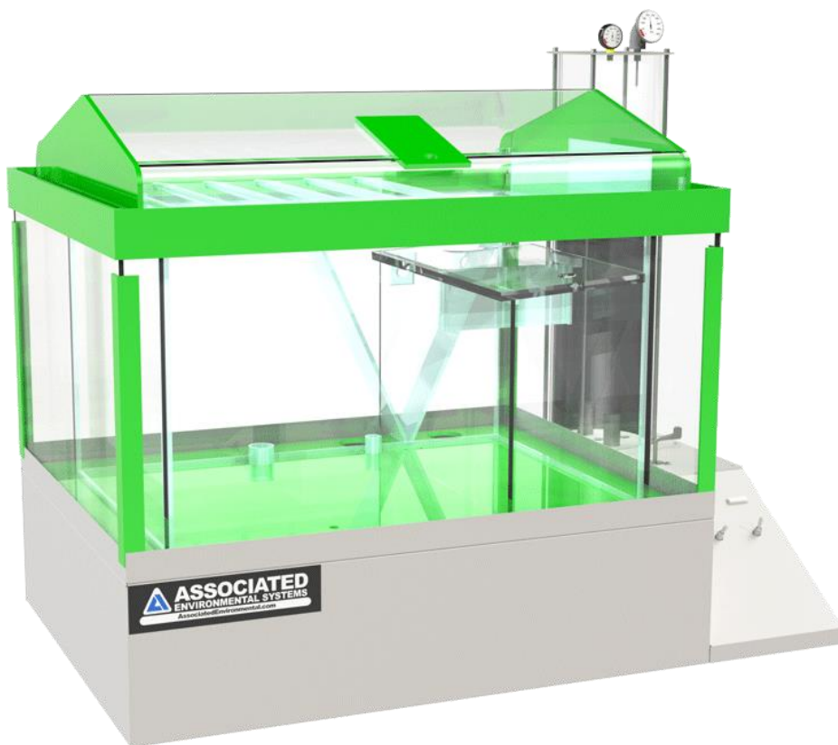
Figure 2.5 Photograph of the salt spray chamber apparatus used for 14-day ASTM B117 test.
