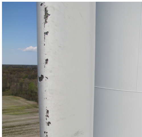
Figure 1.1: The onset of roughness on the leading edge of a wind turbine blade due to surface erosion [1].
