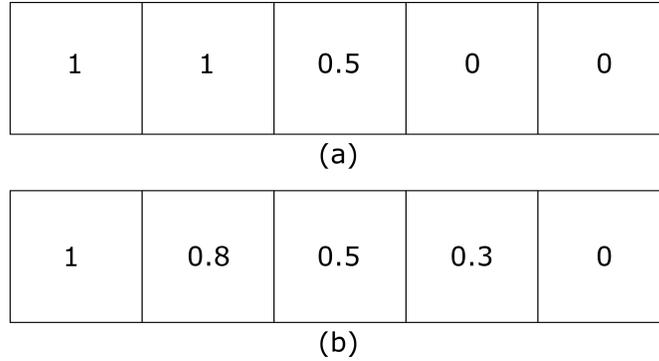
Figure 4.4: Volume fraction field: (a) ideal sharp interface (b) smeared interface
