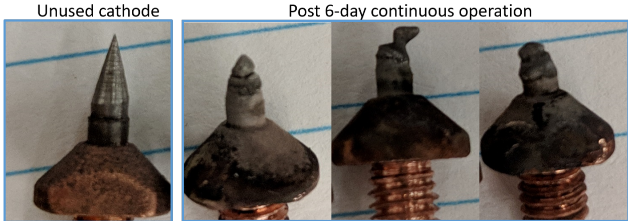
Figure 4.44: The three thoriaated tungsten cathodes after a 6-day continuous operation run in helium at GCS pressure 300 torr and 180 A arc current. Also shown for comparison is an unused cathode.
