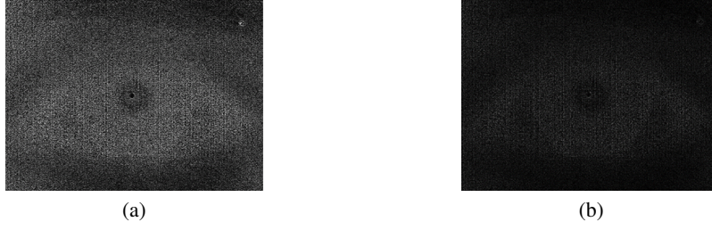
Figure 2.3: Noise residual from an image captured using the Aoptix Insight sensor. (a) Before enhancement. (b) After enhancement. The application of enhancement model subdues the scene content in the image significantly.
