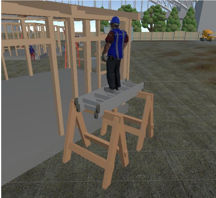
Figure 3.20: Hazard 1 – Worker using step ladder as scaffolding
