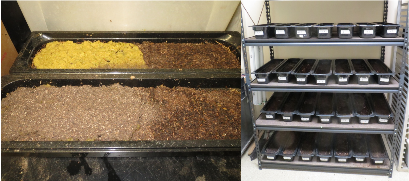
Figure 3.1. A) Laboratory set-up for vermicomposting feeding trial with the seven treatments, one replication per shelf and a total of four replications and B) Close-up of feeding of pineapple on one half of worm bin (back) and covered with ground leaves before being wet by misting (front).
