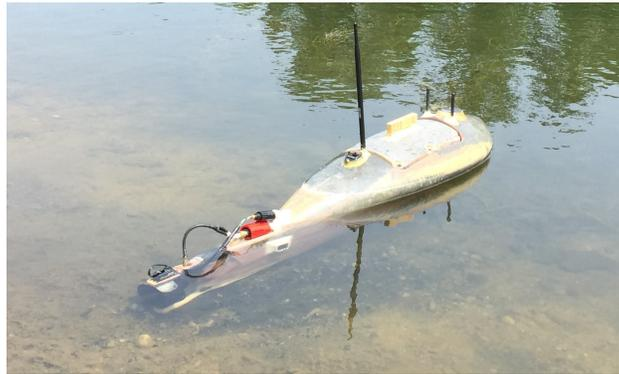
Figure 2.9: An USV prototype developed by the Smart Microsystems Lab based on an alternative design concept.
