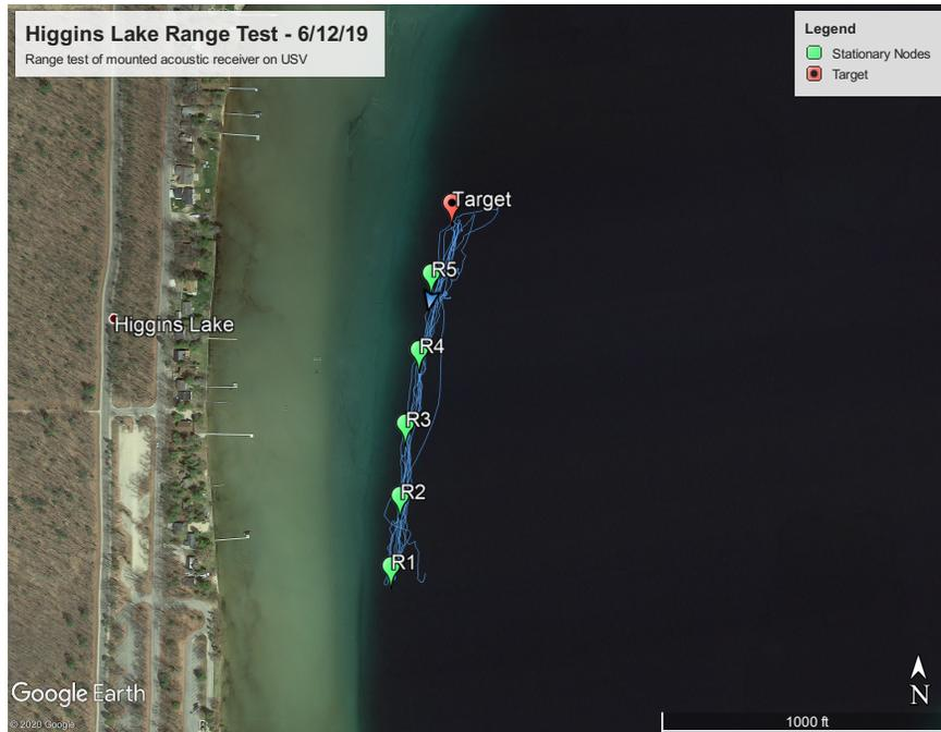
Figure 2.5: Map of the acoustic receiver range test for the mounted and stationary acoustic receivers. The blue arrow and line show the USV's path, the red pin marks the target, and the green pins mark the stationary receivers.
