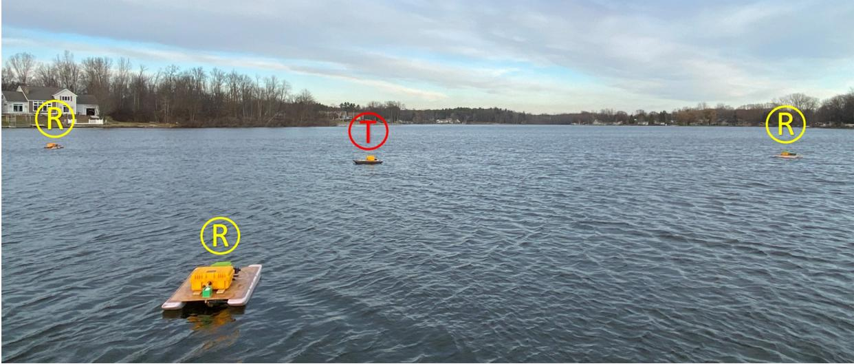
Figure 2.8: Deployed USV network. (T) represents the USV carrying the acoustic tag, and (R) represents the receiving nodes.
