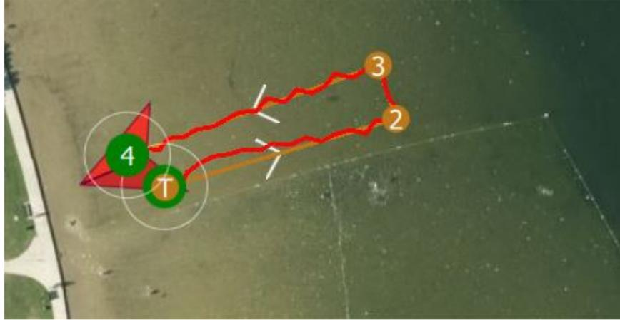
Figure 4.1: USV waypoint tracking after controller tuning. Slight steady-state oscillations along the trajectory can be observed.
