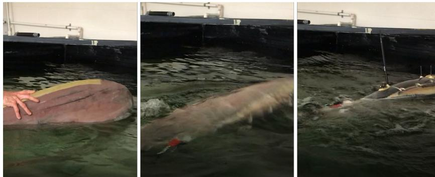
Figure 2.10: Demonstration of the self-righting capabilities of the USV based on the alternative design.
