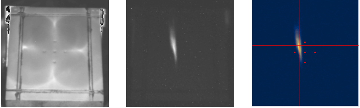
Figure 4.16: Viewer image analysis process. Left: CCD image of the image with light on to find scale from the 5 mm dot markings. Center: Raw TIFF image of the beam from CCD. Right: Background subtracted beam image with the red lines marking the beam spot center, and red dots indicating the center with 5 mm distance between each dot. In this image, each pixel corresponds to approximately 0.15 mm.
