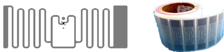
Figure 1.2: Low cost example UHF RFID tags for supply chain applications.
