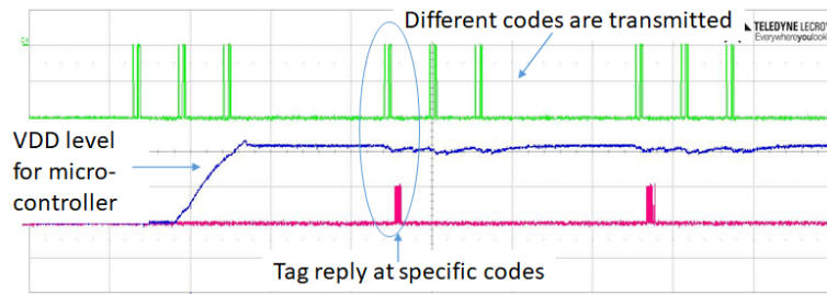
Figure 6.16: Activation of a dual mode tag due to specific code sent from the reader.
