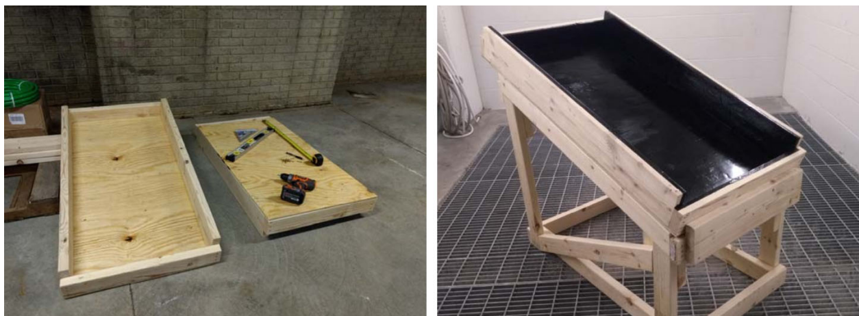
Figure 10: Construction of Wooden Rainfall Racks and Soil Form, Photos by Patrick Bollinger
