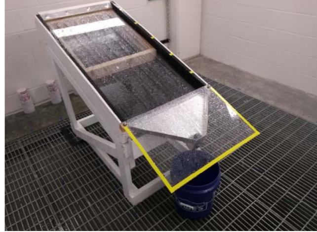
Figure 11: Concept Design Sketch and Completed (Built) Version of Rainfall Test Apparatus, Photo and sketch by Patrick Bollinger
