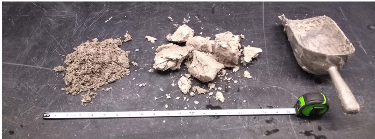
Figure 4: Consistency of Typical Settled CGR Solids (After Decanting), Photo by Patrick Bollinger
