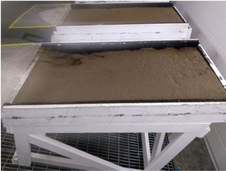
Figure 61: Soil Forms Showing Soil Erosion After Rainfall Simulation, Photos by Patrick Bollinger
