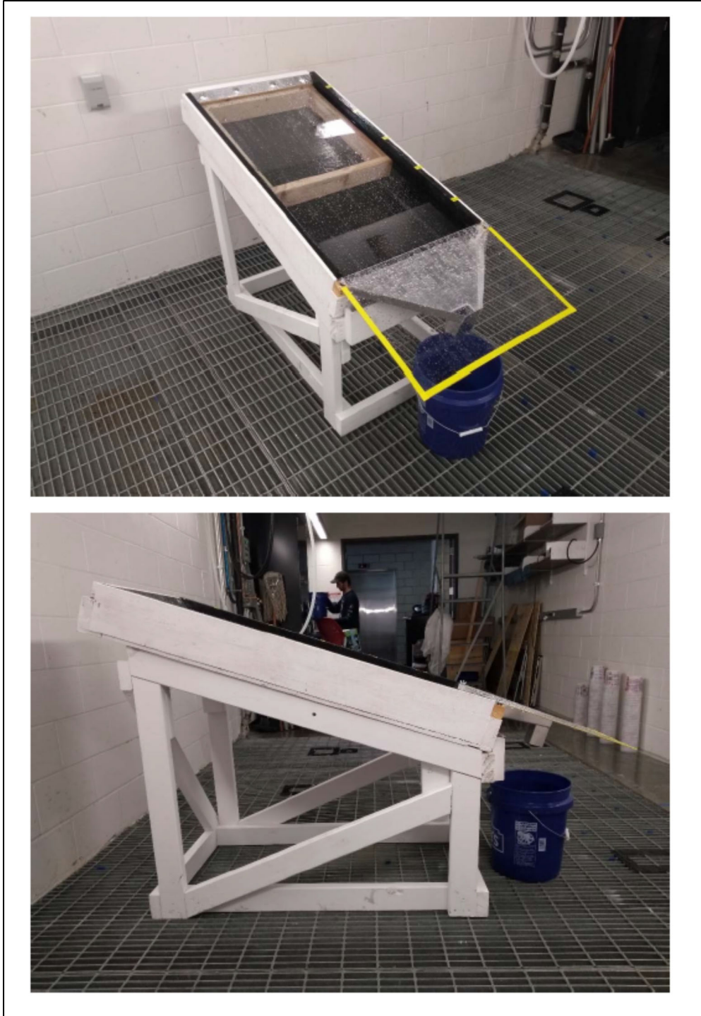
Figure 59: Assembled Rainfall Wooden Rack, Soil, Form, and Metal Funnel, Photos by Patrick Bollinger
