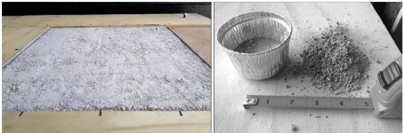
Figure 41: Soil Loss Due to Wind Erosion from Compacted Soil Form, Photos by Patrick Bollinger
