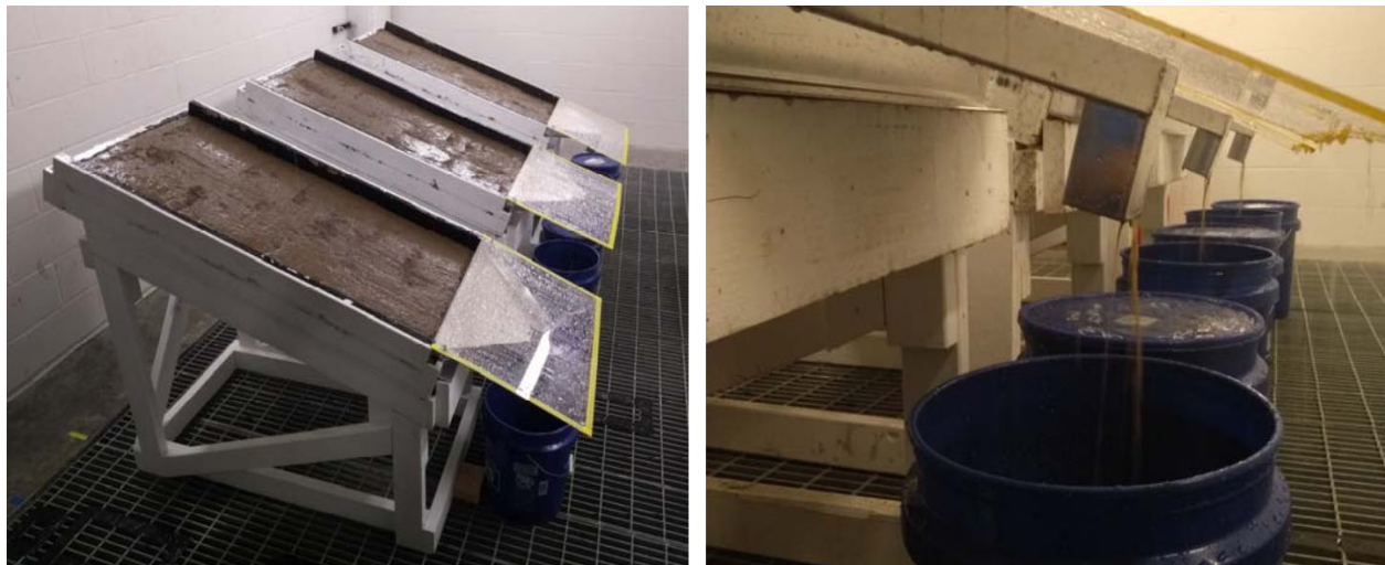
Figure 22: Typical Rainfall Simulation and Captured Sediment-Laden Water Runoff, Photos by Patrick Bollinger
