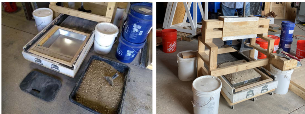
Figure 37: Steps During Compaction of Soil Forms using UTA, Photos by Patrick Bollinger
