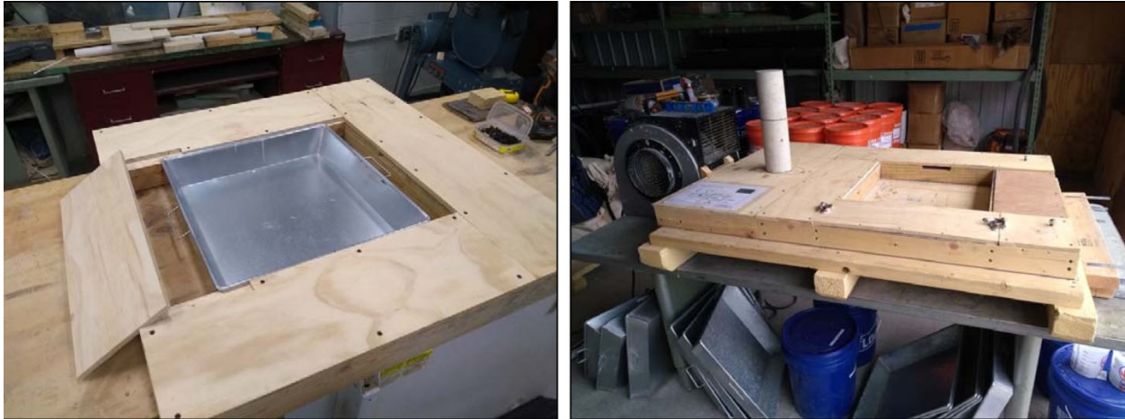
Figure 35: Wind Erosion Test Apparatus (WETA) During Fabrication and Final Construction, Photos by Patrick Bollinger
