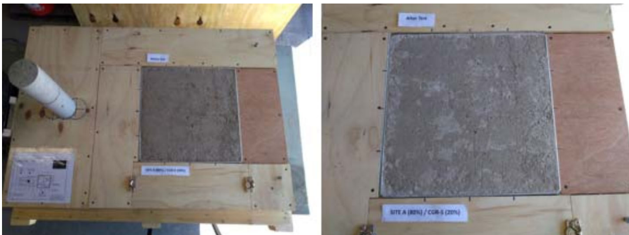
Figure 40: Views of WETA and Compacted Soil Form During Wind Erosion Test, Photos by Patrick Bollinger
