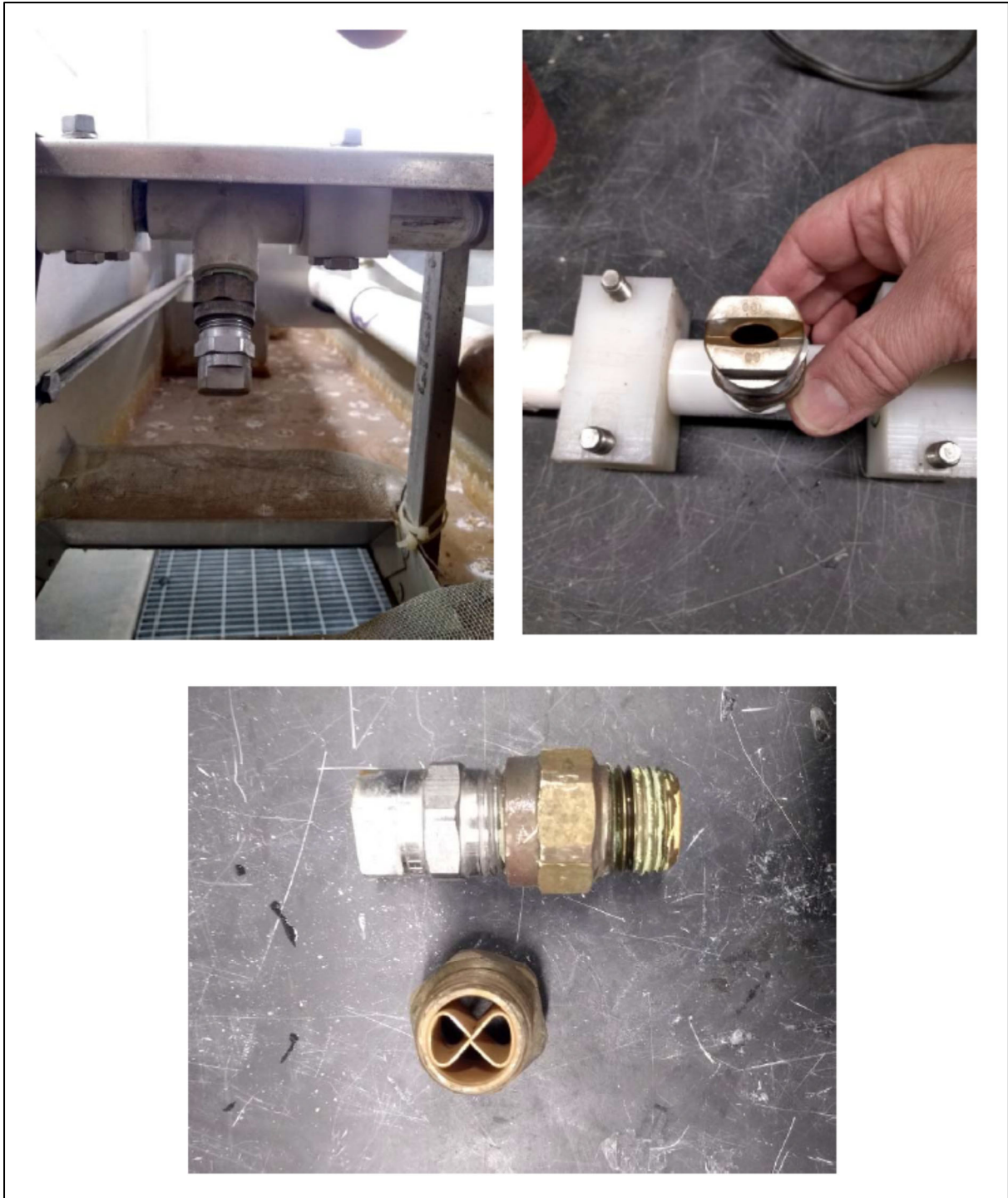
Figure 58: VeeJet Model 80100 Nozzles in Rainfall Simulator at Iowa State University, Photos by Patrick Bollinger
