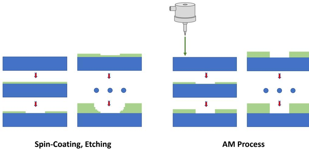
Figure 1.10: Left: dielectric material is spin-coated and processed one layer at a time, involving patterning and etching. Right: AM processes allows for final dimensions to be fabricated in as few steps as needed.
