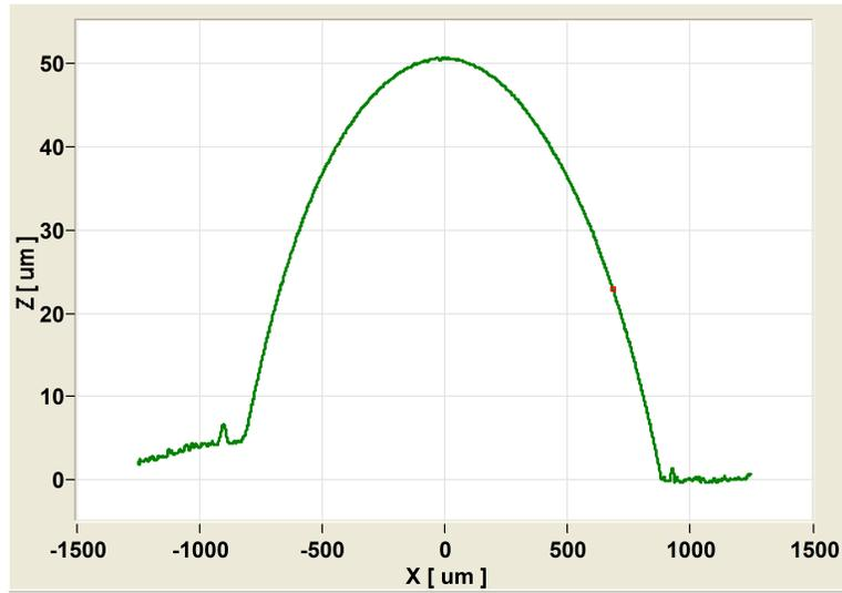
Figure A.2.7: Profile of BCB lens printed on top of patch antenna.
