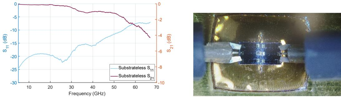
Figure 3.22: (a) S-Parameters of substrate-less BCB package containing two devices. (b) Photo image of the measurement.
