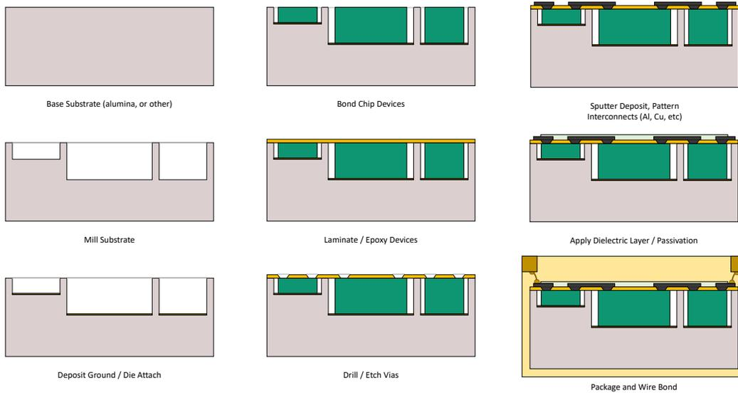
Figure 1.5: Diagram of GE High Density Interconnect fabrication technique used in the 1990s [1].
