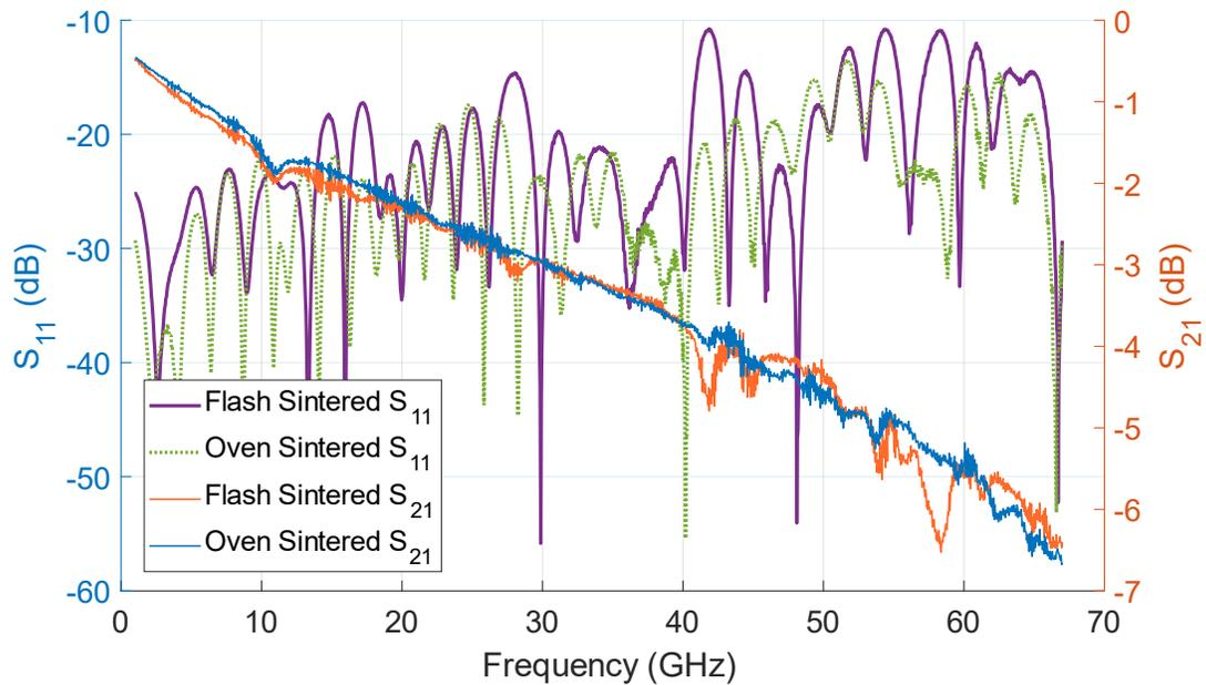
Figure 2.9: 34 mm long microstrip transmission line printed on LCP. S-parameters shown for both the UV and oven sintered samples.
