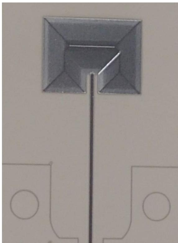
Figure 2.13: UV sintered AJP printed antenna on an LCP substrate.
