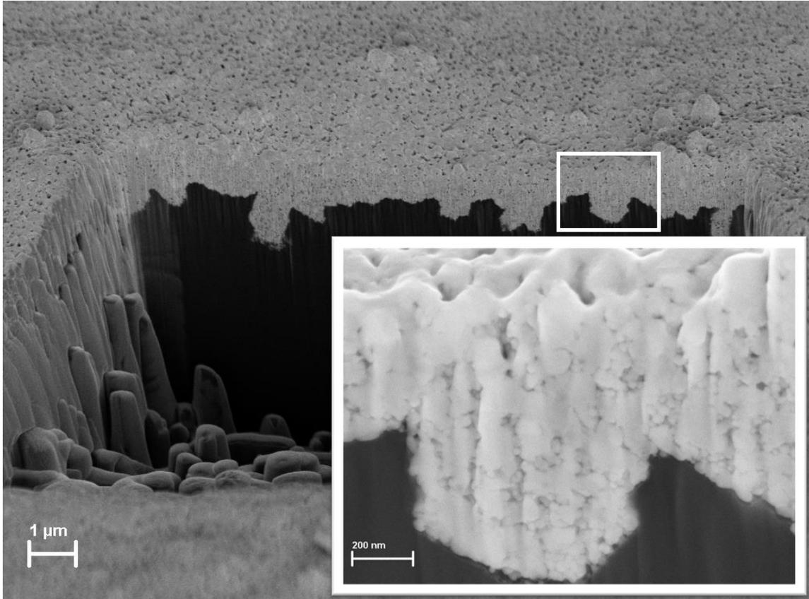
Figure 2.8: FIB cross-section SEM image of Thermal (Oven) Sintered AgNP ink (light grey) on LCP (dark grey).
