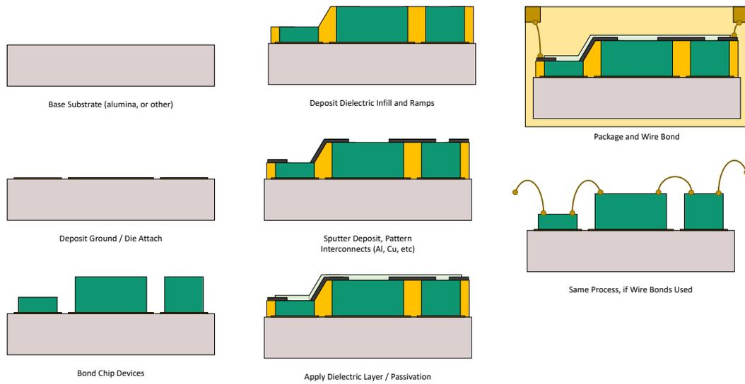
Figure 1.6: Diagram of Chip First/Chip Last fabrication technique used to encapsulate devices on substrate surfaces.
