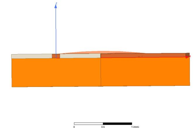
Figure A.2.6: Patch With  $50\ \mu\text{m}$  Dielectric Lens 3D model from HFSS simulation
