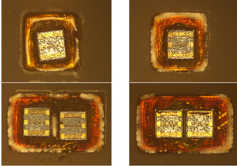
Figure 3.12: Microscope photo images of manual placement chips before removal of protective PMMA film and printing of AgNP interconnects. Left show purposefully offset angles, while right show careful alignment and appropriate distancing of chips.
