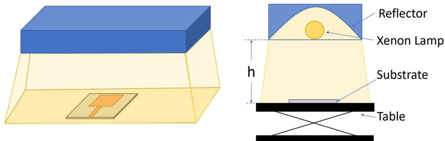
Figure 2.1: Illustration of the flash sintering system.
