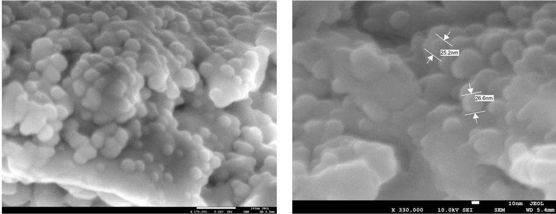
Figure 2.7: SEM images of AgNPs sintered into tight clusters with average 30 nm diameters (left: X 170,000, right: X 330,000).
