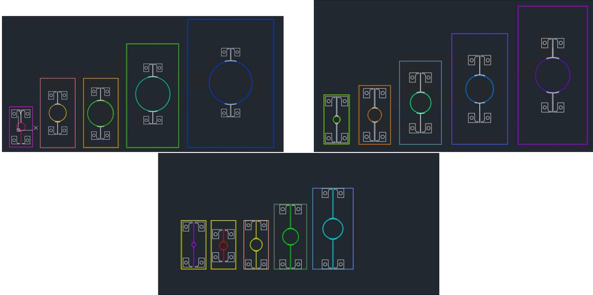
Figure A.1.2: Set of 10, 15, 25 GHz ring resonators on 4 MIL thickness LCP. Measured with no surface dielectric loading and then after dielectric loading to determine dielectric permittivity of printed BCB films.
