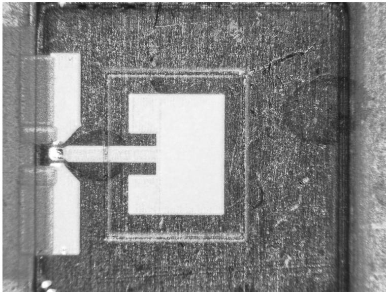
Figure A.2.8: Lens Barrier Fabrication.
