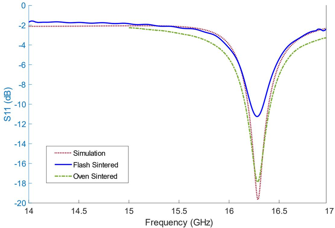
Figure 2.11: S-Parameters of patch antenna sintering comparison.
