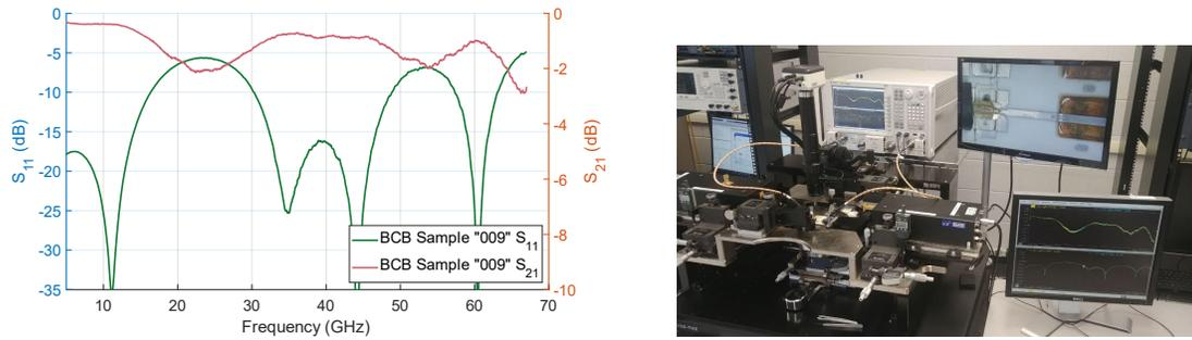
Figure 3.10: (a) S-Parameters of 2 mm BCB fill with transmission line interconnection to LCP. (b) Photo image of measurement setup for GSG probe station.
