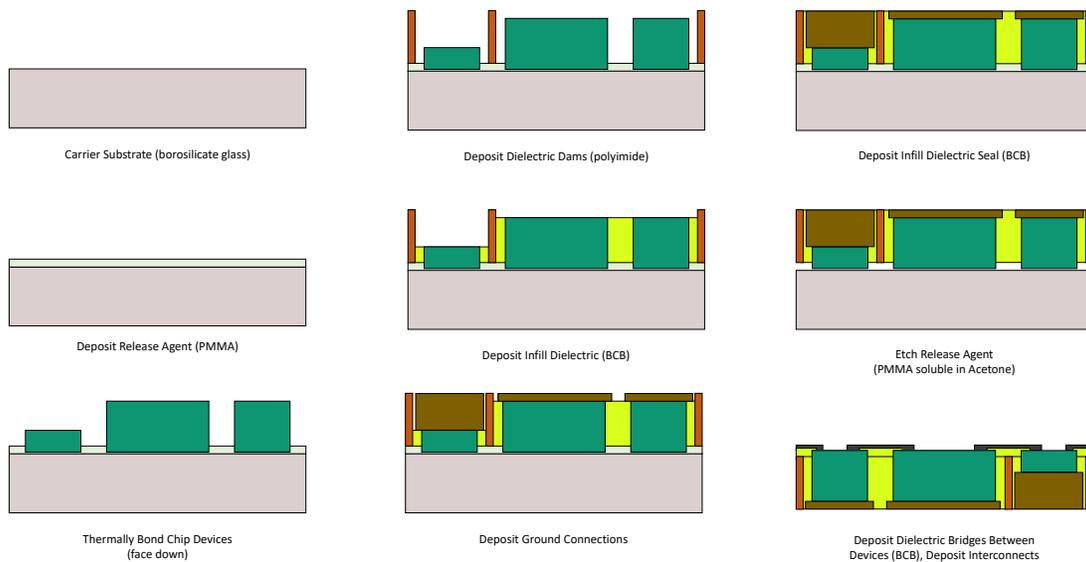
Figure 1.8: Diagram of Substrate-Less fabrication technique used in this research to print packages with fully AM processes.
