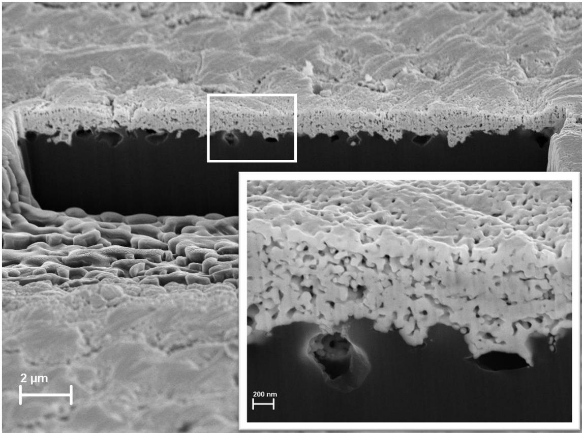
Figure 2.6: Cross-section SEM image of UV Flash Sintered AgNP ink (light grey) on LCP (dark grey).
