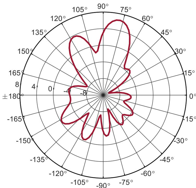
Figure 2.12: Polar pattern of UV sample patch with gain 6.69dBi.
