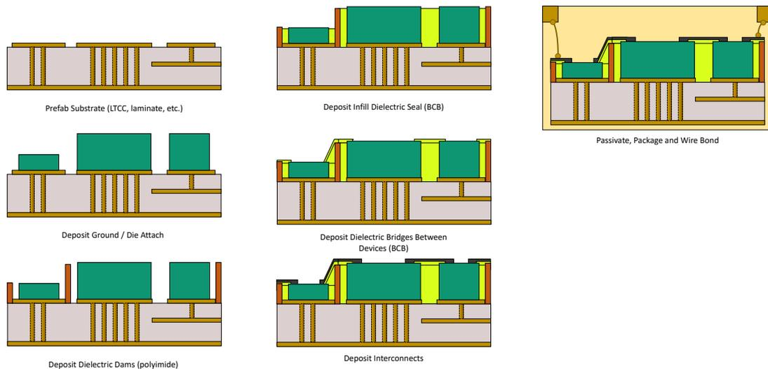
Figure 1.9: Diagram of Substrate-Less on PCB fabrication technique as compliment to Chip Last fabrication approach.
