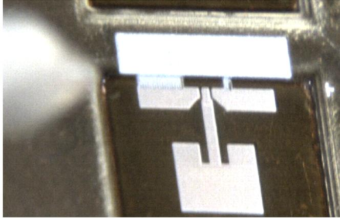
Figure 3.17: Process Camera capture of 30-degree angle printing on Patch Antenna ground connection using Ag ink.
