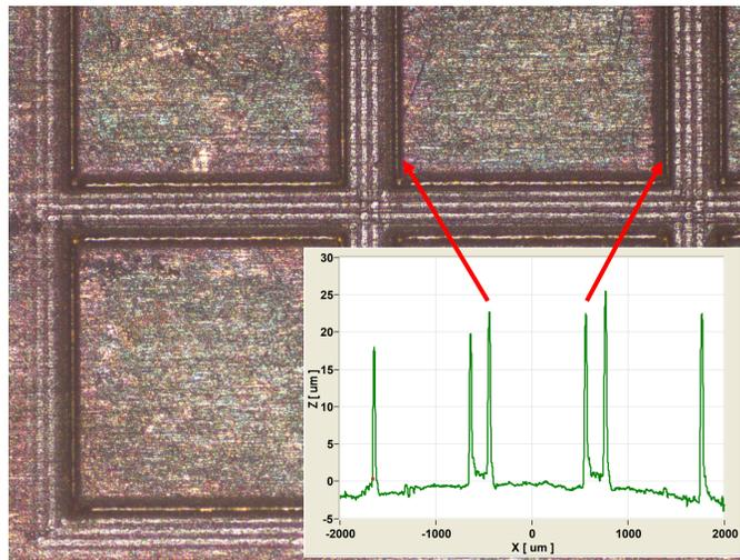
Figure 3.4: Fabricated cells for varied height dielectric dams, no fill material placement in this step.
