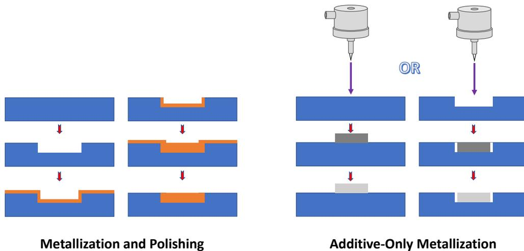
Figure 1.2: Left: mechanical polishing of unwanted metal layers must be performed, alongside pattern and etch lithography to reach desired metal patterns. Right: AM methods allow for the final metal pattern to be achieved in the first steps, without removal of unwanted material.
