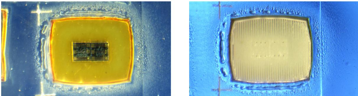
Figure 3.21: Fabricated substrateless package. Left: face side of the dice. Right: ground plane printed on back with AgNP ink.
