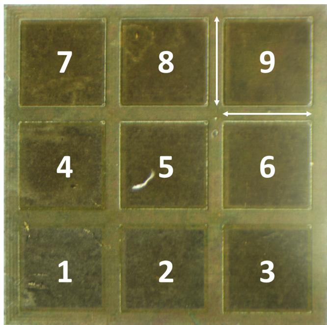
Figure 3.5: Dielectric array with varying BCB thickness,  $5\ \mu\text{m}$  to  $45\ \mu\text{m}$  (1 - 9 layers)
