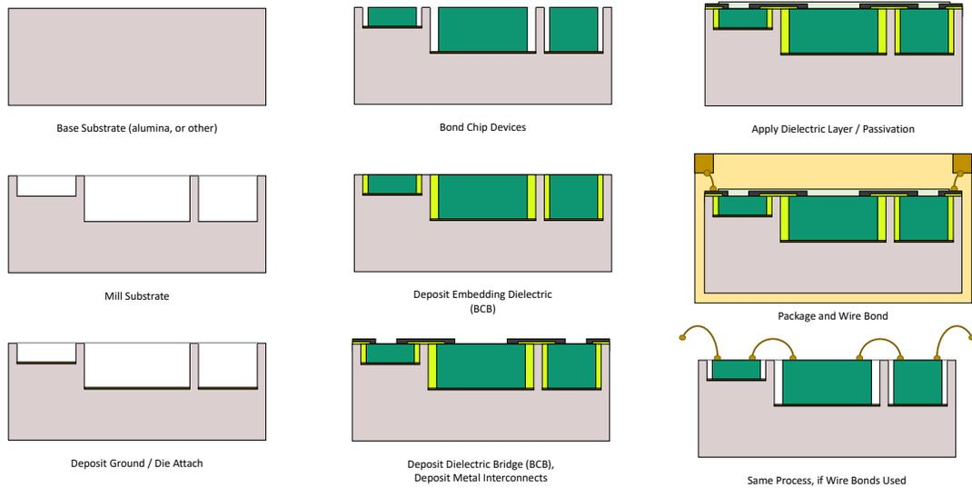
Figure 1.7: Diagram of Embedded Devices fabrication technique used to encapsulate devices embedded in cavities etched into substrate surfaces.
