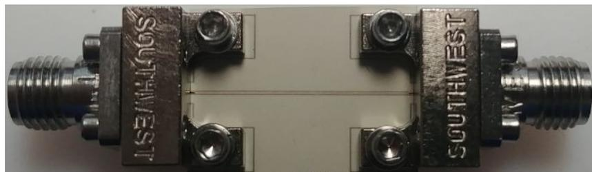
Figure 2.10: Connectorized Ag transmission line on LCP.
