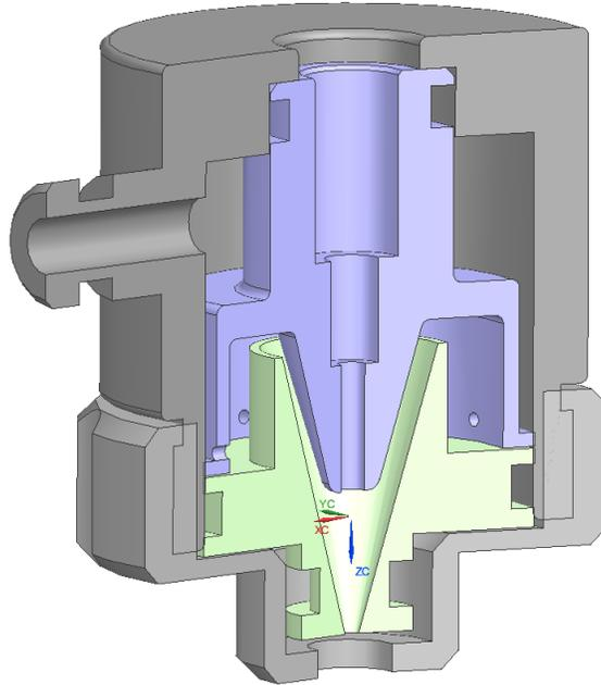
Figure 1.1: Cutaway view of Optomec 5x print head.
