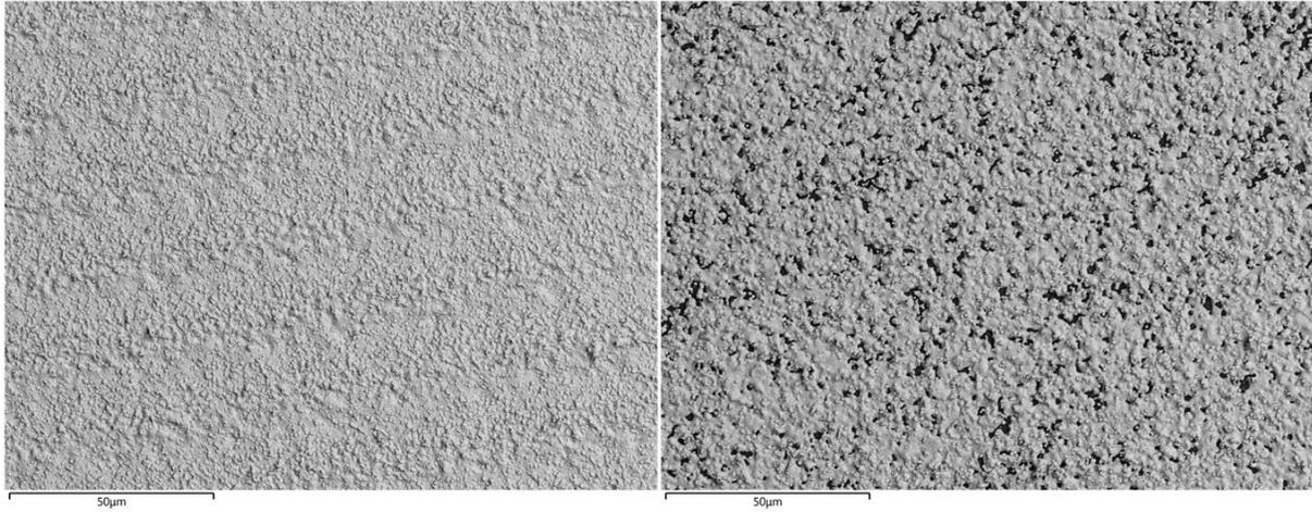
Figure 2.5: SEM images of as-printed (left) and UV Flash Sintered (right) AJP Silver NPs on Si.
