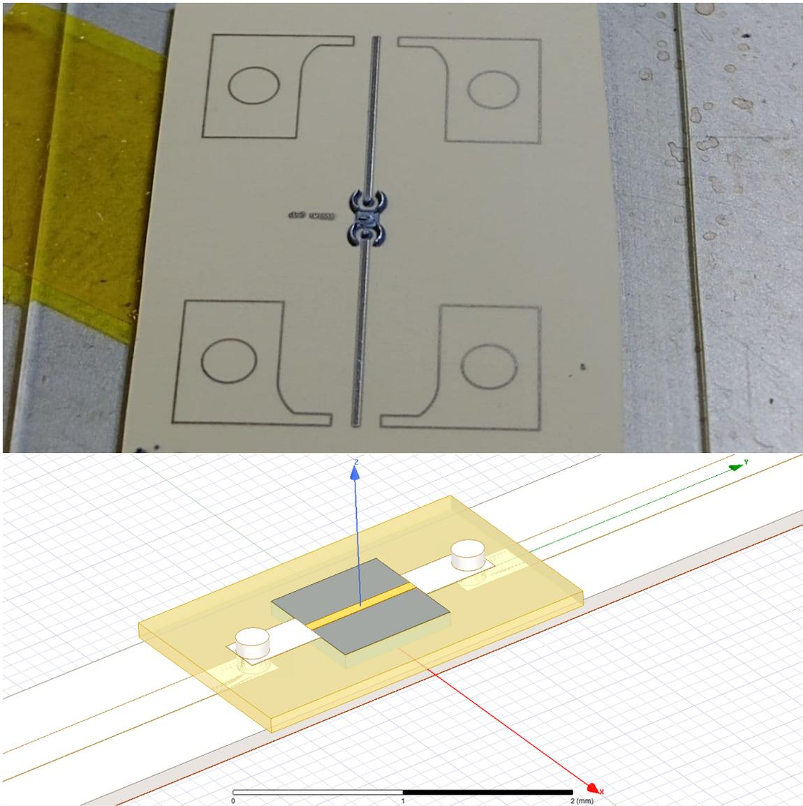
Figure A.2.10: 3D render of Coaxial Chip Interconnection
