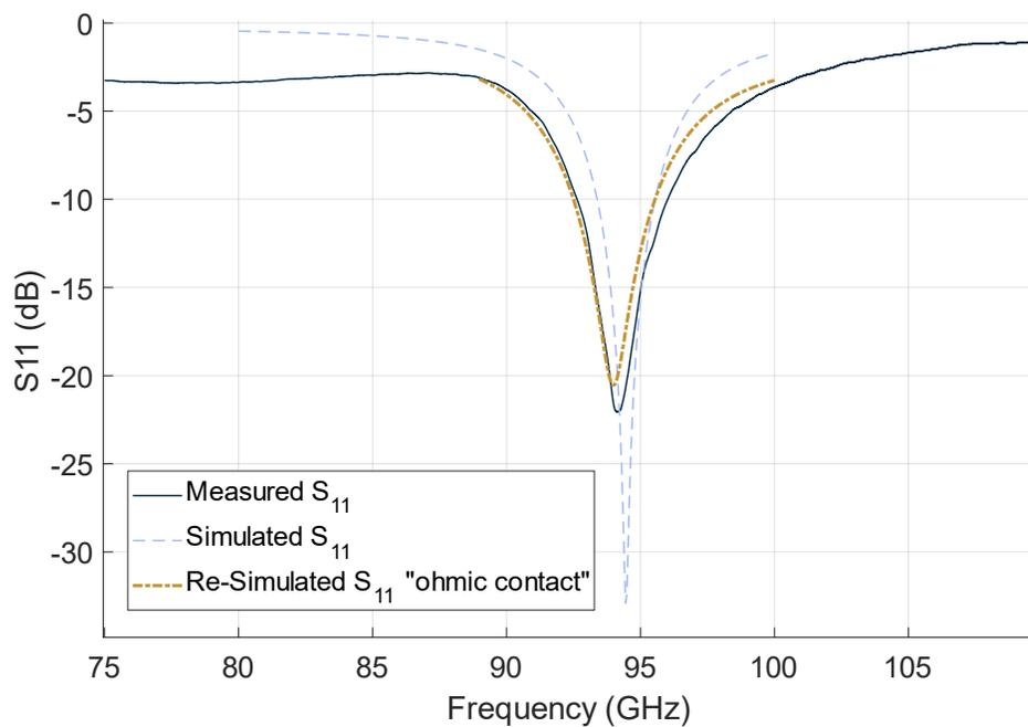
Figure 3.18: Measured and simulated  $S_{11}$  of the patch antenna, including a re-simulation with series resistance added for probe to silver contact.
