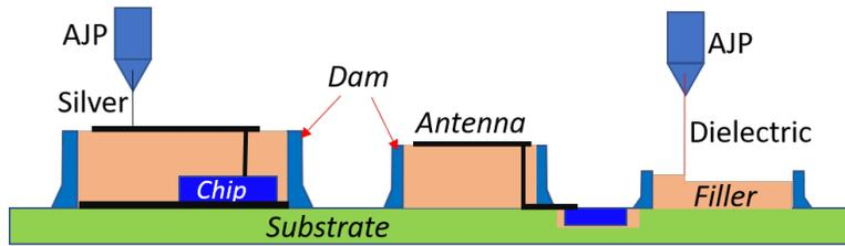
Figure 3.1: Selective dielectric deposition using a dam and filling process.
