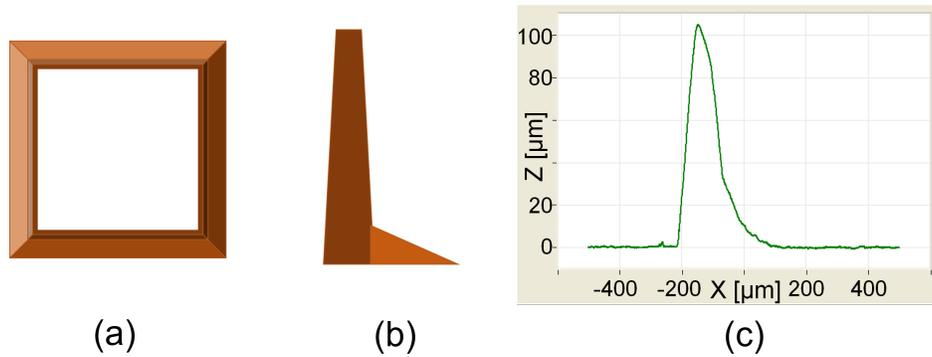
Figure 3.3: (a) Top-down view of dam; (b) Cross-section view of brim and wall; (c) 2D scanned profile of the dam wall.
