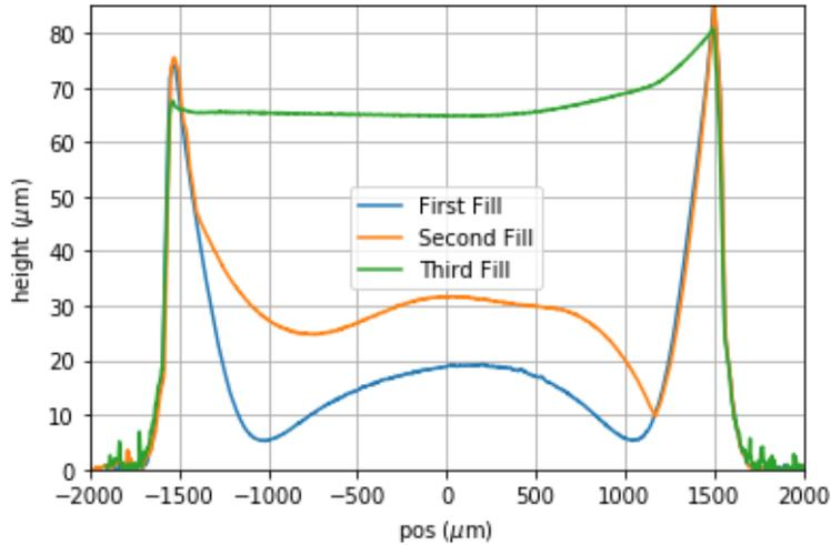
Figure 3.15: Left: 2D Profile of the dam with multiple fillings; Right: Printed Ag patch antenna on filled BCB.
