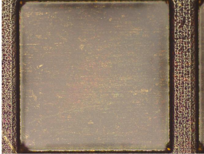
Figure 3.6: 3 mm x 3 mm Dielectric dam fill with 45  $\mu\text{m}$  BCB thickness.
