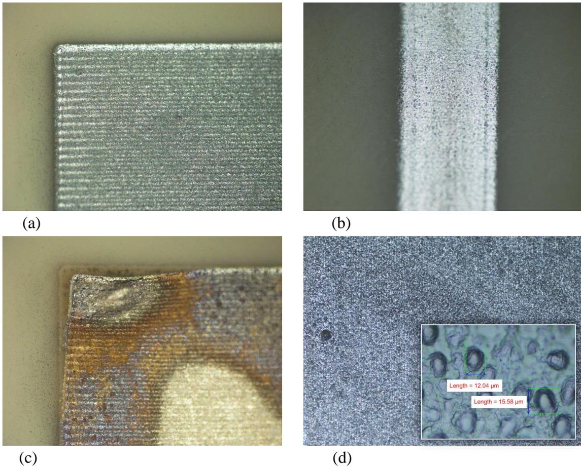
Figure 2.3: (a) Wet AJP Ag ink. (b) Flash UV sintered AJP Ag ink. (c) Delamination of Ag ink under flash UV sintered layers. (d) Bubbles formed under Ag ink during flash UV sintering.
