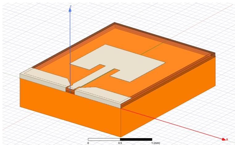
Figure 3.14: Patch antenna 3D model exported from HFSS simulation.
