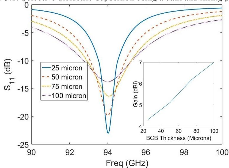
Figure 3.2: Simulation of 94 GHz patch antenna on BCB with thickness from 25 to 100  $\mu\text{m}$ . Superimposed gain at resonance.
