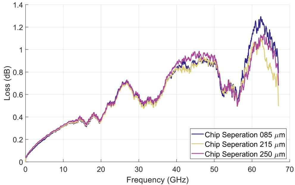
Figure 3.13: Losses: Chip Spacing over DC - 67 GHz. Distance between the chips were varied from 85 to 250  $\mu\text{m}$ .
