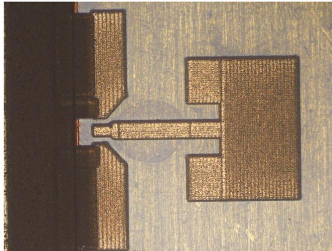
Figure 3.16: Left: 2D Profile of the dam with multiple fillings; Right: Printed Ag patch antenna on filled BCB.
