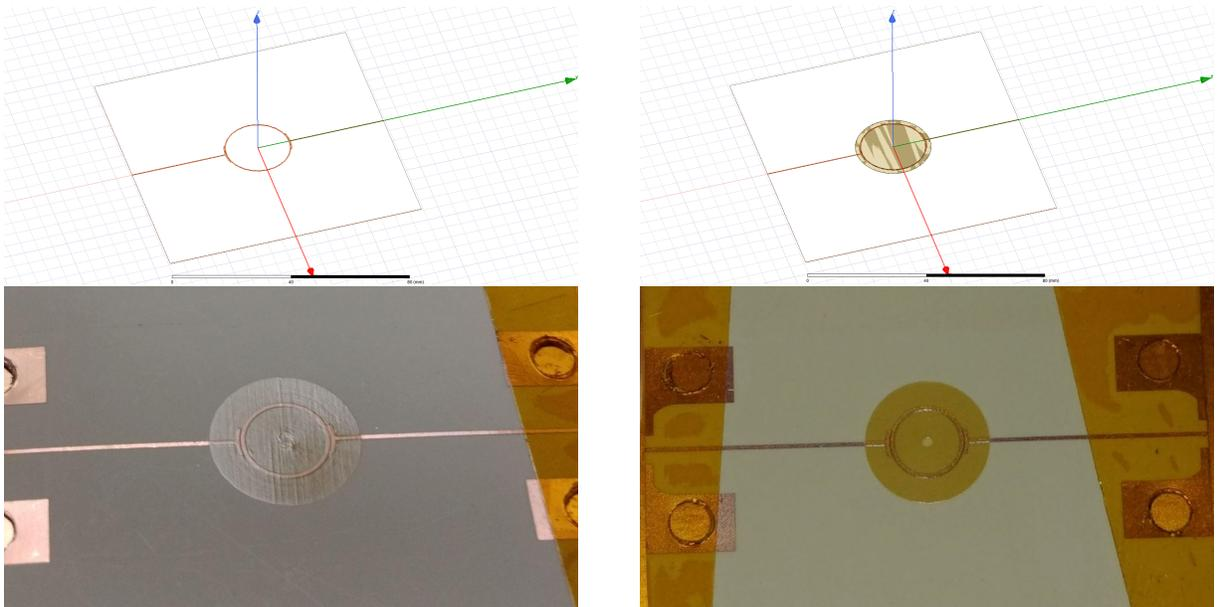
Figure A.1.1: Dielectric Verification using 14 GHz unloaded and loaded ring resonator on etched LCP.
