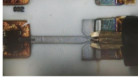
Figure 3.8: (a) S-Parameters of embedded 0 dB GaAs single chip in BCB with interconnection to LCP. (b) Photo image of the measured circuit.
