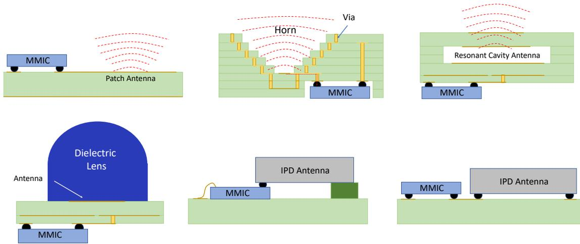
Figure 1.4: Various embedded and integrated MMIC circuits formed as integral active MMW systems.
