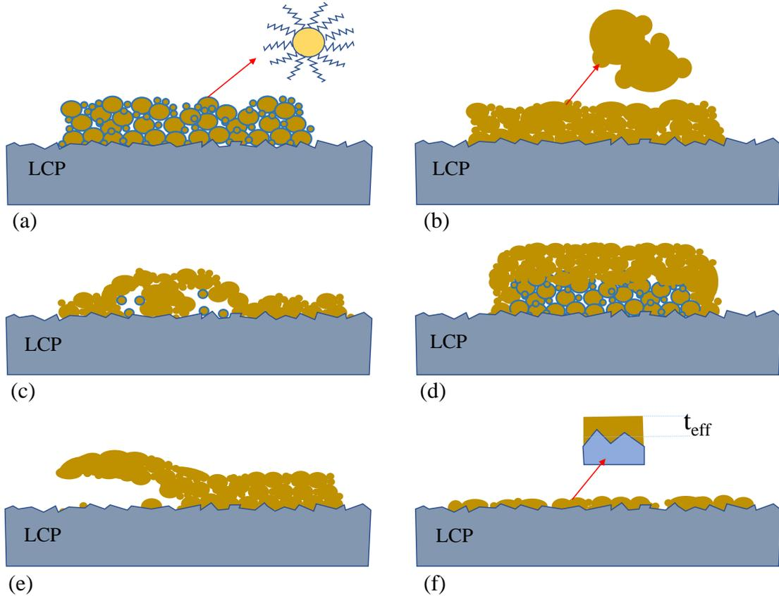
Figure 2.2: Illustration of the flash sintering symptoms. (a) As deposited Ag ink. (b) Fully sintered film. (c) Sintered particles with air-pockets. (d) Sintered outer-layer of particles with wet defects below. (e) delamination of Ag film from substrate. (f) Thin Ag film on rough surface.
