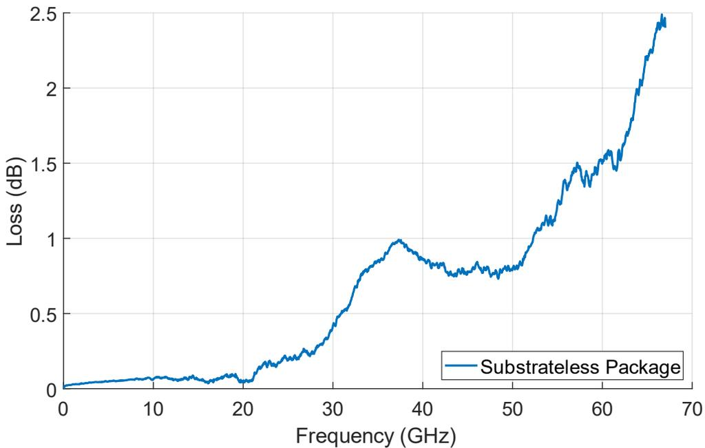
Figure 3.23: Losses: Substrate-less package over DC - 67 GHz. Distance between the chips were  $23 \mu\text{m}$  [ $77 \mu\text{m}$  pad-to-pad spacing].
