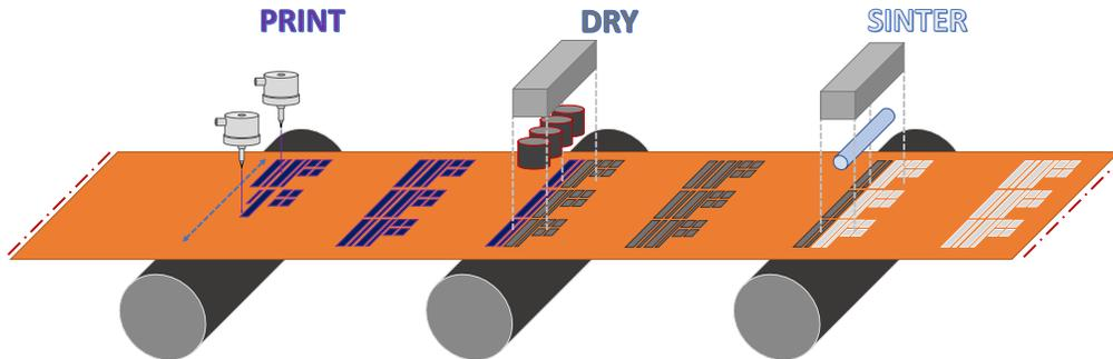
Figure 1.3: Proposed Reel to Reel fabrication using AJP and flash sintering for conductive traces.
