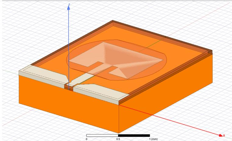
Figure A.2.5: Patch with BCB lens 3D model from HFSS simulation
