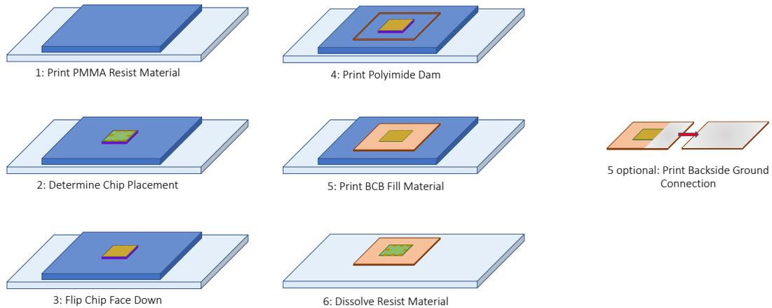
Figure 3.20: Fabrication steps used to make a substrateless package for bare die chip devices.
