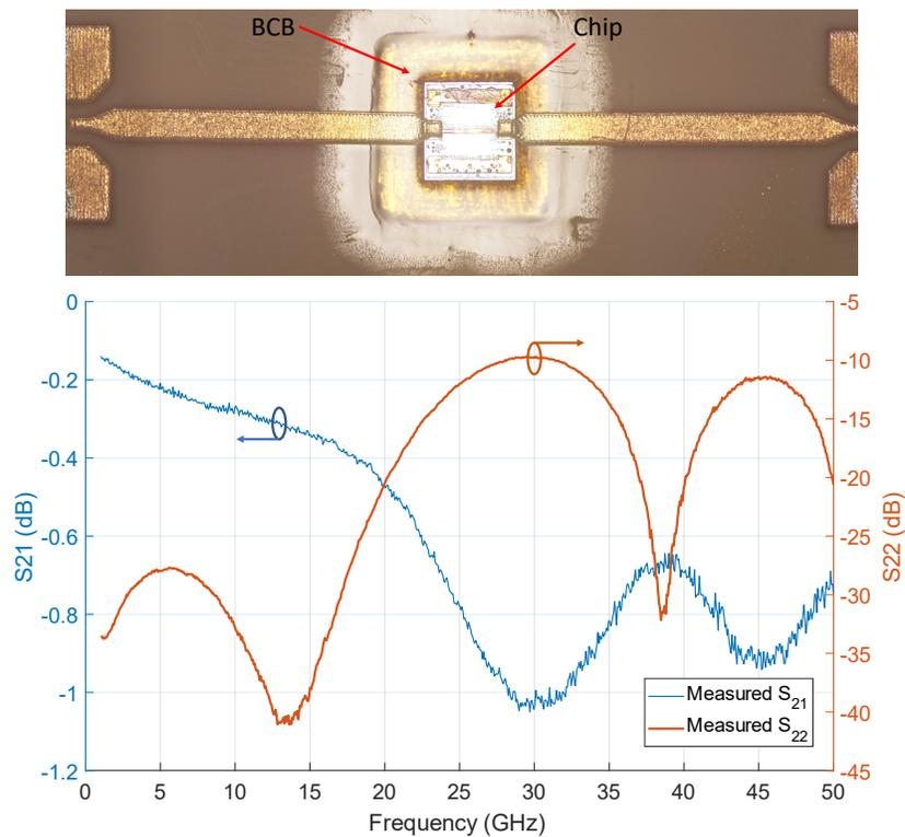
Figure 3.11: Measured S-Parameters of embedded chip in a cavity.
