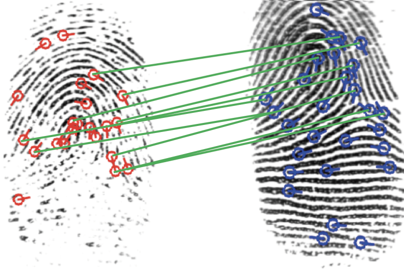
Figure 1.12 Example of minutiae match between two fingerprint impressions of the same finger. This example highlights the difficulty of minutiae matching given a poor quality enrollment image (left) which has many missing minutiae. Despite this difficulty, a COTS minutiae matcher is able to correctly match these two fingerprints with a score of 150, well above the score threshold of 69 @ FAR = 0.01\% . Fingerprints retrieved from the FVC 2004 DB1 A database [109]
