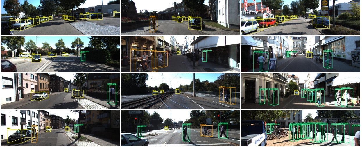
Figure 4.5: Qualitative Examples. We visualize qualitative examples of our method for multi-class 3D object detection. We use yellow to denote cars, green for pedestrians, and orange for cyclists. All illustrated images are from the val1 [24] split and not used for training.
