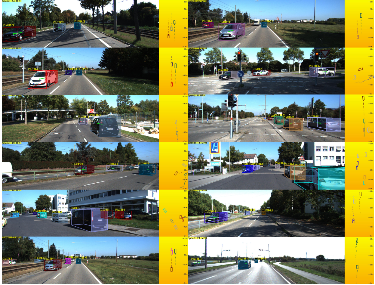
Figure 5.6: Qualitative Examples. We depict the image view (left) and BEV (right). We show velocity vector in green, speed and ego-motion in miles per hour (MPH) on top of detection boxes and at the top-left corner, and tracks as dots in BEV.
