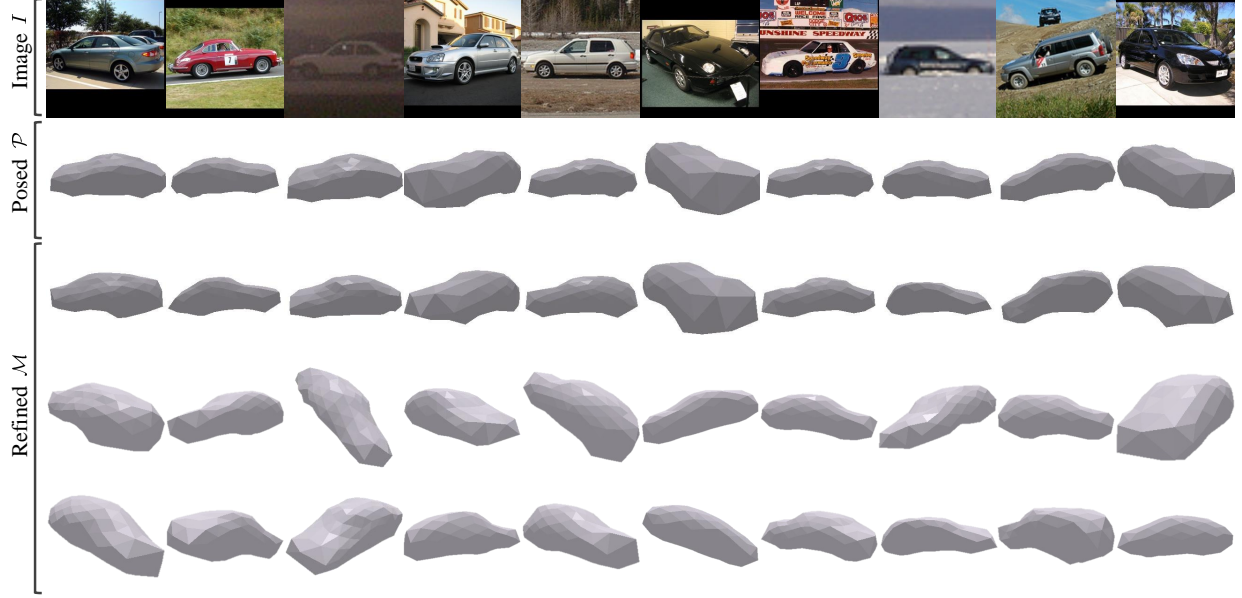
Figure 6.7: Qualitative 3D mesh reconstructions on additional Pascal3D+ cars. We visualize input image (row 1), posed template (row 2), and the refined mesh (row 3 – 5) in view coordinates from two additional novel viewpoints.
