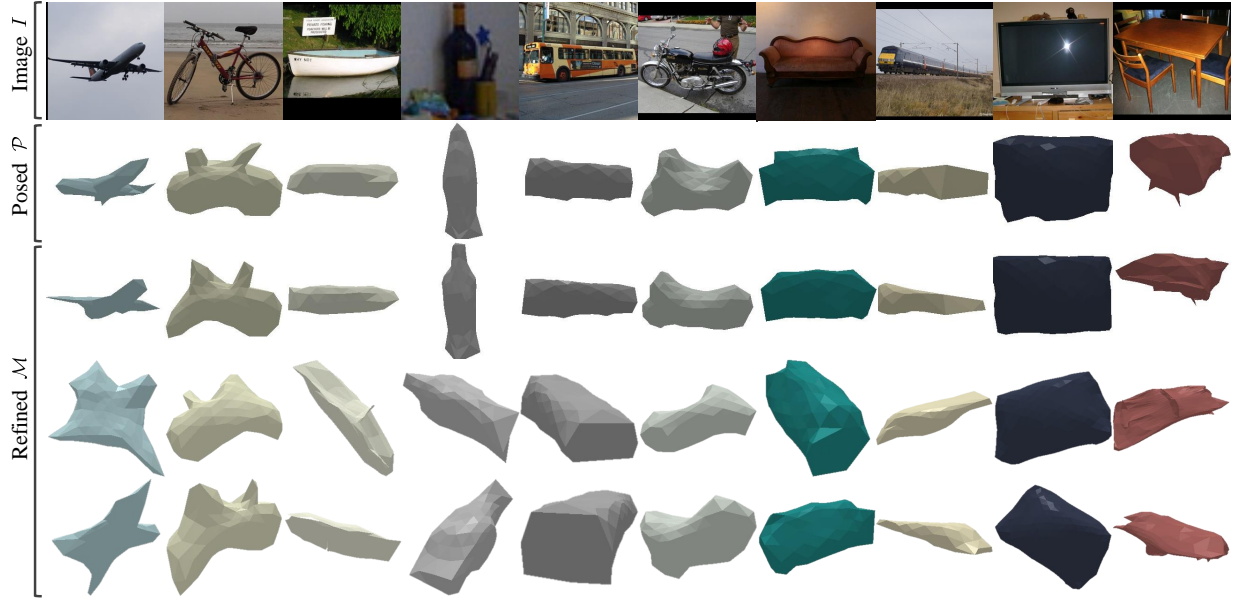
Figure 6.10: Qualitative 3D mesh reconstructions on additional Pascal3D+ categories. We visualize input image (row 1), posed template (row 2), and the refined mesh (row 3 – 5) in view coordinates from two additional novel viewpoints.
