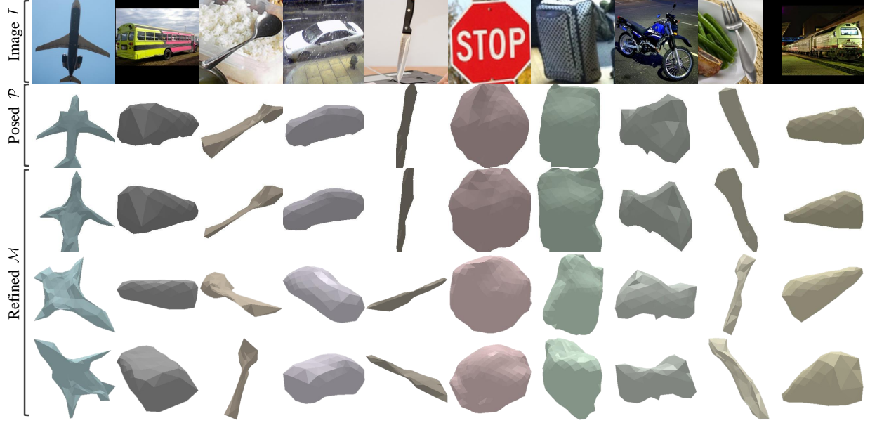
Figure 6.9: Qualitative 3D mesh reconstructions on additional COCO categories (right). We visualize input image (row 1), posed template (row 2), and the refined mesh (row 3 – 5) in view coordinates from two additional novel viewpoints.
