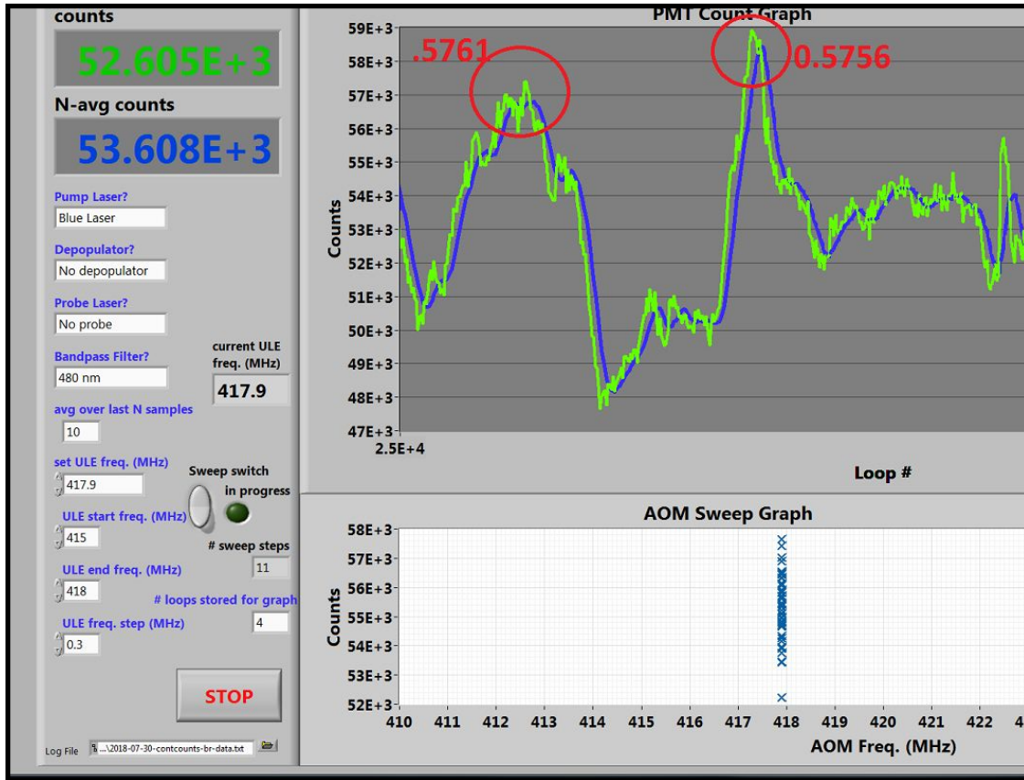
Figure 4.8: A screenshot of the VI I wrote for recording PMT counts for the branching ratio measurements.
