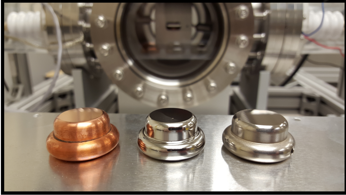
Figure 3.2: From left to right: a copper, niobium, and titanium electrode.
