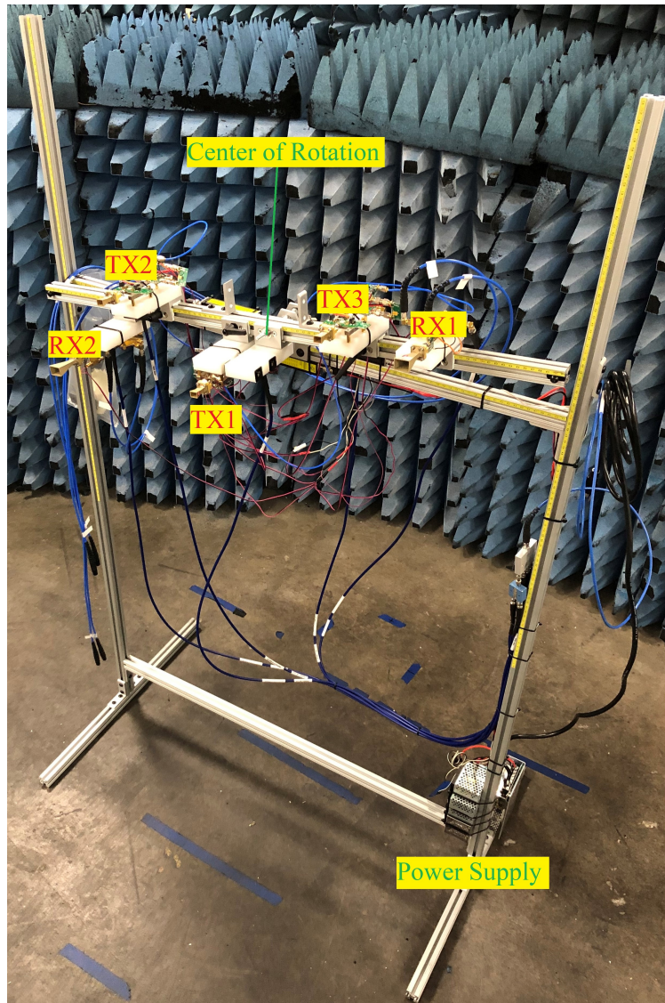
Figure A.4: First iteration of the implemented dynamic antenna array. Two receivers' adjustable baseline range was [60.0 cm, 83.6 cm], or [76\lambda, 106\lambda] based on 38 GHz.
