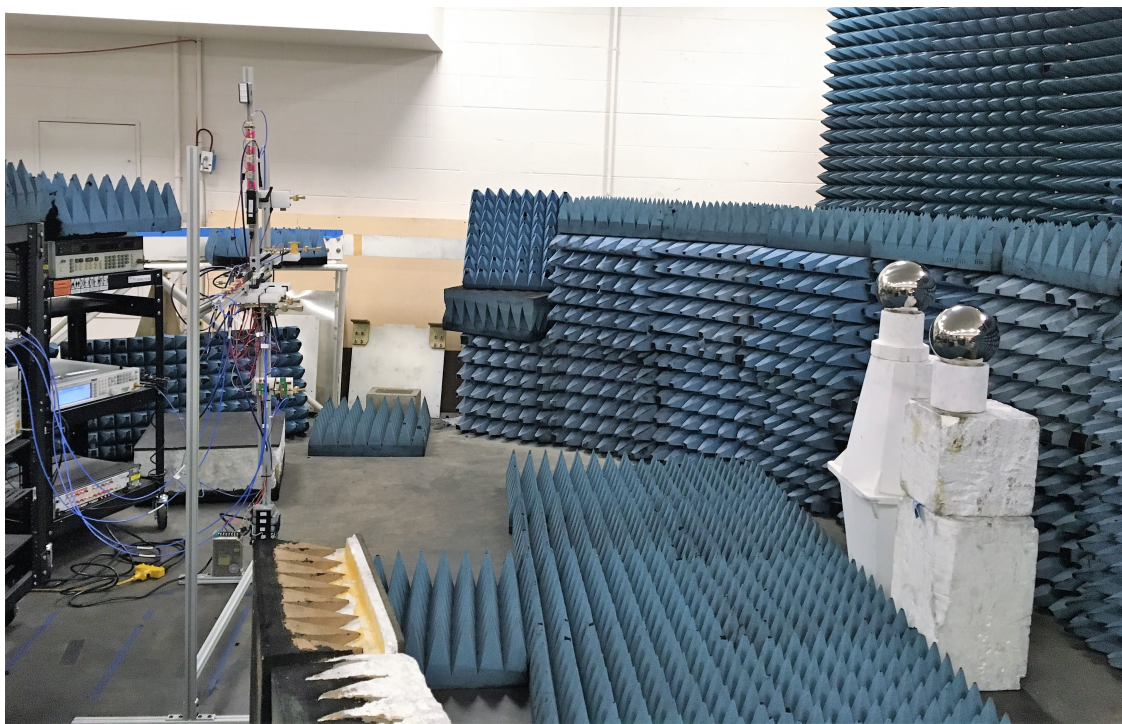
Figure 3.1: Side view of the experiment setup of two reflecting spherical targets backed by walls of RF absorbers in a 7.6 m semi-enclosed arch range. [2].
