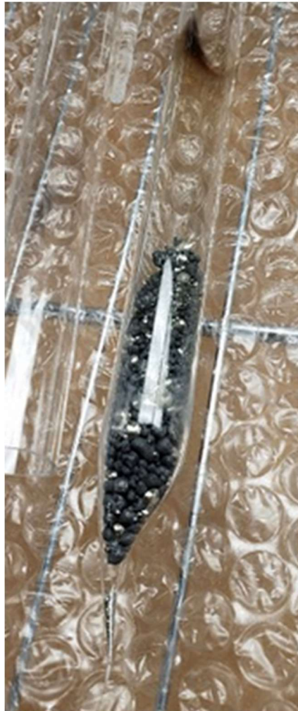
Figure 14. Sealed crucible, showing sharp tip, 'dimple' from pressure checking, and sample precursor materials within.
