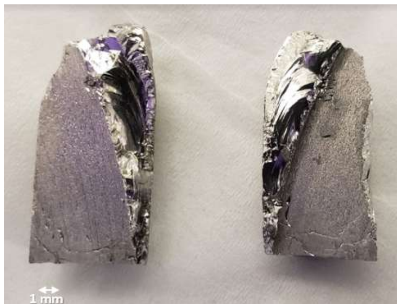
Figure 36. Image of a fracture surface of sample 13, a large-grained polycrystalline Sn. 9 Ge. 1 Te ingot, showing fracture along the boundaries of both large and small grains within the ingot- the large grains denoted by faceting, the small grains denoted by a ‘woody’ appearance.
