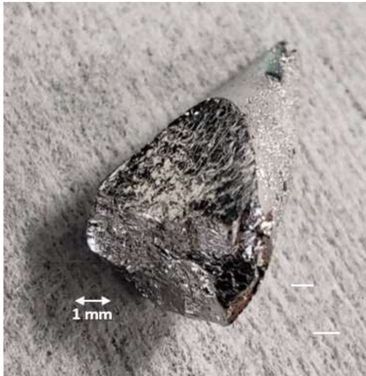
Figure 35. Image of a fracture surface of sample 20, a polycrystalline \text{Sn}_{.8}\text{Ge}_{.2}\text{Te} ingot, showing a ‘wood-grain’ texture that stems from a structure comprised of a multitude of small grains.
