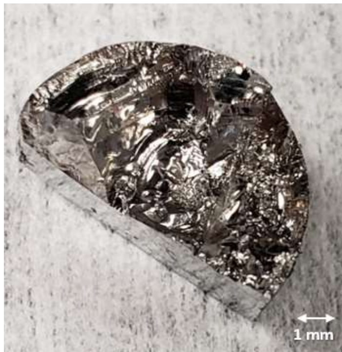
Figure 37. Image of a fracture surface in sample 18, a single-crystal \text{Sn}_{.8}\text{Ge}_{.2}\text{Te} ingot, showing extensive faceting and no areas of small-grained, 'woody' texture, indicating that the entire sample is comprised of one large grain.
