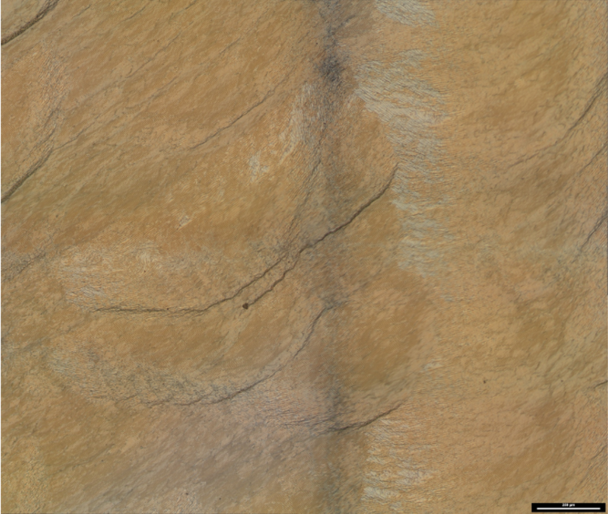
Figure 8.36: Mosaic Boundary at higher magnification showing consistently smooth step flow growth over the interface.
