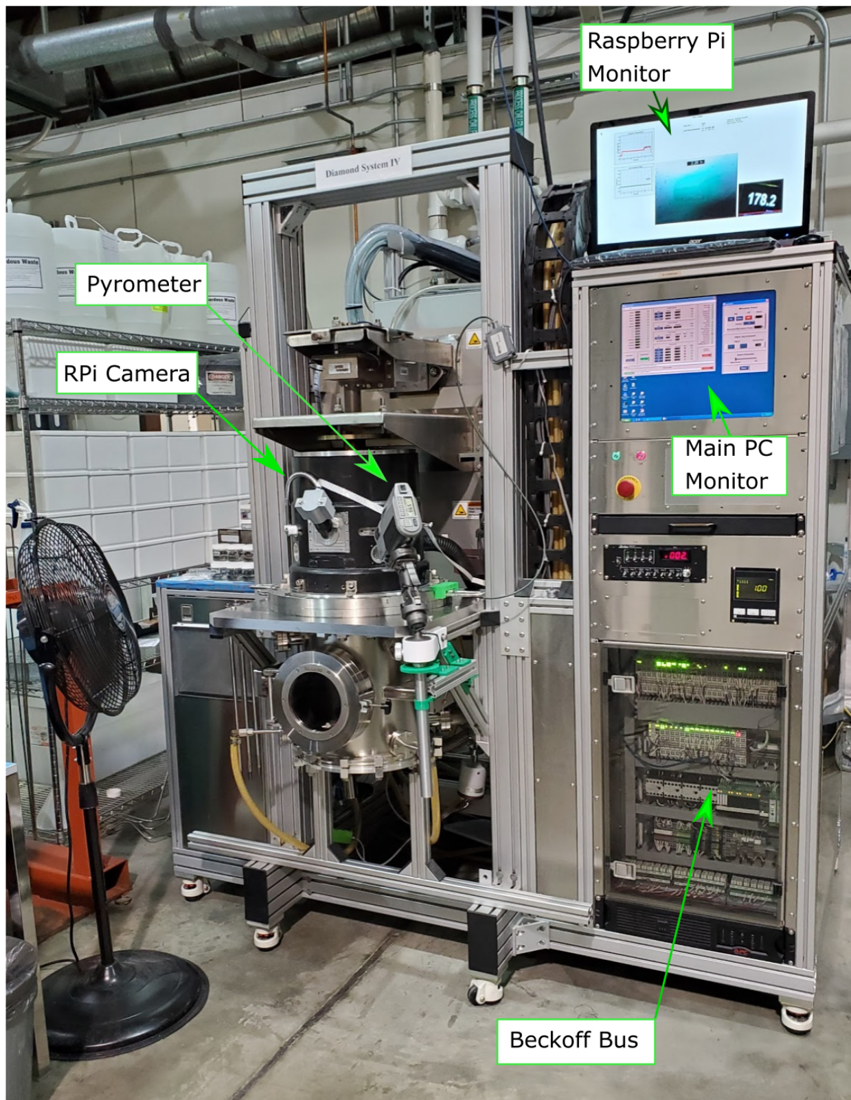
Figure 4.11: Diamond System 4 (DS4) during normal operation.
