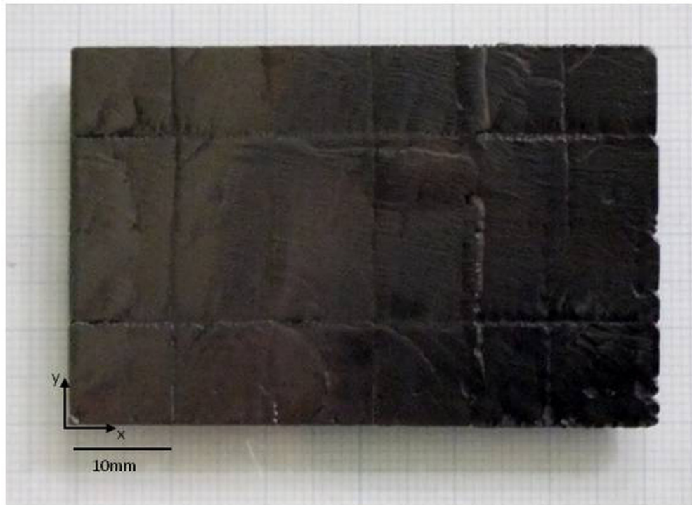
Figure 3.55: A 40 \times 60 \text{ mm}^2 as-grown mosaic wafer with thickness of 1.8 mm [235].
