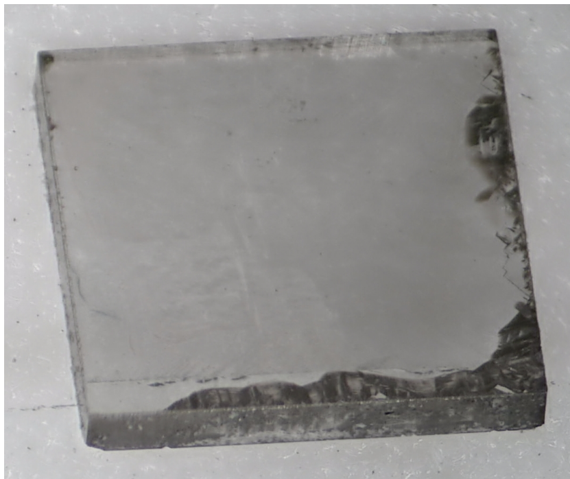
Figure 9.3: Separated CVD grown plate, 400 \mu\text{m} thick.
