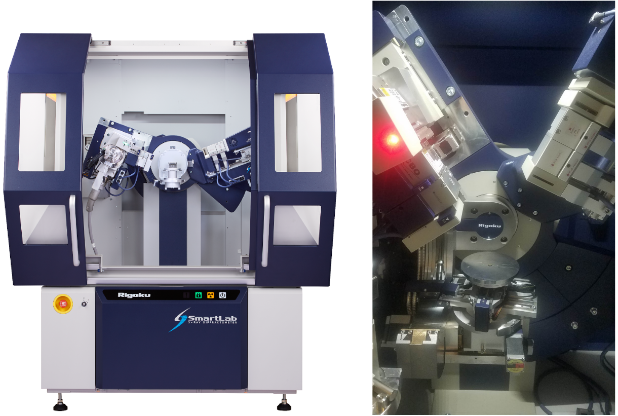
Figure 5.19: a) Stock photo of the Rigaku Smartlab system [269]. b) System performing a wide angle \theta - 2\theta scan.
