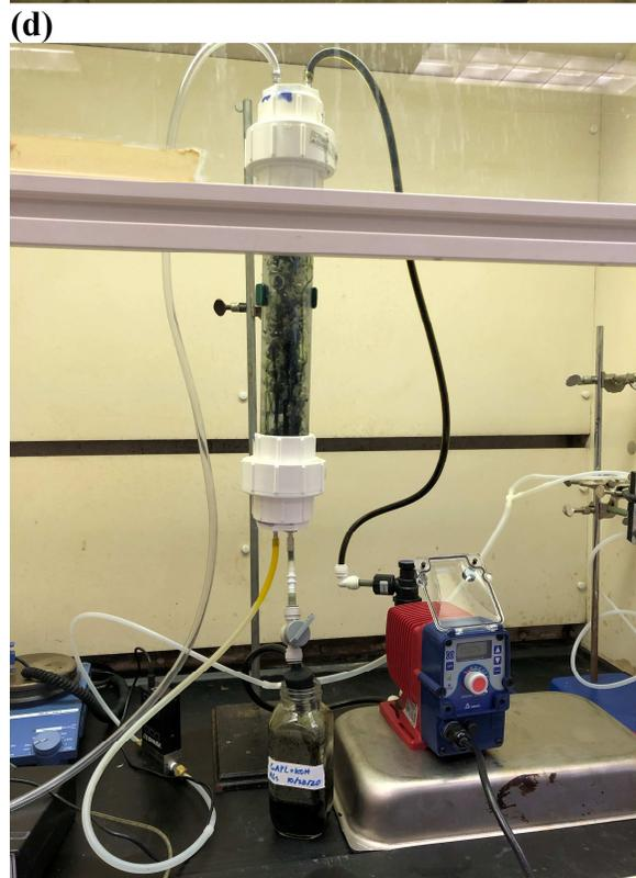
**Figure 84:** Absorption Experimental Setup Photo **a)** not in use **b)** gas flow control setup **c)** column in use **d)** setup in use
