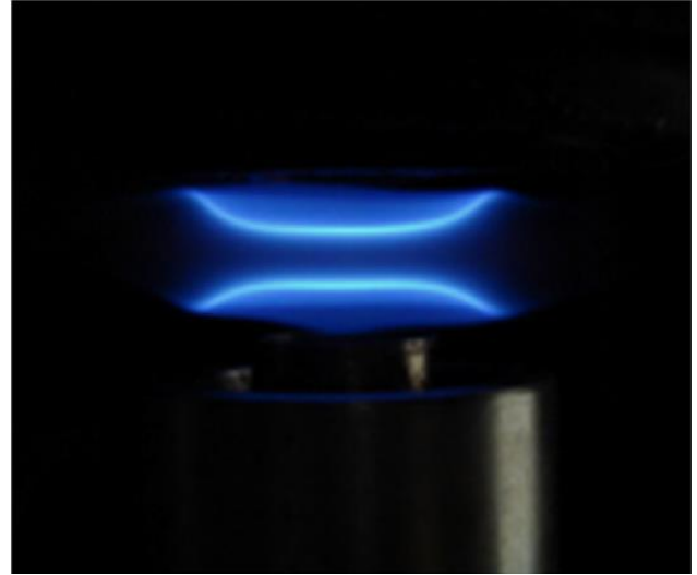
Figure 2-2. Twin counter-flow/stagnation flames, retrieved from [13].
