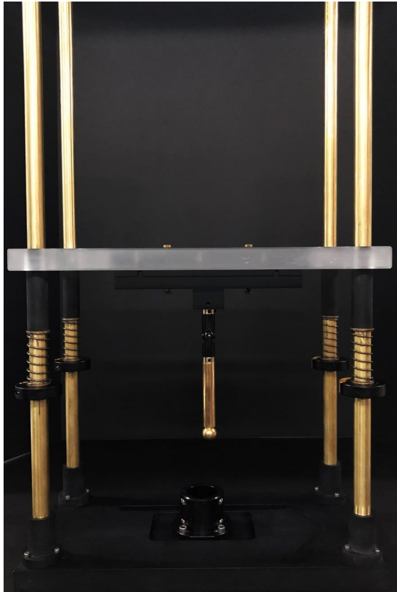
Figure 4.6. Final custom-built loading press used in this study
