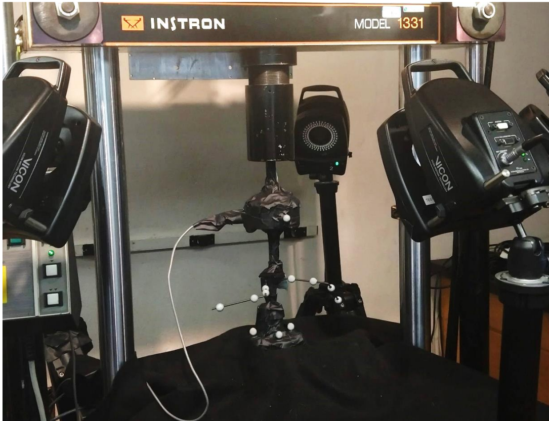
Figure 2.2. Photograph depicting the testing set-up of the Vicon optical tracking system
