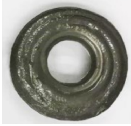
(b) Printed multi-permeability iron core.
