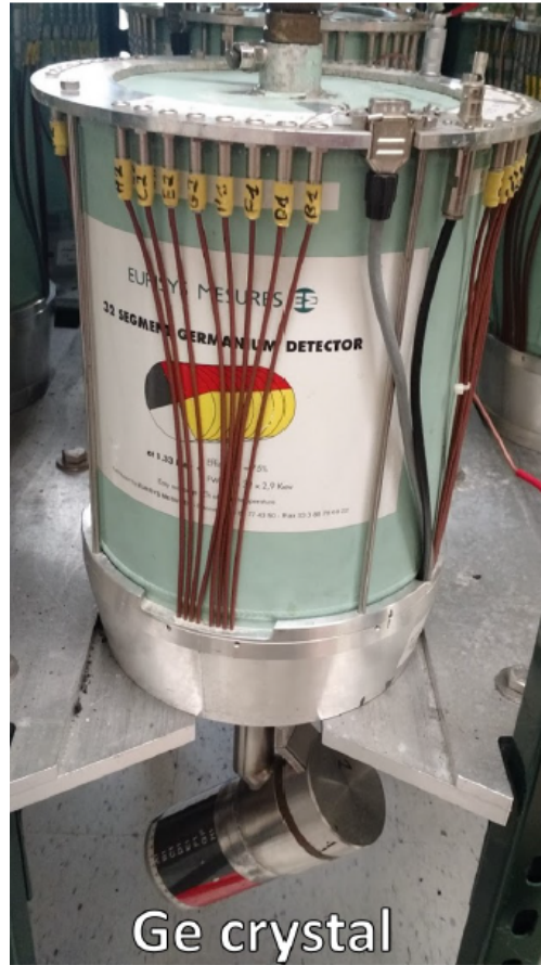
Figure 3.15: A single SeGA detector. The large green cylinder is the liquid-nitrogen dewar. The germanium crystal is located in the aluminum housing at the bottom of the photo. Figure from [108].
