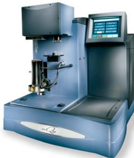
Figure 8 - TA TGA Q500 thermogravimetric analyzer (Image ©2020 TA Instruments/Waters Corporation reproduced with permission from [64].)
