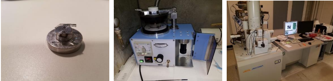
Figure 40 - (a) Samples 2 and 4 mounted on aluminum stub (b) Pure osmium coater Neoc-AN (c) JEOL JSM-7500F SEM
