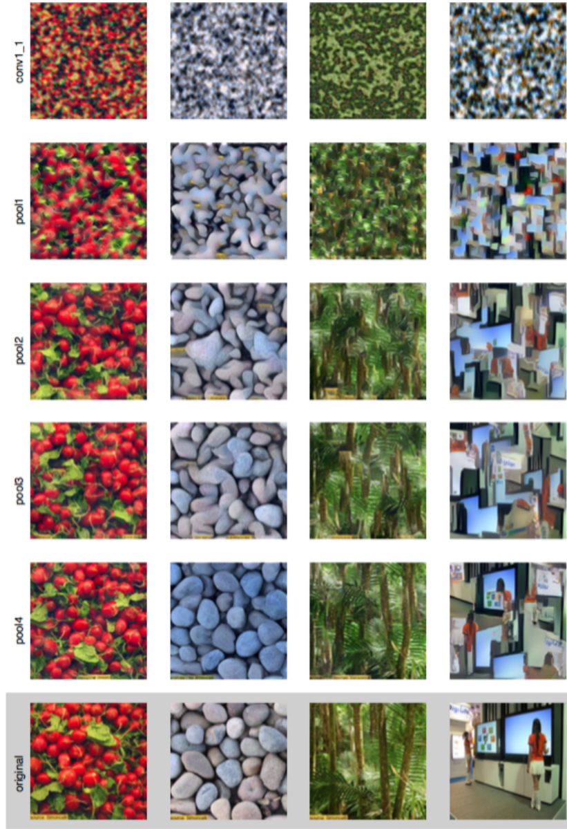
Figure 2.4 Synthesis results with different layers. The last row shows the original images. The first row shows synthesized image by matching statistics from only "conv1-1" layer and the second shows that matching statistics from "conv1-1" and "pool1" layers and so on. With only lower layer statistics, the synthesis lose information of the texture. Adding statistics from deeper layers improves the performance, which proves higher layer statistics are necessary to capture texture information. The last column shows result of a natural image, which has more localized structure and is not stationary.
