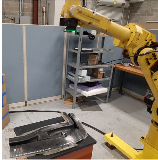
Figure 5.20: Physical setup for the flatbed test
