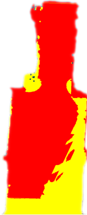
Figure 5.17: Box test camera positions 1 and 2 aligned using center point transformation then ICP, reference versus registered meshes
