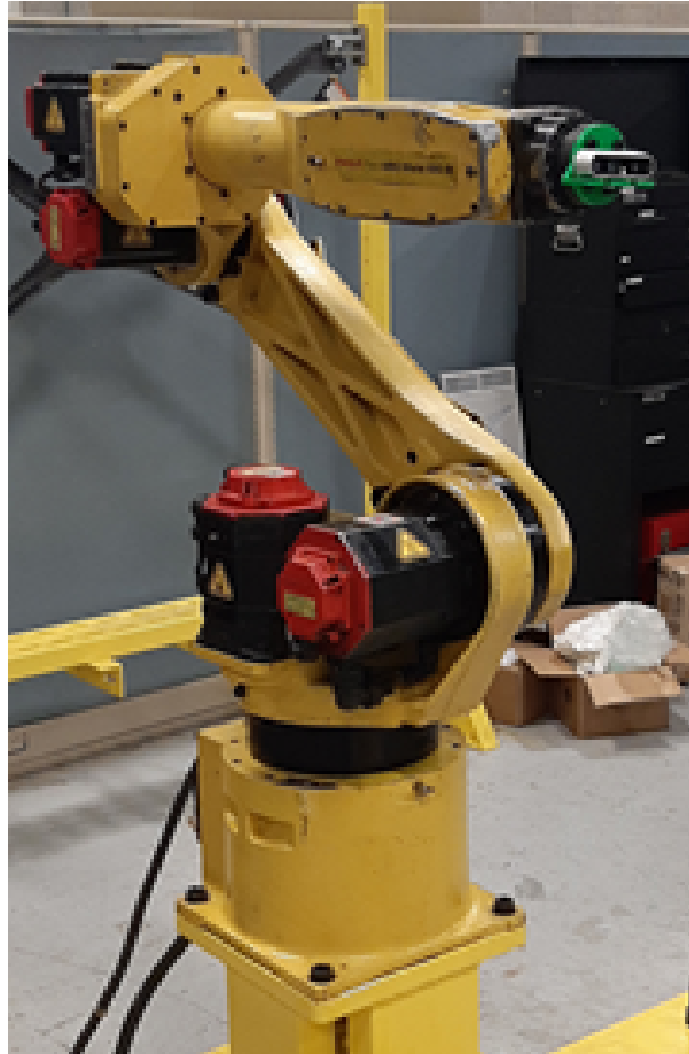
Figure 5.10: Camera as the end-effector of a Fanuc ARC Mate 100ib robot arm
