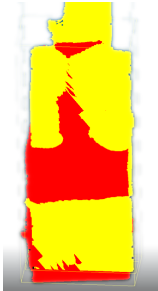
Figure 5.15: Box test camera positions 1 and 2 aligned using ICP, reference versus registered meshes
