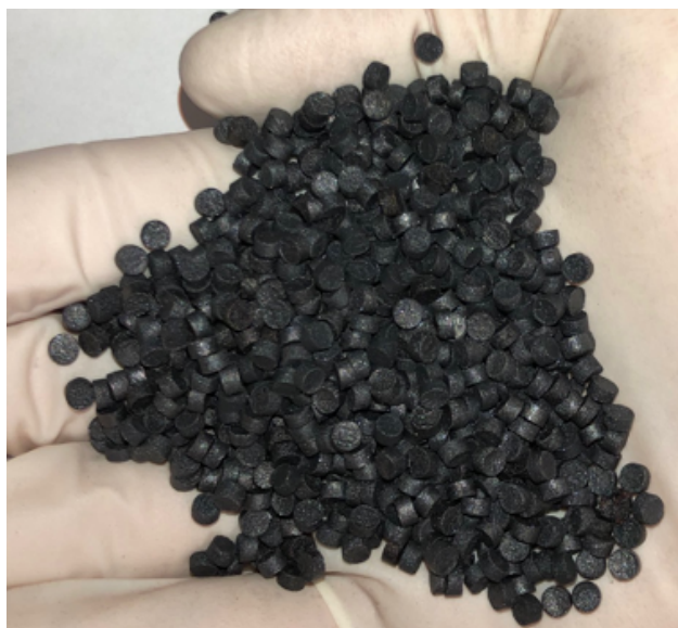
Figure 4.1: Magnesium-manganese-oxide pellets: These pellets are made by solid-state mixing of the magnesium- and manganese-oxide followed by a heat-treatment process. The mixed powder is added the mixed powder to an automatic pellet press.
