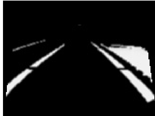
(d) This image shows the preprocessed camera input (B&W) for the real environment. The extracted features are similar between the simulated and physical world, though the real-world has more noise and the white floor is retained as a potential “line feature.”
