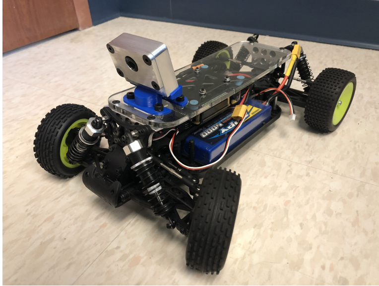
Figure 4.16: This 1/10th scale buggy features a Raspberry Pi 3B+, Navio2 interface board, Logitech F710 USB dongle, and a Raspberry Pi camera. Not pictured: LiDAR.
