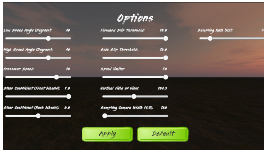
Figure 4.12: When the simulator is connected to a multi-display host, the second display allows users to adjust options in real-time. This greatly speeds up tuning the buggy model to match the physical model, and helps make the simulator more extensible to other vehicle types.
