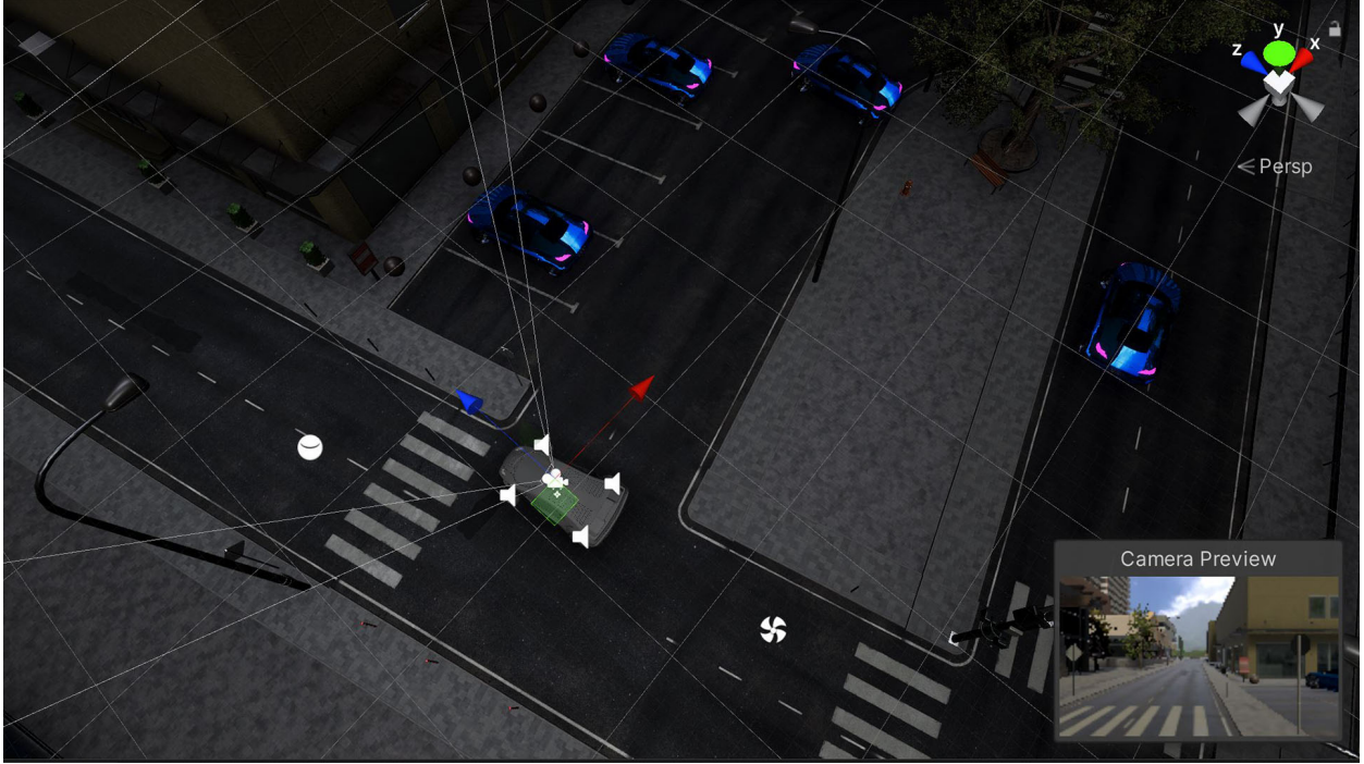
Figure 4.25: The application's Editor Mode. At center, we can identify the vehicle controller and the single LiDAR camera that performs the sampling in the virtual environment.
