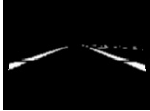
(b) This image shows the preprocessed camera input (B&W) for the simulated environment. The lines stand out relative to the rest of the image, improving classifier robustness.
