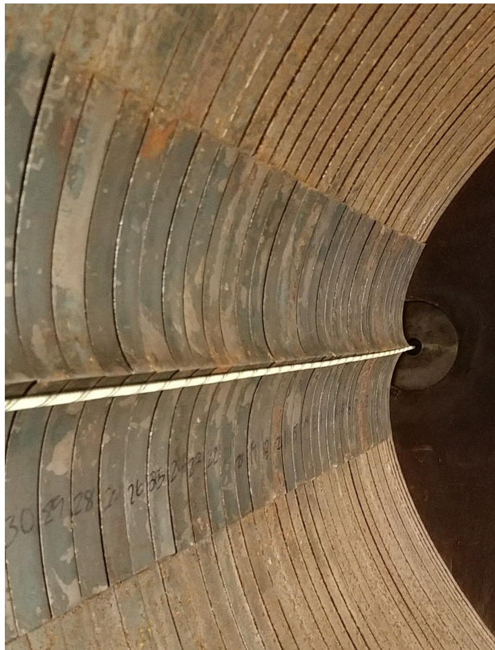
Figure 4.7. Example of how Det-cord is mounted along the focus point of the logarithmic spiral of the driver section. Adapted from [85]
