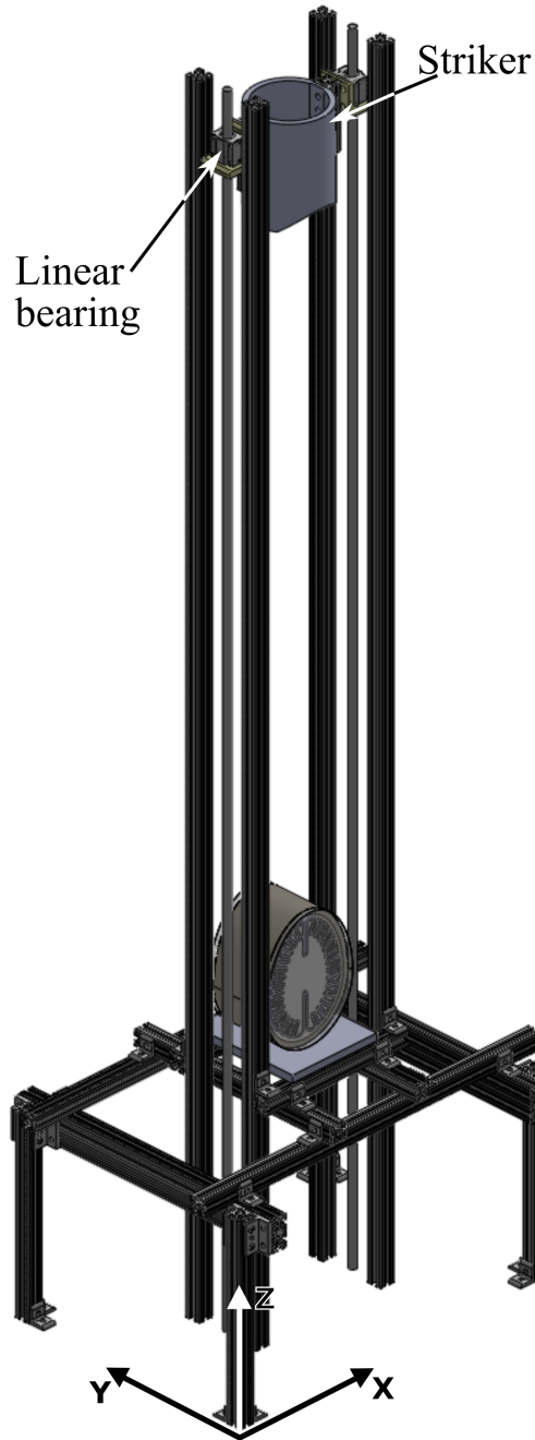
Figure 4.1. 3D CAD Representation of the Drop Tower with Impactor and Biofidelic Test Object. External dimensions: X- 61 cm (24 in), Y- 46 cm (18in), Z- 183 cm (6ft).
