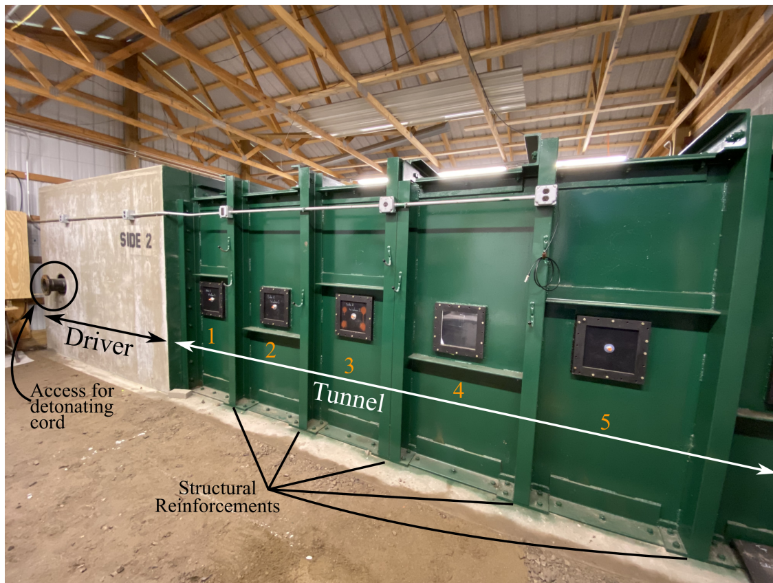
Figure 4.6. Isometric Side View of the ABC detailing Driver and Tunnel sections. Called-out Structural Reinforcements correspond to the vertical demarcated line in figure 4.5. Individual access windows are numerically labeled. Access point for the mounting and detonation of the explosive charges is identified (black circle, left side of figure). Adapted from [85]
