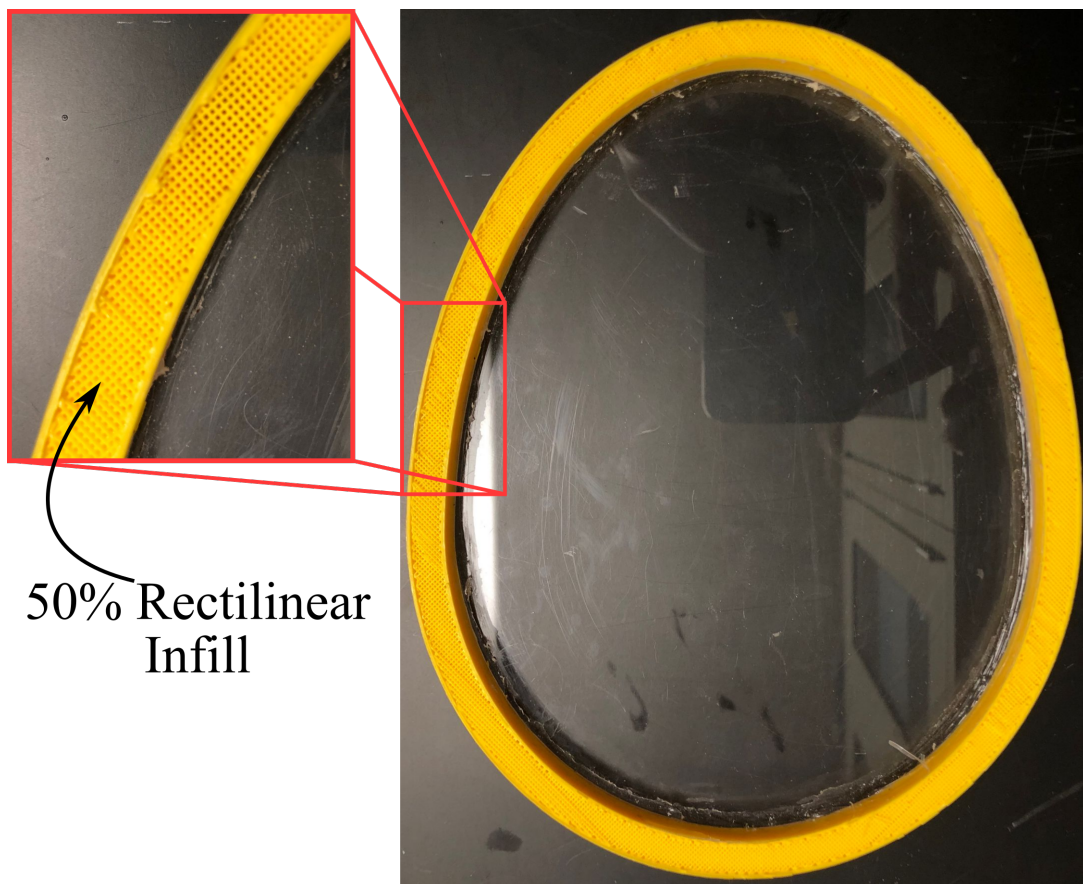
Figure 3.11. Example of the 50% rectilinear infill pattern present within the 3D printed skulls.
