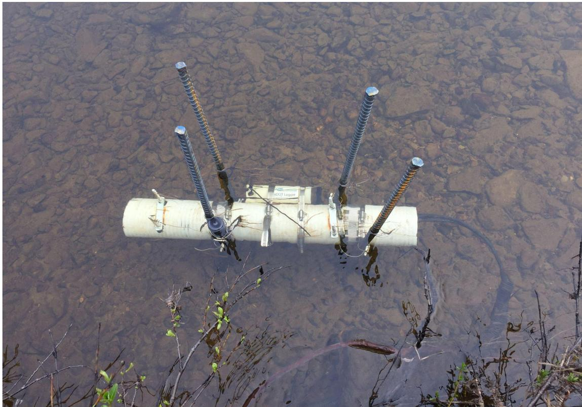
**Figure 3.2.2:** In-situ UV-visible spectrophotometer encased in a PVC housing and anchored into the stream bed. Pressure transducer also housed and attached to the PVC.
