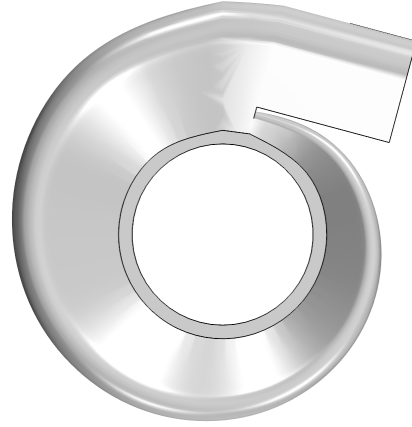
(b) 3D CAD model of the trapezoidal volute
