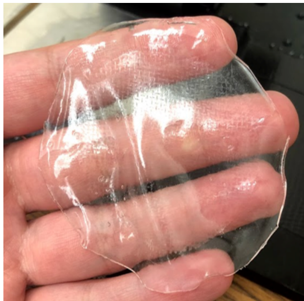
Figure 5.2: (a) Process of preparation of PVC gel membrane; (b) A photograph of a fabricated PVC gel membrane.
