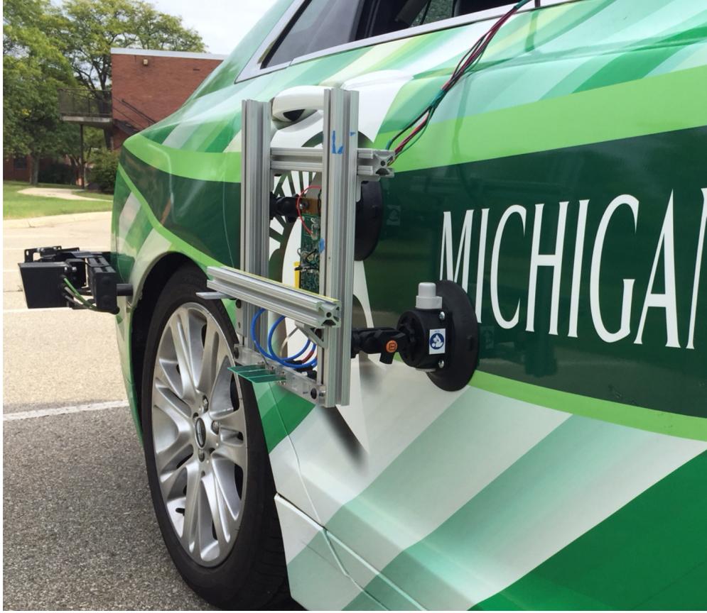
Figure 5.5: The 40 GHz radar hardware suction mounted to the MSU CANVAS autonomous vehicle test platform. Approximately 20 minutes of driving data was captured at MSU’s Spartan Village. Image [5] © 2020 IEEE.
