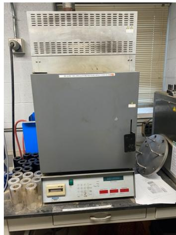
**Figure 17 NCAT ignition oven**
