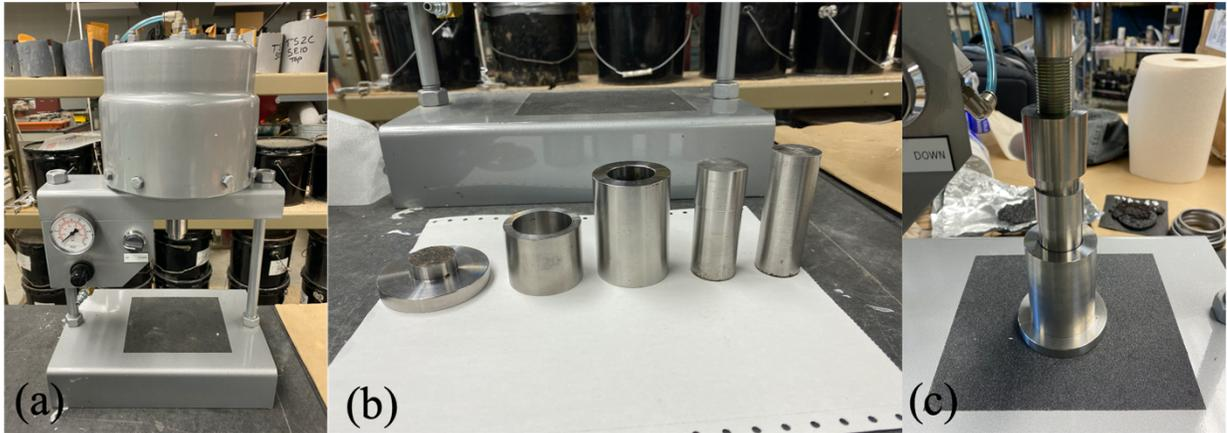
**Figure 33. (a) Pill compressor, (b) compaction molds and (c) pill preparation**
