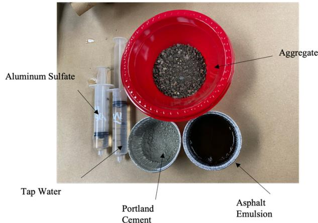
**Figure 1. Mix-Time Test Materials**
