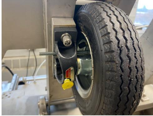
**Figure 49 Illustration of how the wheel was locked by a steel rod in HLW test**
