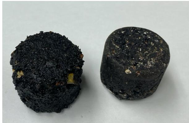
**Figure 56. Sample expansion after integrity test**
