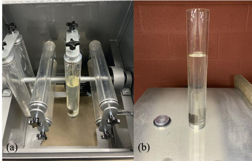
**Figure 35. Compatibility Test Abrasion Test Setup**
