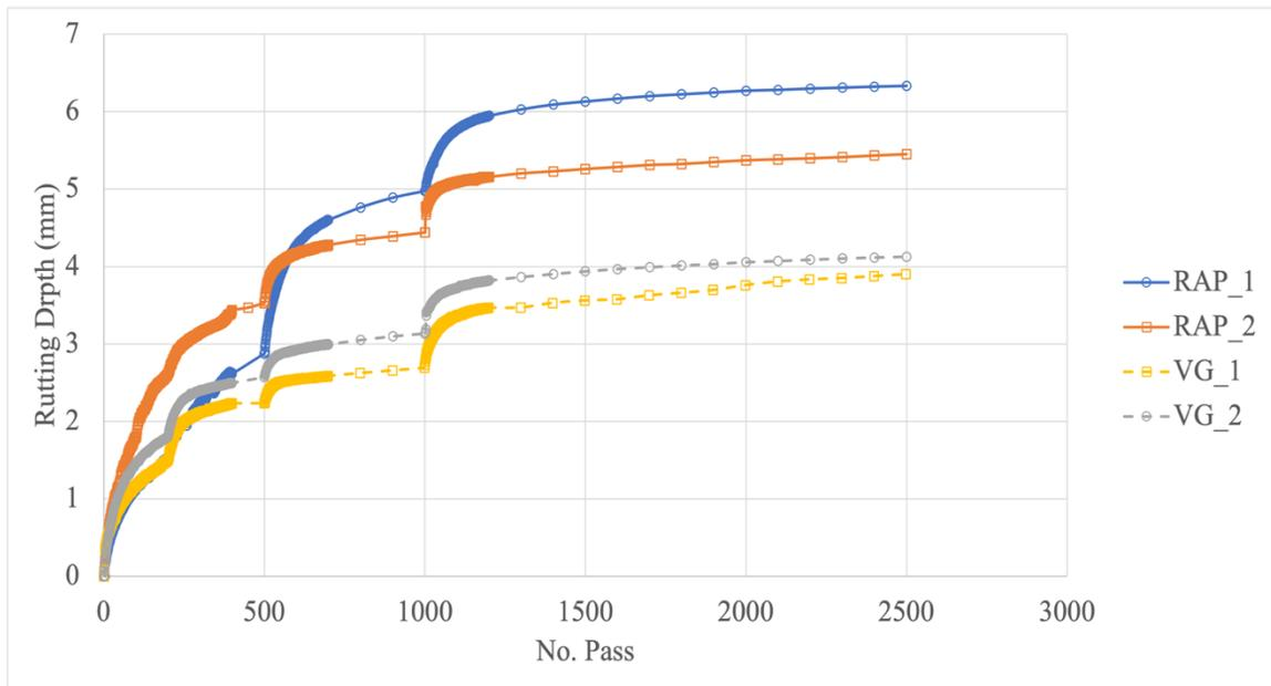
**Figure 61. HWT Rutting Plot Data at 54°C (wet)**
