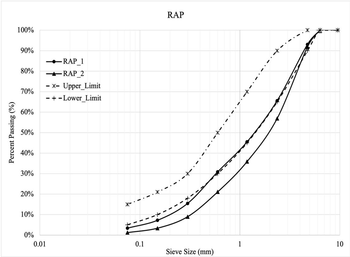
**Figure 18 Gradation of RAP aggregate (covered with binder – as it was received from the RAP stockpile)**
