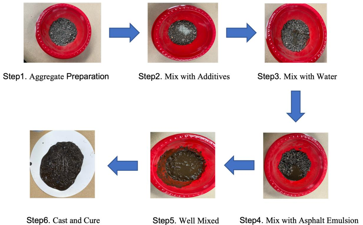
**Figure 22. Mix-time test procedures**
