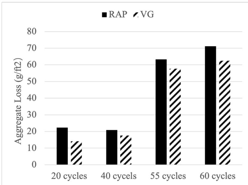
Figure 67 HLW test abrasion loss with application rate at 18 lb/yd<sup>2</sup>
