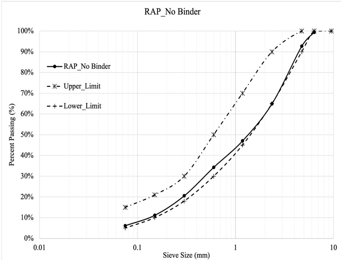
**Figure 19 Gradation of RAP aggregate without binder (after burning out the binder from the surface of the RAP aggregates)**
