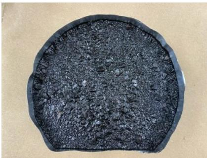
**Figure 44. Asphalt substrate with cured slurry seal layer**
