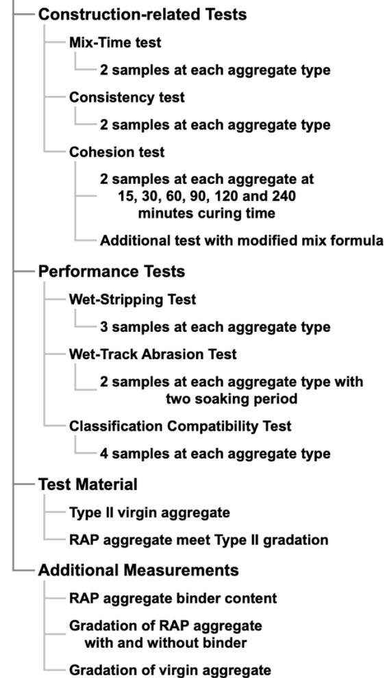
Figure 14 Test plan for the traditional ISSA tests
