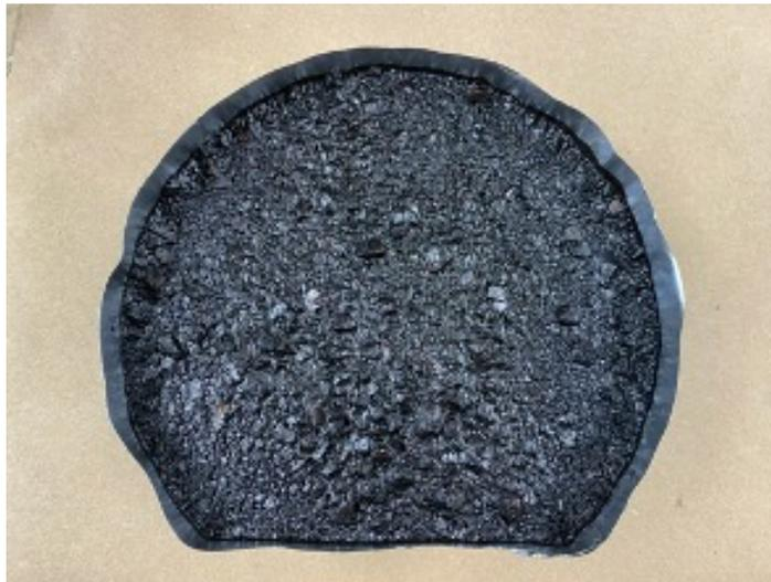
**Figure 41. Prepared HWT specimen**
