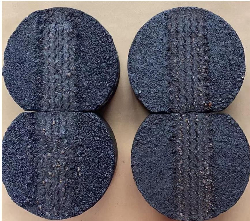
**Figure 59. Samples tested in the wet condition: RAP(*left*) and VG(*right*) Comparison**
