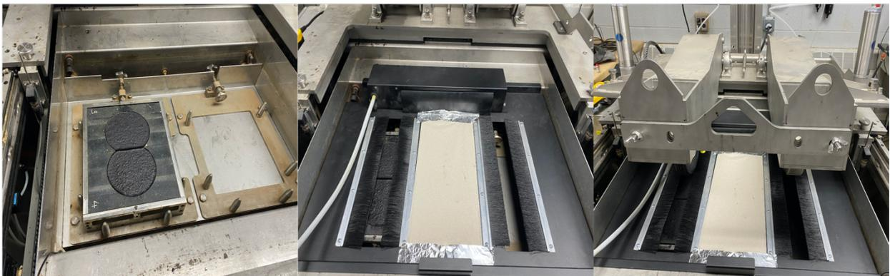
**Figure 46. Hamburg wheel tracking tester (dry set up)**
