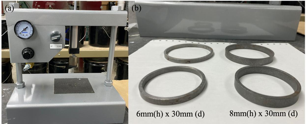
**Figure 25. (a) Cohesion tester and (b) mold rings**
