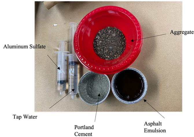
**Figure 21. Components of the slurry seal mix time (ISSA TB 113) test**
