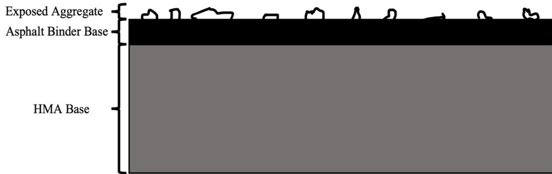
**Figure 68 Conceptual drawing of exposed aggregates and asphalt binder base**
