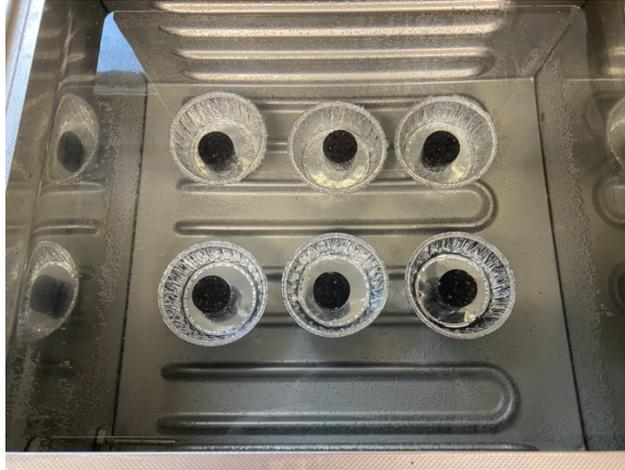
**Figure 34. Compatibility Test 6-Day Soaking**
