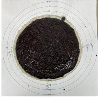
**Figure 3. Consistency Test Sample Result**
