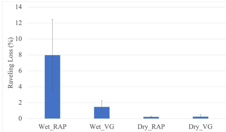
**Figure 60. HRW raveling loss values for both RAP and VG mixtures tested in dry and wet conditions.**
