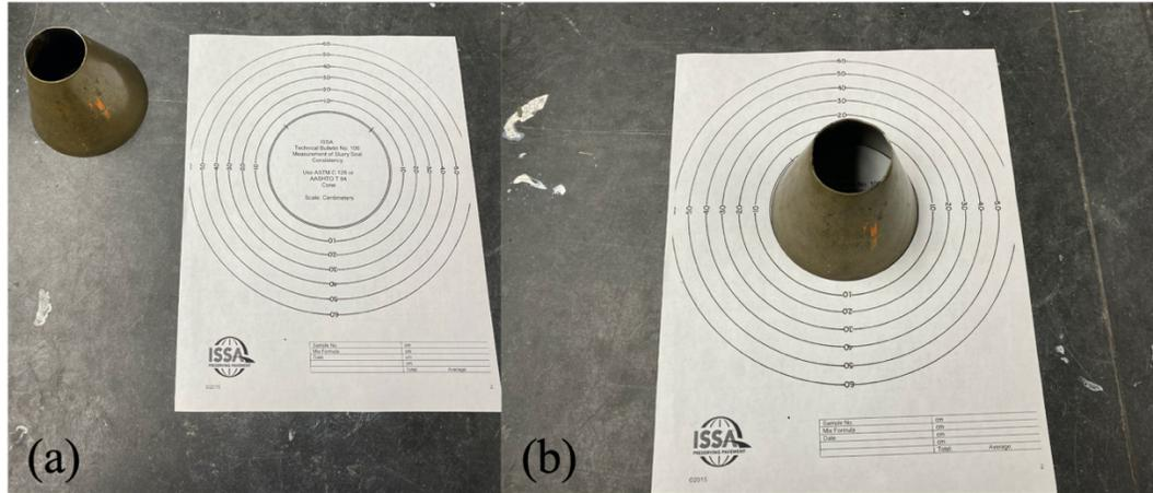
**Figure 23. Consistency test set-up**
