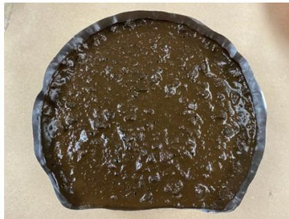
**Figure 43. Asphalt substrate with wet slurry seal layer**
