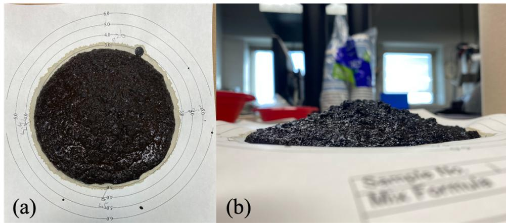
**Figure 24. (a) Illustration of spreading of the slurry seal sample and (b) side-view of the slurry seal ‘clump’**
