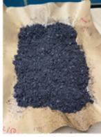
Step1: Prepare desired amount of HMA loose mixture
