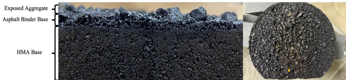
**Figure 69. Actual picture of slurry seal with RAP illustrating the exposed aggregates.**
