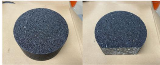
Step5: Cut the base to match the Hamburg wheel tracking tester mold
