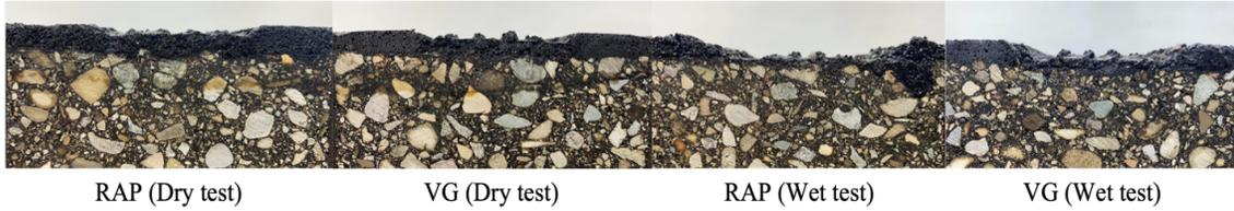
**Figure 63. Cross sectional views of the slurry seal samples after the HRW tests**
