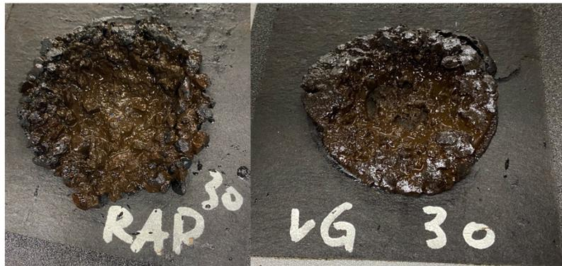
**Figure 51. The modes of rupture for RAP and VG aggregates tested at 30 minutes**
