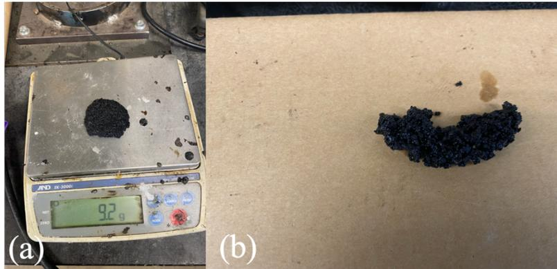
**Figure 54. Wet-stripping test sample (a) before and (b) after the test**
