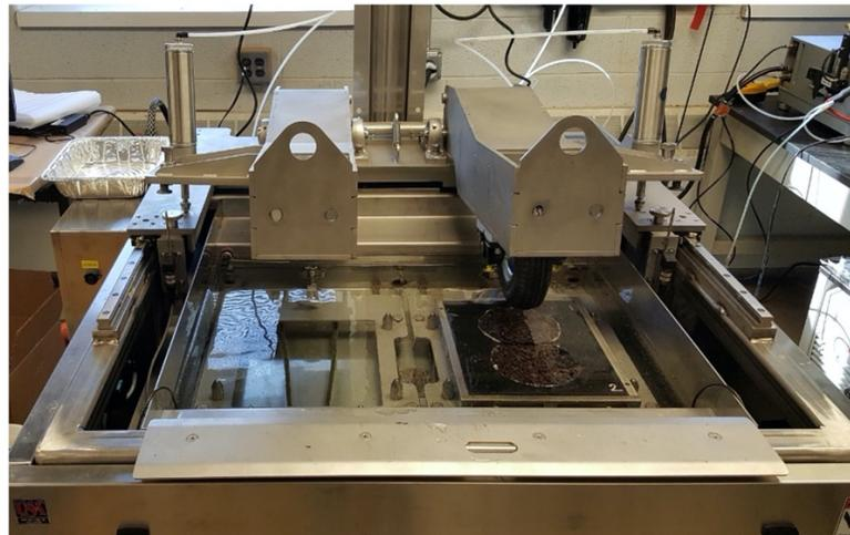
**Figure 45. Hamburg wheel tracking tester set up with water bath**
