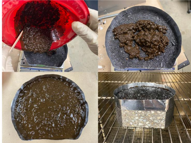
**Figure 40. Illustration of casting of the slurry seal sample and oven-drying**
