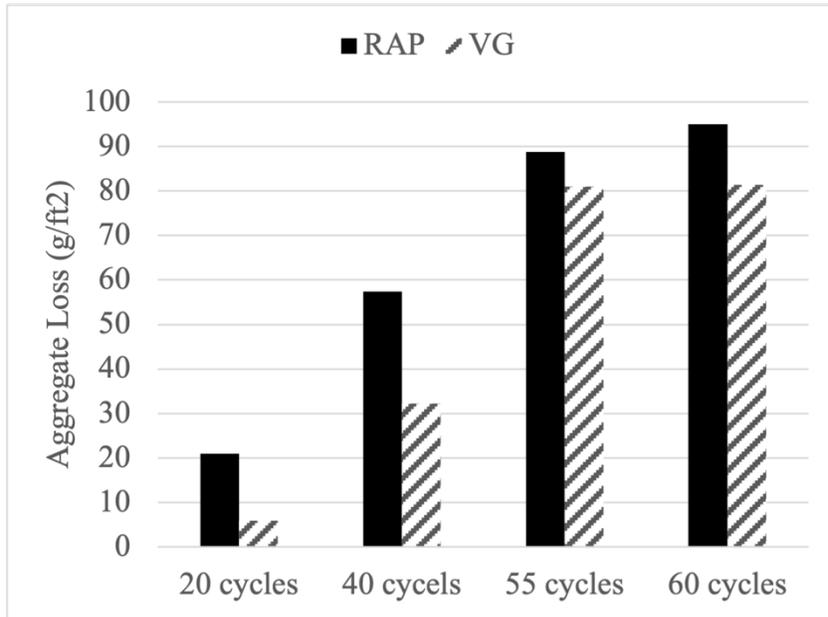
Figure 66 HLW test abrasion loss with application rate at 10 lb/yd<sup>2</sup>
