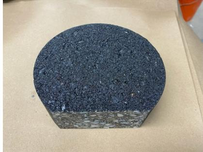
**Figure 42. Compacted asphalt mixture substrate used in the Hamburg tests**
