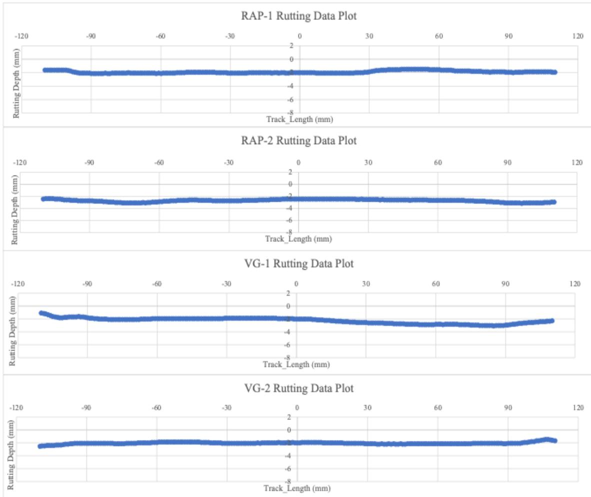
**Figure 65. Longitudinal rutting profiles of the samples tested in wet condition.**
