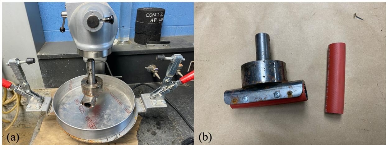
**Figure 30. (a) WTAT device N-50 Hobart model and (b) rubber hose used to abrade the surface**
