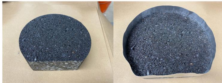
**Figure 39. Illustration of the wrapping of the circumference of the sample with an aluminum tape.**
