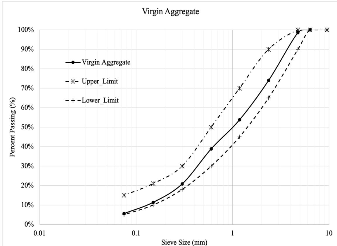
**Figure 20 Gradation of Virgin aggregate without binder**
