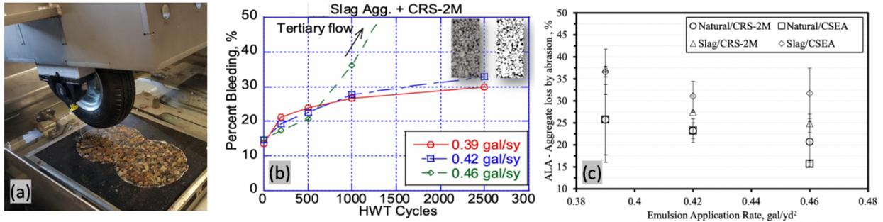
Figure 13. (a) A picture of the modified HWT device for chip seal abrasion and bleeding testing, (b) an example bleeding data and (c) abrasion (aggregate loss) data.
