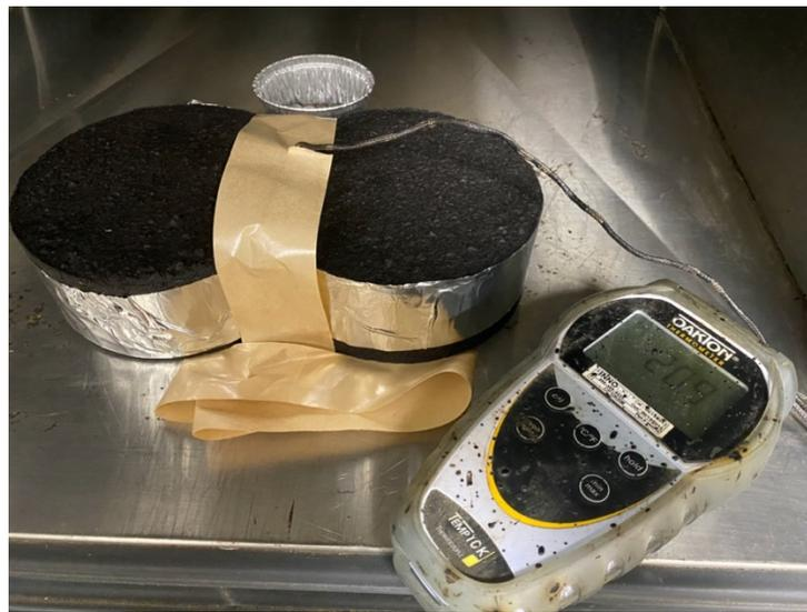
**Figure 47. HWT test sample pre-conditioning in the environmental chamber**
