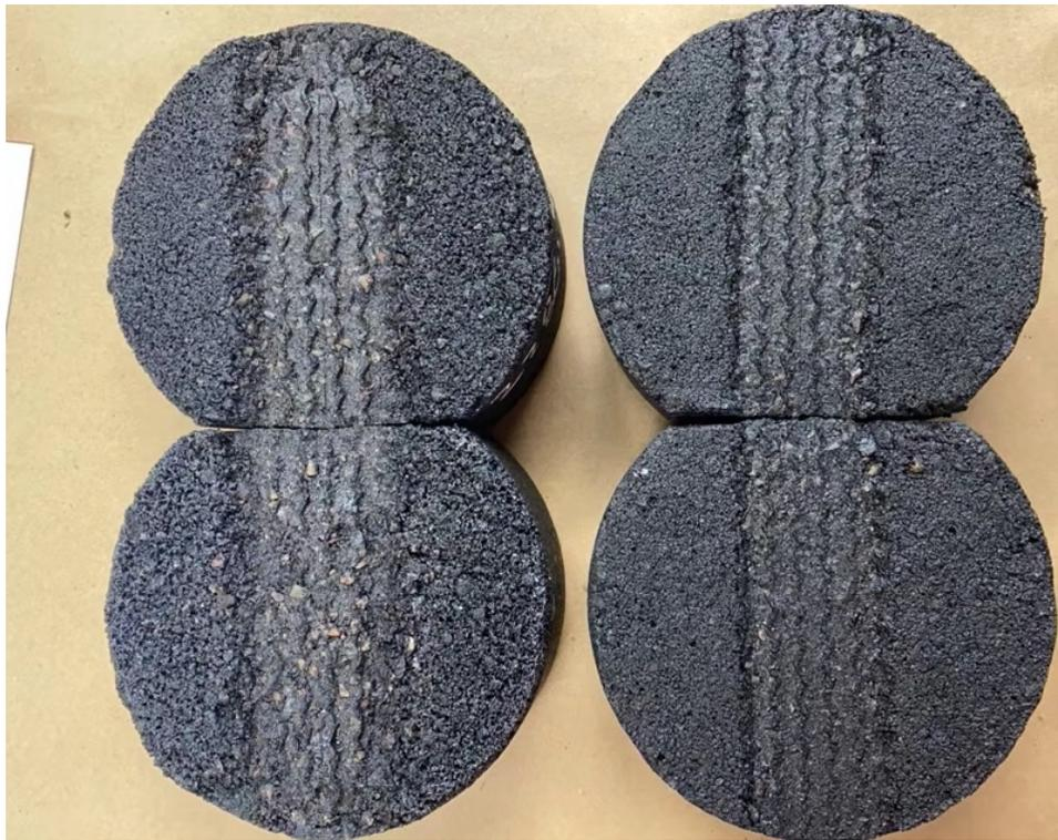
**Figure 57. HWT RAP Mixture Wet (*left*) and Dry (*right*) Comparison**
