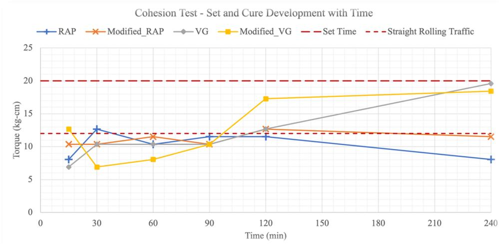
**Figure 50. Cohesion test results from this study**
