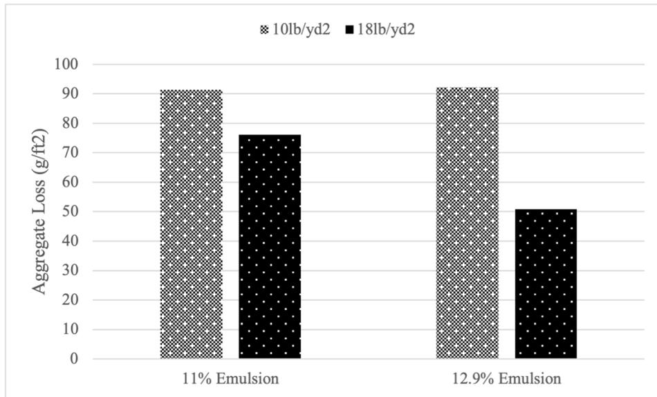
**Figure 70 Modified HLW test abrasion data using 100% RAP aggregates**
