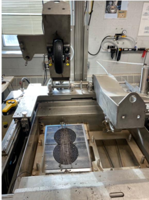
**Figure 48. HLW test setup with slurry seal (after the abrasion test)**
