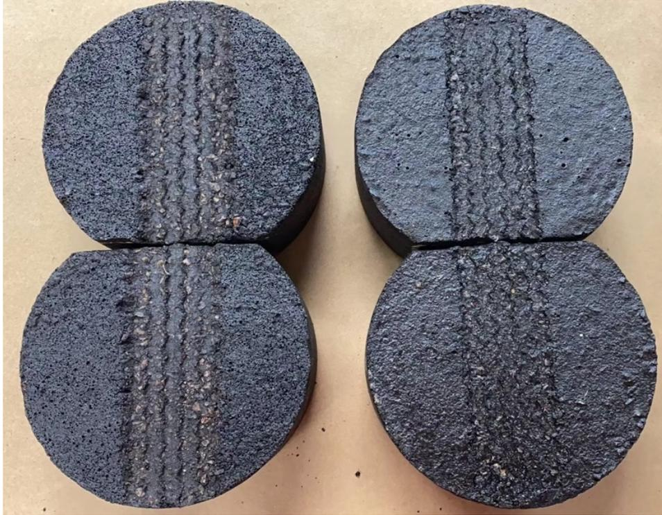
**Figure 58. HWT VG Mixture Wet (*left*) and Dry (*right*) Comparison**
