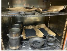
Step2: Place material and compaction molds in oven at compaction temperature
