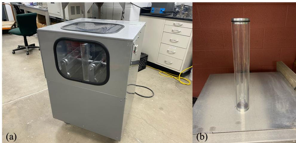
**Figure 32. Schulze-Breuer device(a) and test tube(b)**
