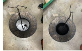
Step2: Place HMA material in compaction molds
