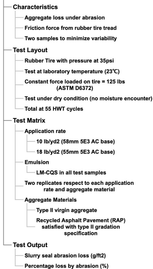
Figure 16. Hamburg locked wheel (HLW) test plan
