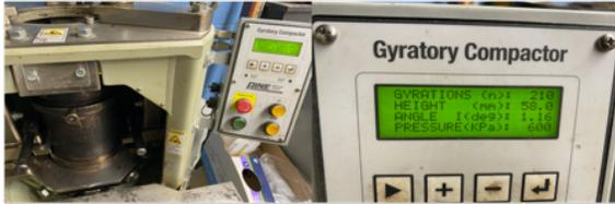
Step3: Compact the HMA mixture in desired height
