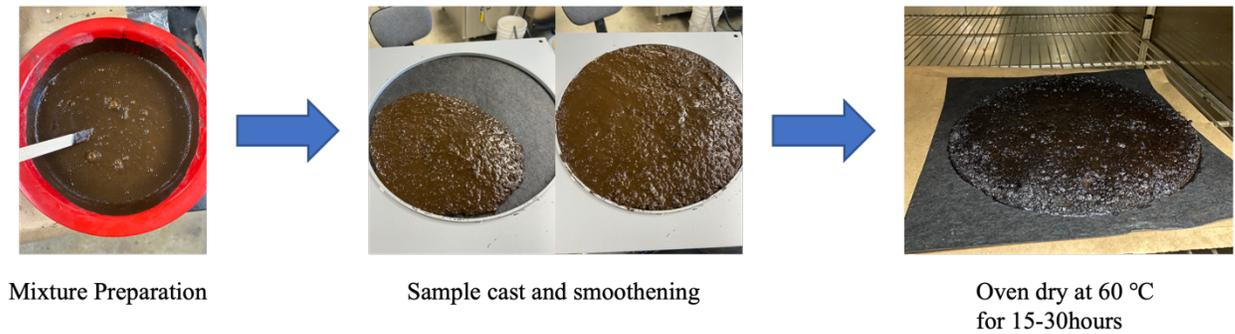
**Figure 29. Sample preparation steps for the WTAT**
