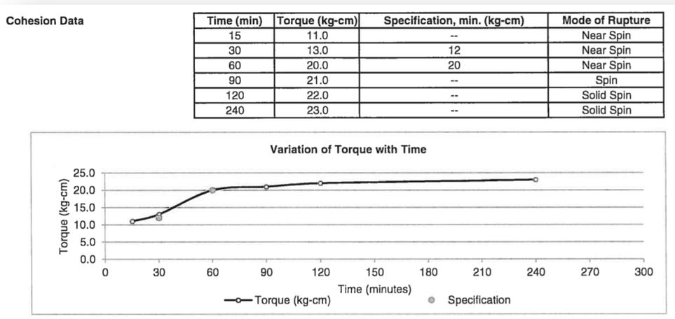
**Figure 52. Cohesion data from the Wood**
