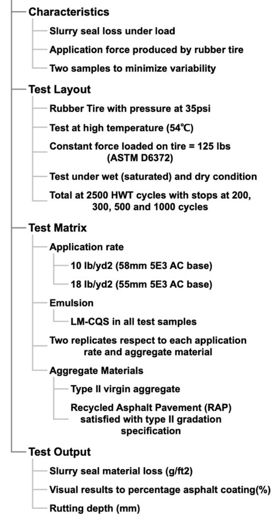
Figure 15. Hamburg rolling wheel (HRW) test plan
