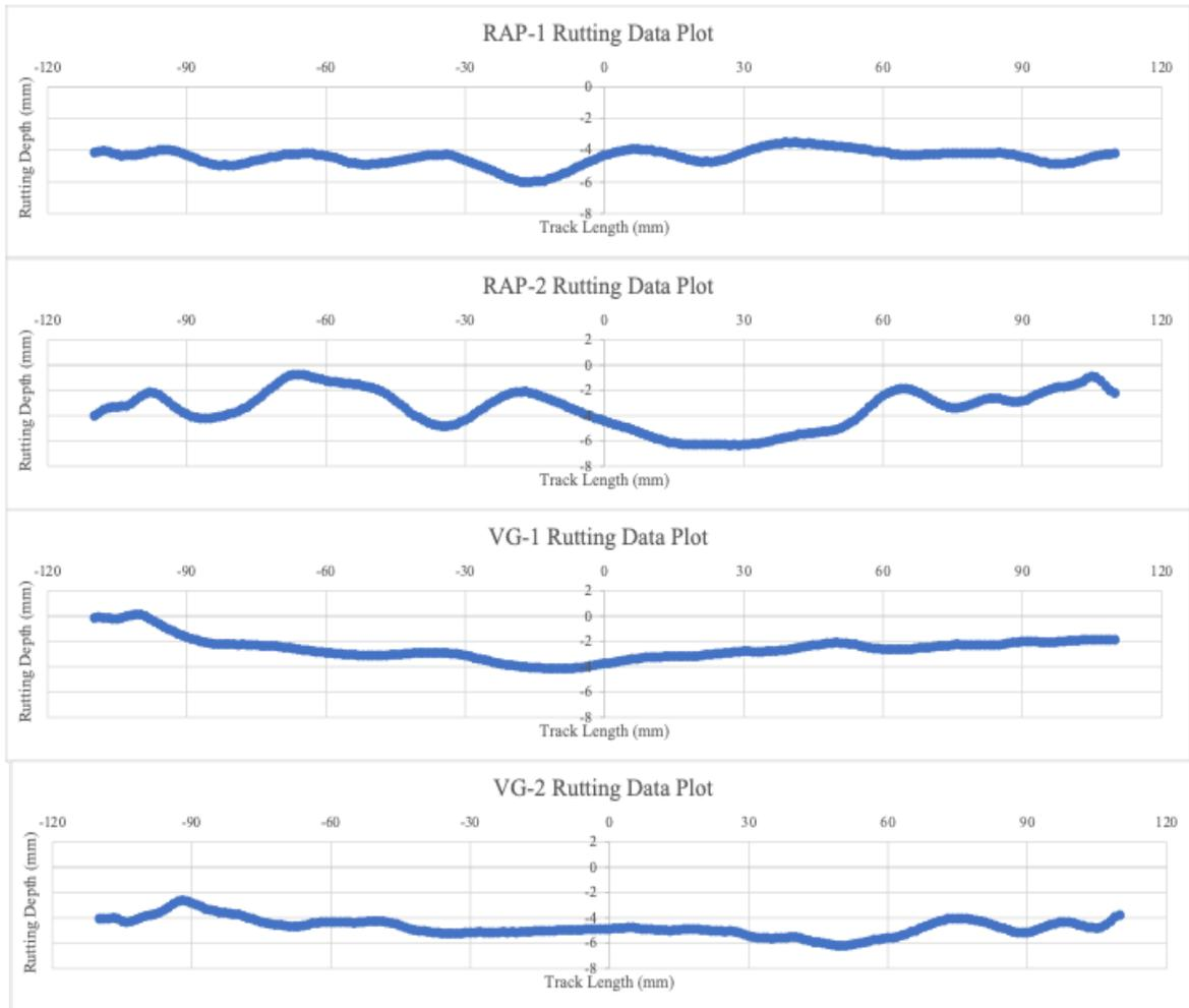
**Figure 64. Longitudinal rutting profiles of the samples tested in wet condition.**
