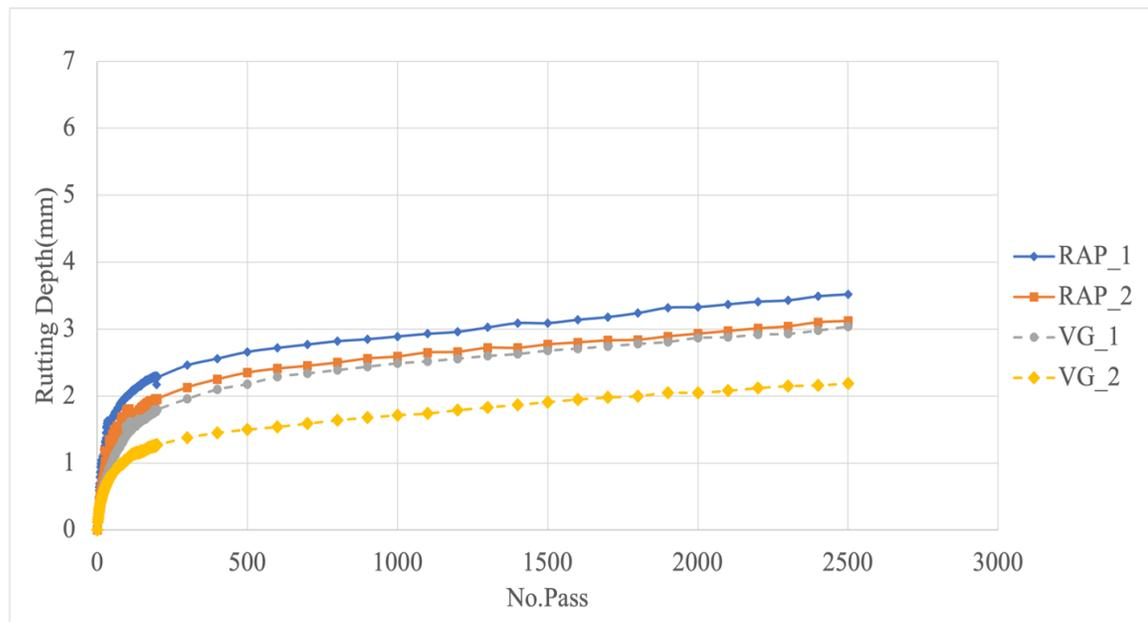
**Figure 62. HWT Rutting Plot Data at 54°C (dry)**
