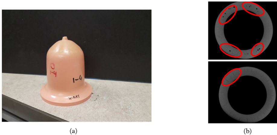
Figure 9.6: Scanning of reference plastic cap, a) Picture of the tested sample, b) Two Micro CT sliced with marked defects.
