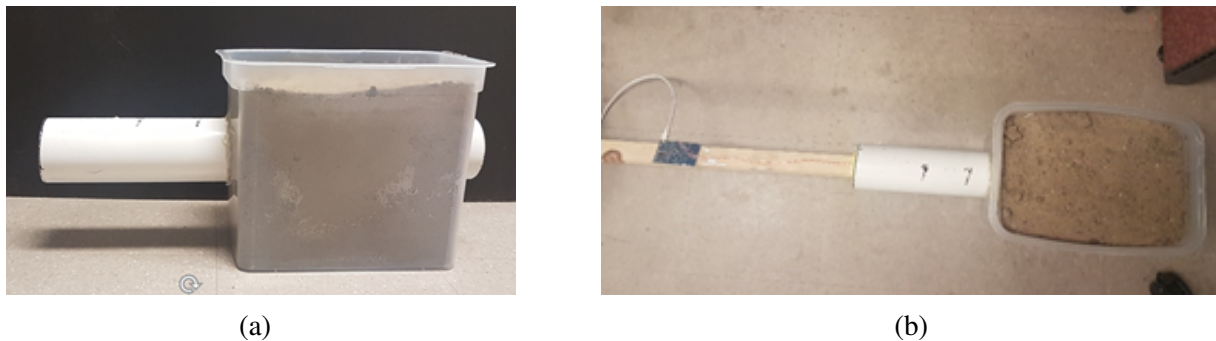
Figure 10.4: a) Preliminary test setup (side view), b) EM sensor inside the preliminary test setup (Top view).
