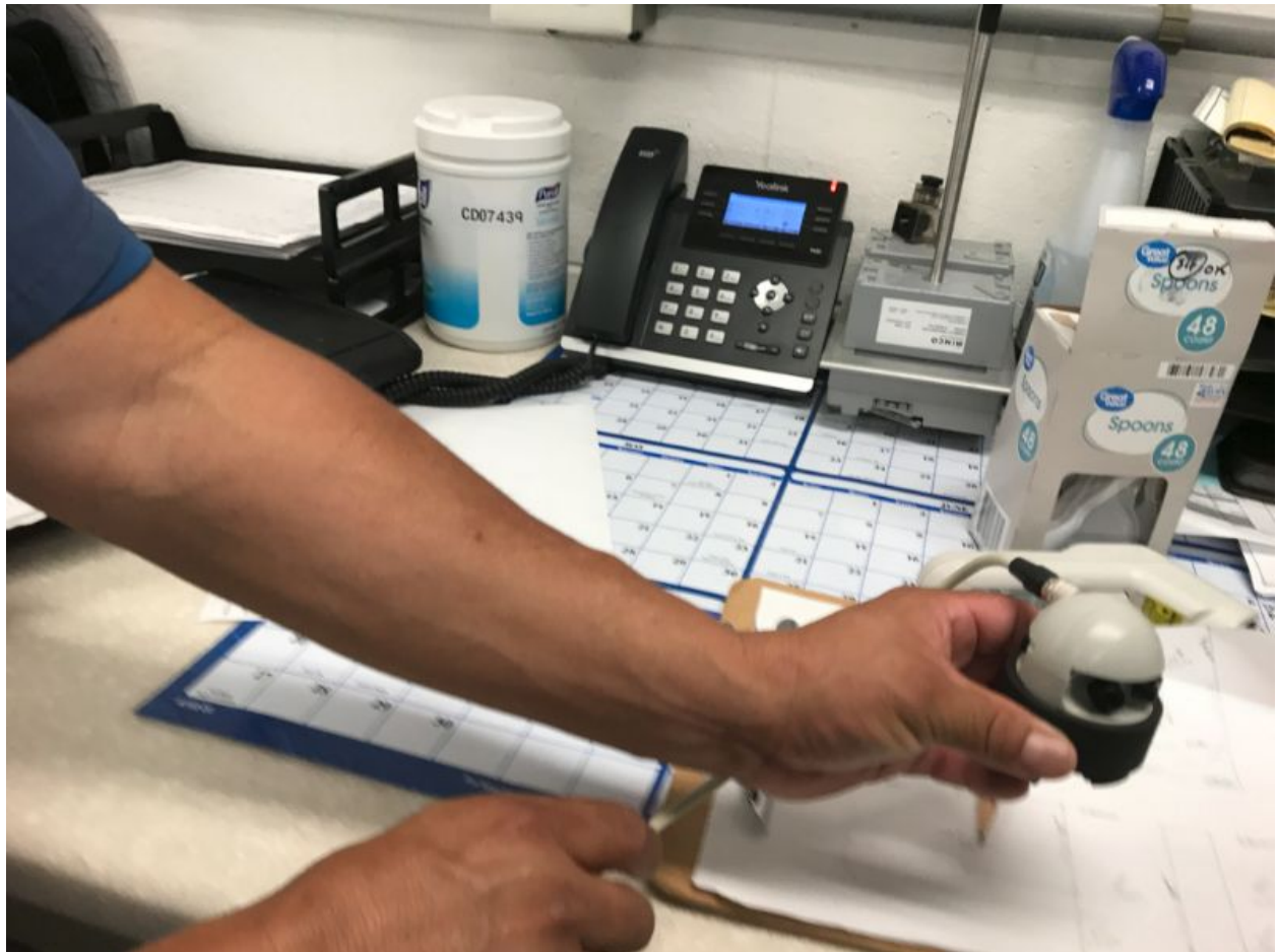
Figure F.23: Egg monitor that goes in the incubation machine to give temperature and humidity readout in a specific section of the incubation machine.
