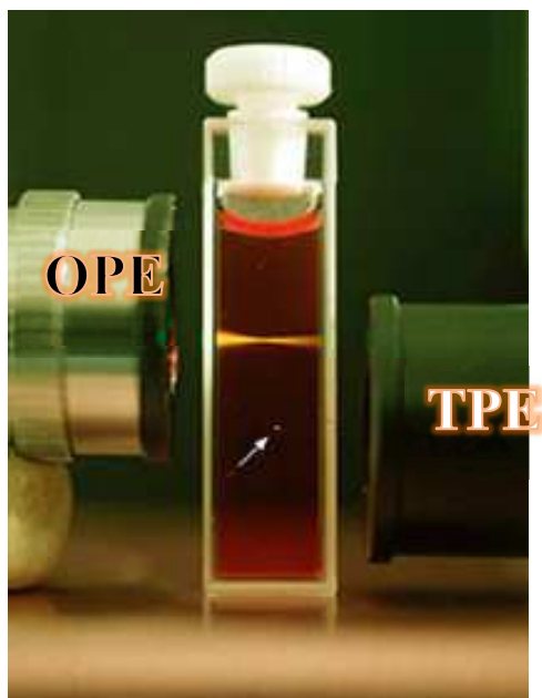
Figure 1.2. Simultaneous OPE and TPE of sample solution in cuvette. The objective on the right for TPE is producing fluorescence only at the focal point (shown with the white arrow). Photographed by Amos W.B. and Cipollone M, MRC Cambridge.
