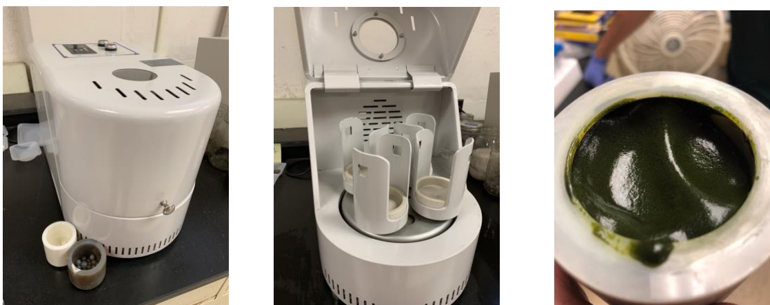
Figure 7. Left & middle: Lab scale planetary ball mill used for the optimization of milling for microalgal biomass. Zirconia (white) and agate (grey) milling vessels are pictured next to the ball mill. Right: Microalgal slurry after cell disruption in the planetary ball mill using agate milling media.
