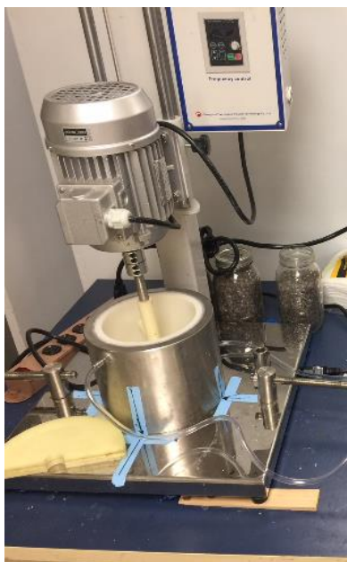
Figure 8. Stirred 2 L ball mill for cell disruption and protein recovery.
