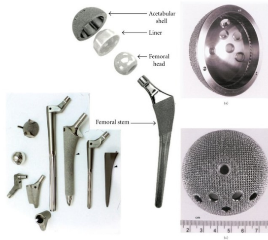
Figure 2.1 Acetabular cup produced by electron beam melting process in a single build [24].
