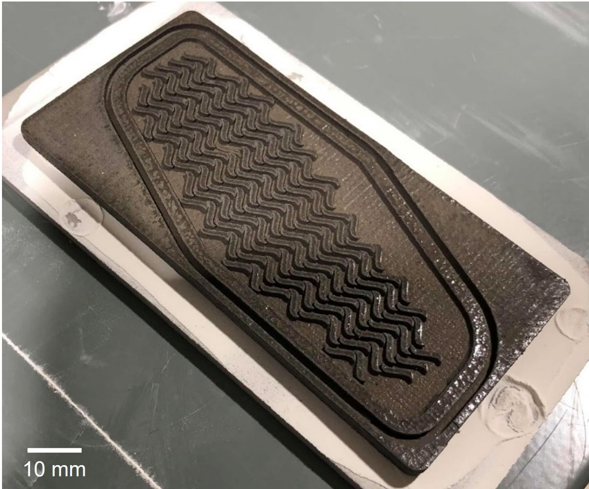
Figure 4.11 Amdry 386 full size heat exchanger fabricated by SEAM process.
