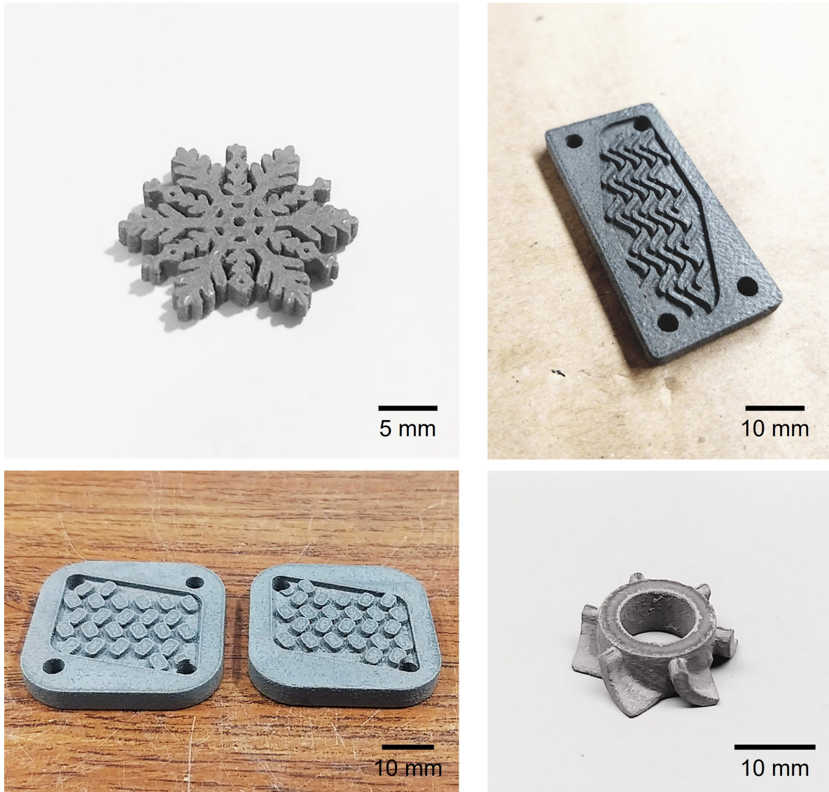
Figure 3.19 Demonstration parts fabricated using SEAM Process first-generation prototype. Top-left: Haynes 214 snowflake; Top-right: SS420 Mini heat exchanger; Bottom-left: Haynes 214 mini heat exchangers; Bottom-right: SS316L turbine.
