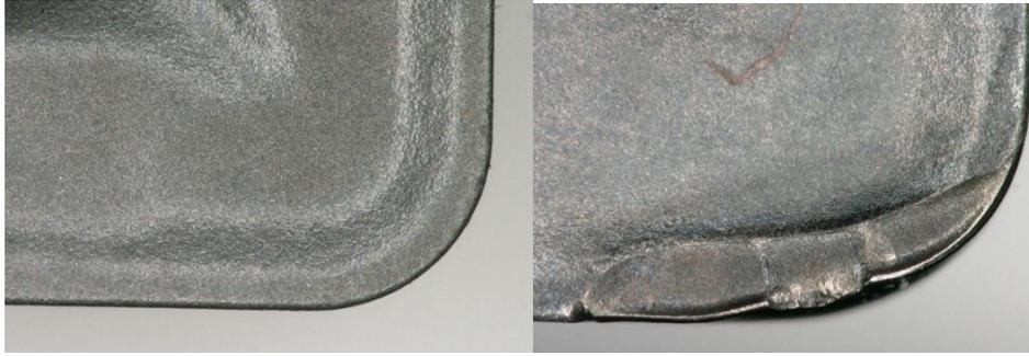
Figure 65. Rake face of the fresh and worn tool after machining with MoS<sub>2</sub> lubrication
